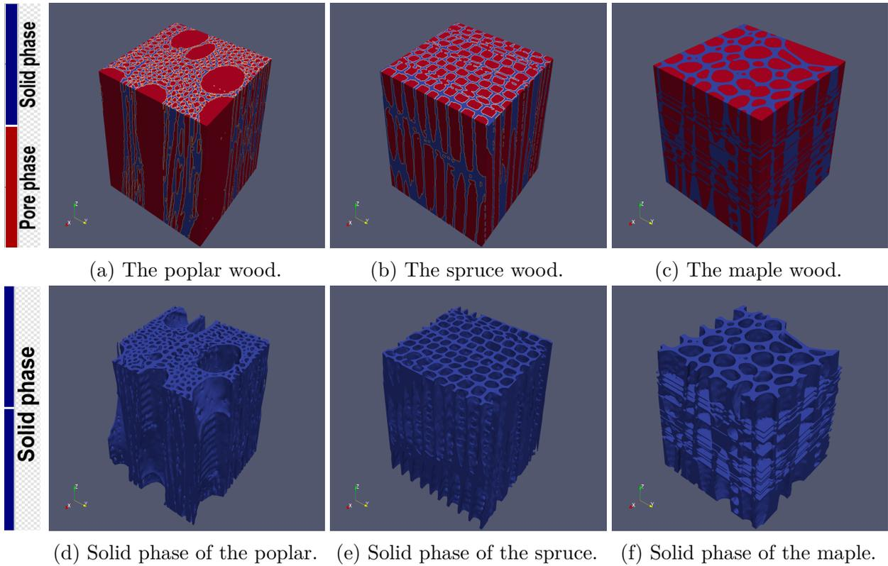
Figure 2: The extracted solid phase from the 3D reconstructed wood specimens scanned by X-ray nano-tomography presented in Fig. 1 to model the material microstructure. Each specimen having the same dimension  $128 \times 128 \times 128$  voxels is treated with ImageJ-Python software.
