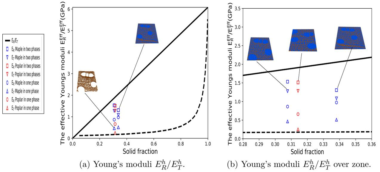
Figure 14: Upscaling strategy, such as the homogenization approach, is used to obtain the effective material properties of wood species over all phases compared with the homogeneous model at the macroscale.
