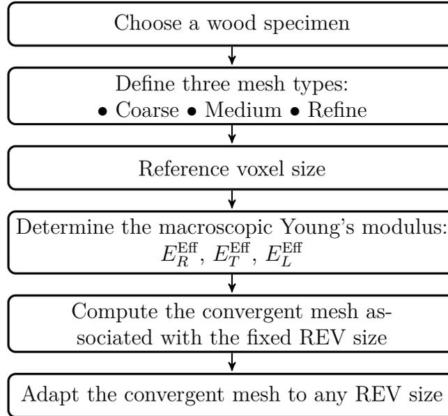
Figure 7: Flow chart to ensure the convergence and set-up scheduling the REV size.
