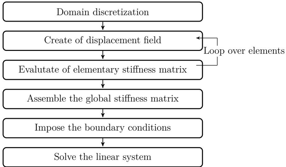
Figure 4: The computation process based on the homogenization scheme employing a FE discretization with displacement.
