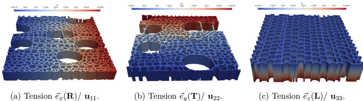
Figure 5: A series of mechanical tests demonstrating the validation of the orthotropic linear-elastic model for the poplar (left), maple (middle), and spruce (right) wood specimens. Each nodal displacement is generated for the uniaxial tensile test.
