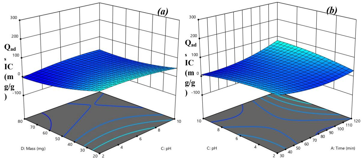
**Fig. S3.** Response surface plots of the central composite design showing the effect of time (min), pH and mass (mg) on the adsorption of the indigo carmine (mg/g)
