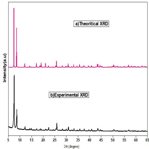
**Fig. S8.** Experimental and theoretical XRD pattern of NH<sub>2</sub>-UiO-66
