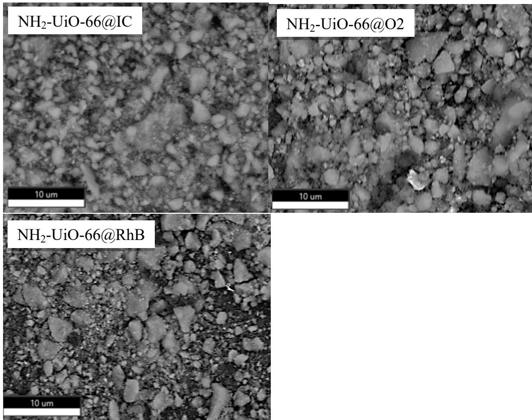
**Fig. S7.** SEM images of NH<sub>2</sub>-UiO-66 after indigo carmine (IC) (a), rhodamine B (RhB) (b) and orange 2 (O2) (c) adsorption
