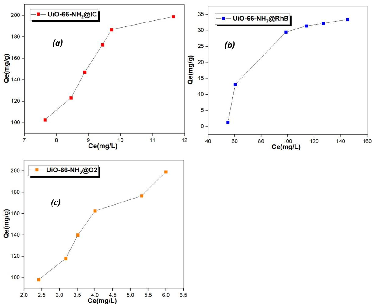
**Fig. S6.** Impact of concentration on the adsorption of indigo carmine (a), rhodamine B (b) and orange 2 (c) using  $\text{NH}_2\text{-UiO-66}$
