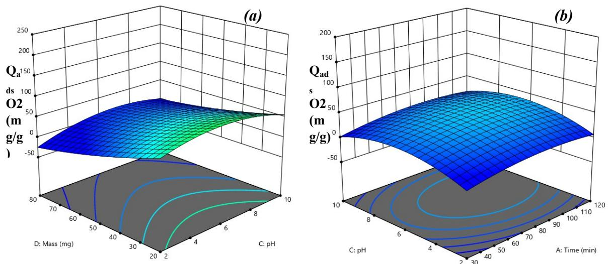
**Fig. S5.** Response surface plots of the central composite design showing the effect of time (min), pH and mass (mg) on the adsorption of the orange 2 (mg/g).
