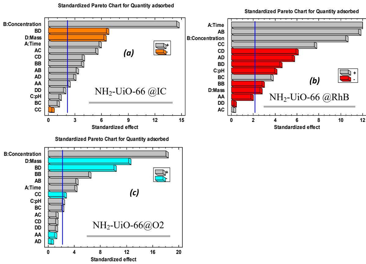
**Fig. S1.** Pareto diagrams of the effects of factors A, B, C and D for organic dyes IC (a), RhB (b) and O<sub>2</sub> (c) adsorption
