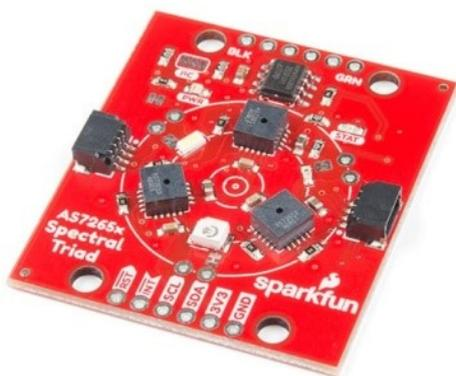
Figure S4. Triad Spectroscopy Sensor – AS7265x.
