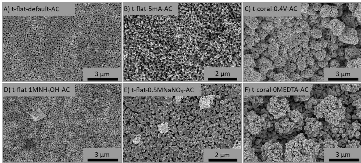
Figure S 14: SEM images of porous Ag catalysts after 1 cycle of catalysis prepared via Ag electrodeposition with slightly altered synthesis conditions: a) reference (-0.1 V vs Ag/AgCl, 0.05 M AgNO<sub>3</sub>, 1 M NaNO<sub>3</sub>, 0.01 M EDTA, 0.5 M NH<sub>4</sub>OH); b)-5mA; c) -0.4V; d) 1M NH<sub>4</sub>OH; e) 0.5M
