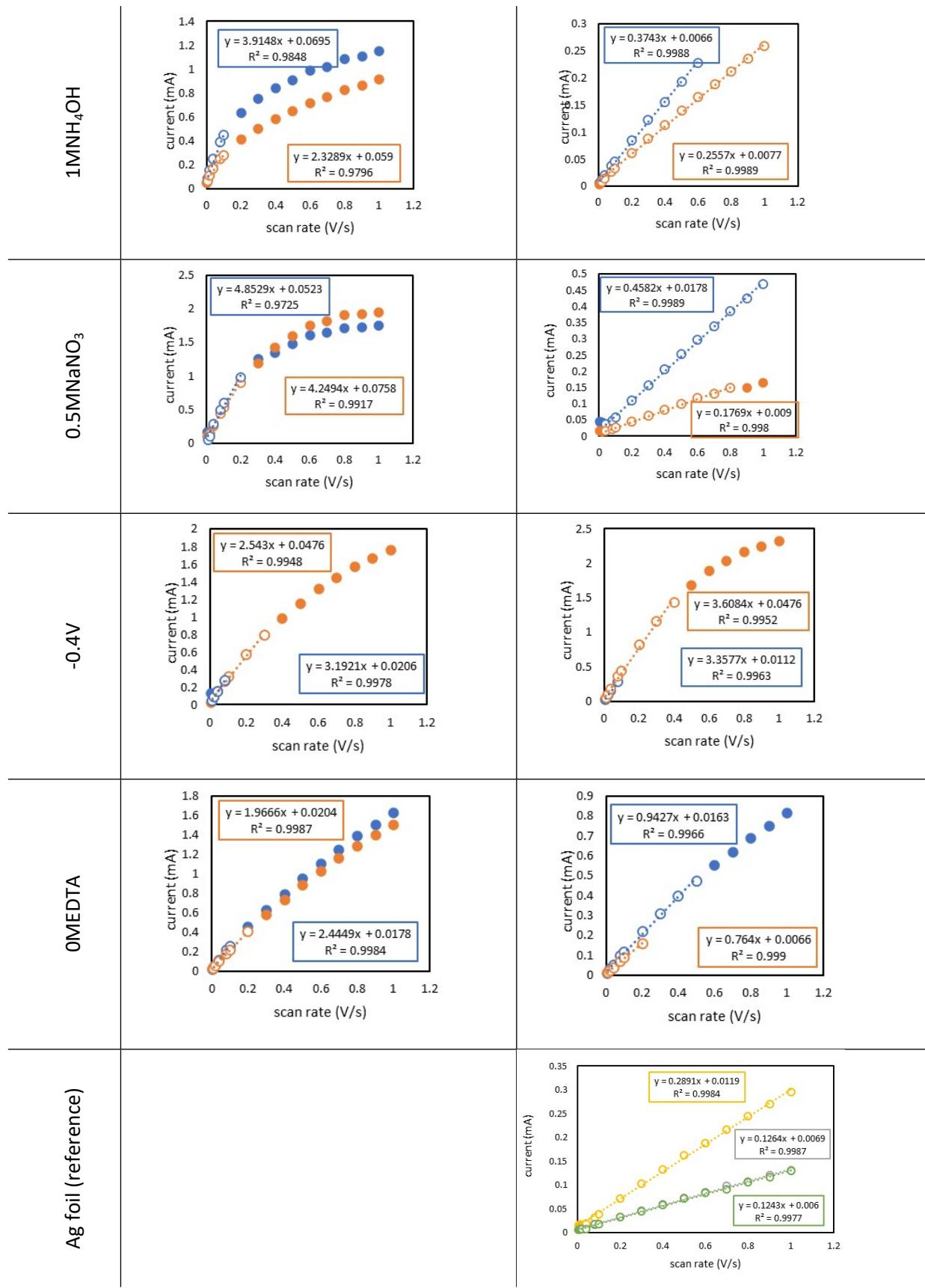
Figure S 7: Figure S 3:DLC graphs of all (non)-templated electrodes. The open dots indicate the data included to fit the double-layer capacitance.
