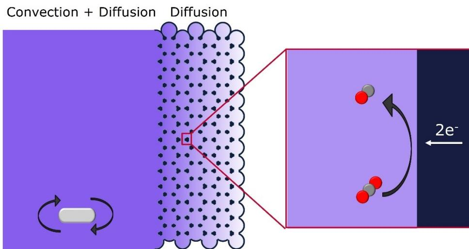
Figure S 2: Schematic representation of convection and diffusion inside the electrochemical cell and the porous electrode including the  $\text{CO}_2$  reduction reaction that is taking place.
