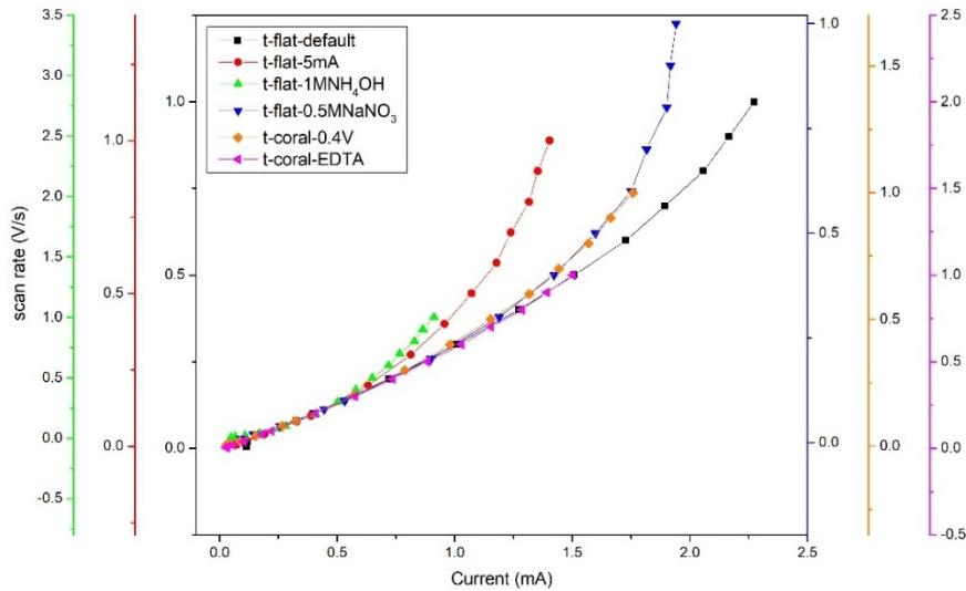
Figure S 8: plots of the scan rate vs the current determined with DLC for the six templated samples showing the different limiting currents
