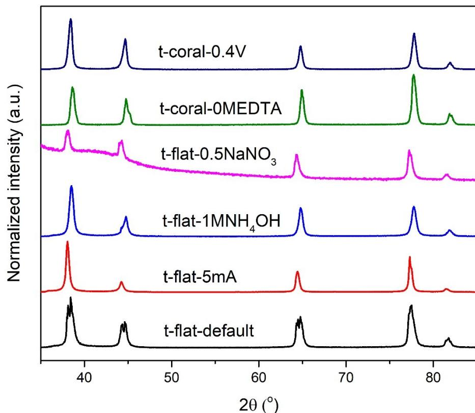
Figure S 5: X-ray diffraction patterns of the t-flat-default, t-flat-5mA, t-flat-1M NH<sub>4</sub>OH, t-flat-0.5M NaNO<sub>3</sub>, t-coral-0MEDTA and t-coral-0.4V electrodes.
