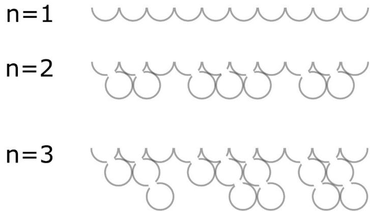
Figure S 9: Illustration of accessible pores for 1 to 3 layers. The grey line is the surface area that is included in the calculation.
