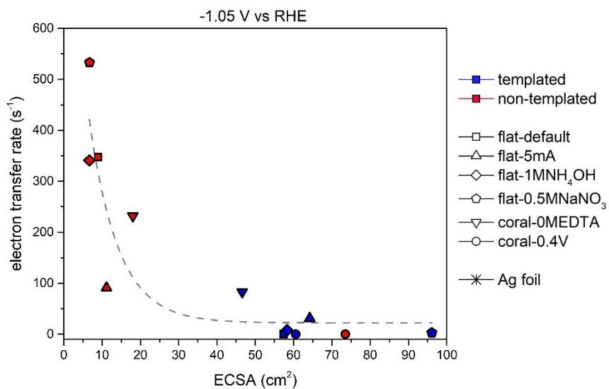
Figure S 13: Electron transfer rate for both the template-based porous (blue) and non-templated equivalent (red) samples nt-flat-default, (n)t-flat-5mA, (n)t-flat-1MNH<sub>4</sub>OH, (n)t-flat-0.5MNaNO<sub>3</sub> and (n)t-coral-0MEDTA at -1.05 V vs RHE plotted versus the ECSA. A dashed gray line is provided as a guide for the eye.
