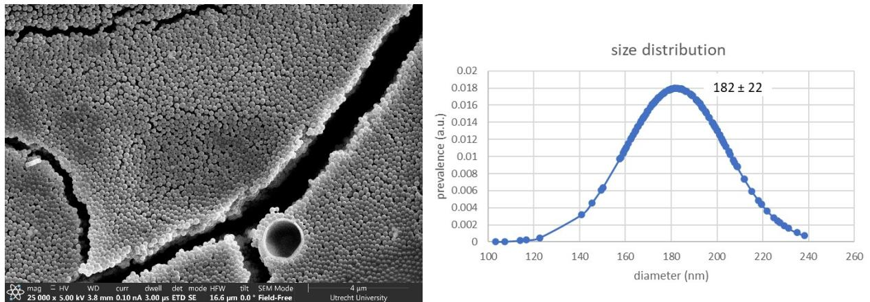
Figure S 3: a) SEM images of the PMMA spheres used in templating; b) size distribution and average diameter of the counted PMMA spheres used for templating
