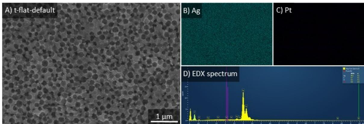
Figure S 4: a) SEM image of the t-flat-default sample, the corresponding EDX maps for b) Ag and c) Pt and the d) the EDX spectrum.
