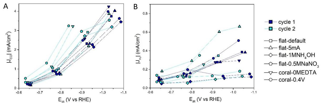
Figure S 15: partial current densities to a) CO and b) H<sub>2</sub> for the first and second cycle of catalysis of the electrodes t-flat-default, t-flat-5mA, t-flat-1MNH<sub>4</sub>OH, t-flat-0.5MNaNO<sub>3</sub>, t-coral-0MEDTA and t-coral-0.4V
