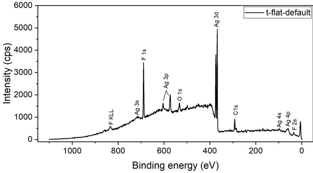
Figure S 6: X-ray photoelectron spectroscopy survey spectrum (Al  $\text{K}\alpha$  radiation,  $E_{\text{pass}}=100$  eV) of the t-flat-default electrode, indicating the presence of Ag, C, O and F.
