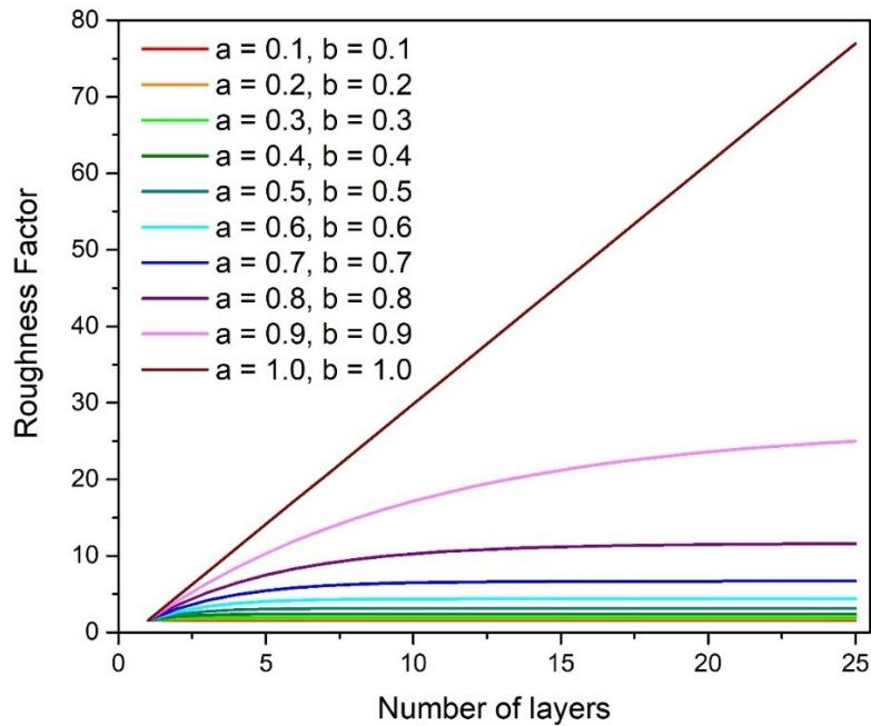
Figure S 11: Calculations of the Roughness Factor for when the parameter  $b$  is varied and  $a$  is kept constant.
