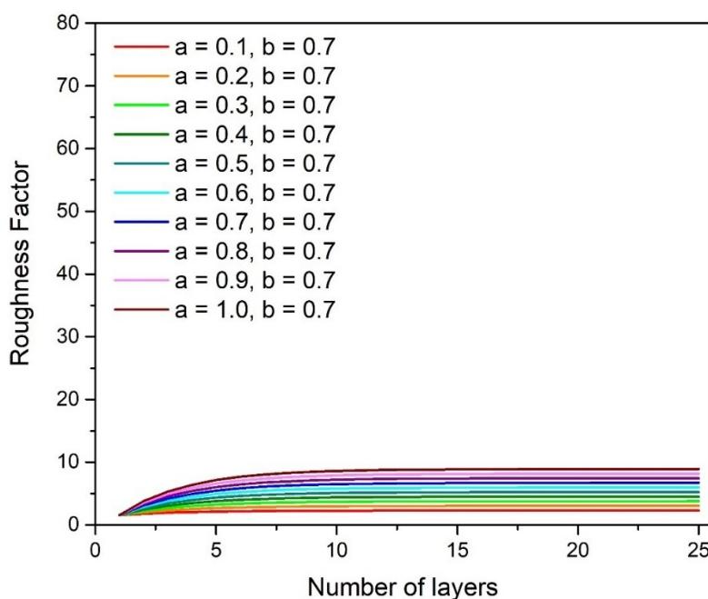
Figure S 10: Calculations of the Roughness Factor for when the parameter  $a$  is varied and  $b$  is kept constant.
