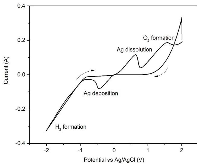
Figure S 1: cyclic voltammogram of the electrodeposition solution consisting of 0.05 M  $\text{AgNO}_3$ , 0.5 M  $\text{NH}_4\text{OH}$ , 1.0 M  $\text{NaNO}_3$  and 0.01 M EDTA run between 2 V and -2 V vs Ag/AgCl with a scan rate of 0.1 V/s.
