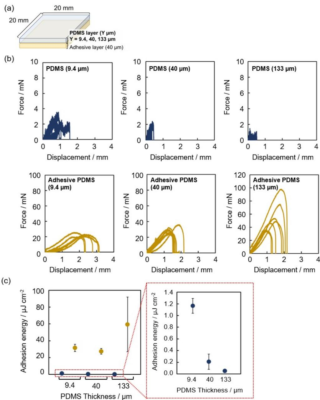
**Figure S7.** (a) The image of adhesive PDMS with the thickness of 9.4, 40, or 133  $\mu\text{m}$  PDMS layer. (b) Results of the tack separation tests of pristine PDMS and adhesive PDMS with each thickness of PDMS layer and (c) calculated adhesion energy values. (PDMS = polydimethylsiloxane).
