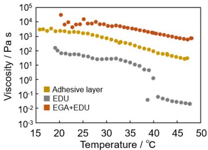
**Figure S8.** Temperature sweep measurements (viscosity vs. temperature) of the adhesive layer, EDU, and EGA+EDU. (EDU = 1-ethyl-3-(3-dimethylaminopropyl)urea; EGA = ethyl gallate).
