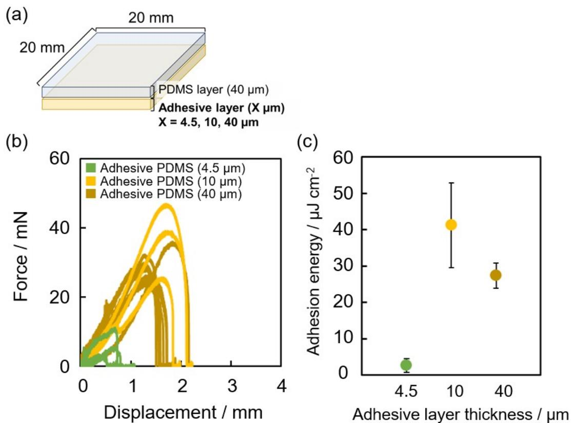
**Figure S6.** (a) The image of adhesive PDMS with the thickness of 4.5, 10, or 40 μm adhesive layer. (b) Results of the tack separation tests of adhesive PDMS with 4.5, 10, or 40 μm thick of adhesive layer and (c) calculated adhesion energy values. (PDMS = polydimethylsiloxane).
