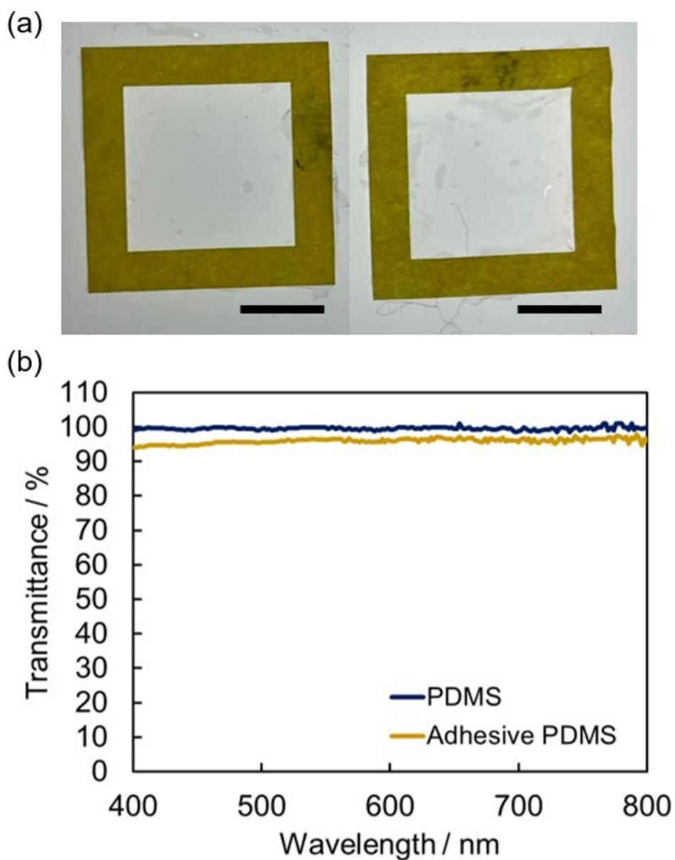
**Figure S4.** (a) Images of the pristine PDMS and adhesive PDMS films (scale bar = 1 cm), and (b) the results of ultraviolet-visible (UV-Vis) analysis of the films. (PDMS = polydimethylsiloxane).
