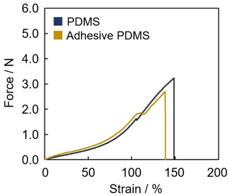
**Figure S5.** Tensile force during the tensile tests on PDMS and adhesive PDMS. (PDMS = polydimethylsiloxane).
