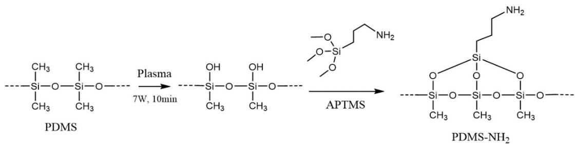
**Figure S1.** Silane-coupling reaction through hydroxyl groups of the plasma-treated PDMS using APTMS to introduce amino groups into the PDMS. (PDMS = polydimethylsiloxane; APTMS = 3-aminopropyltrimethoxysilane).
