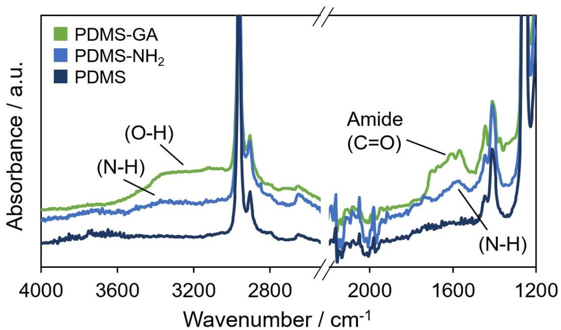
**Figure S2.** FT-IR spectra of pristine PDMS, aminated PDMS (PDMS-NH<sub>2</sub>), and gallol-introduced PDMS (PDMS-GA). (FT-IR = Fourier-transform infrared; PDMS = polydimethylsiloxane).
