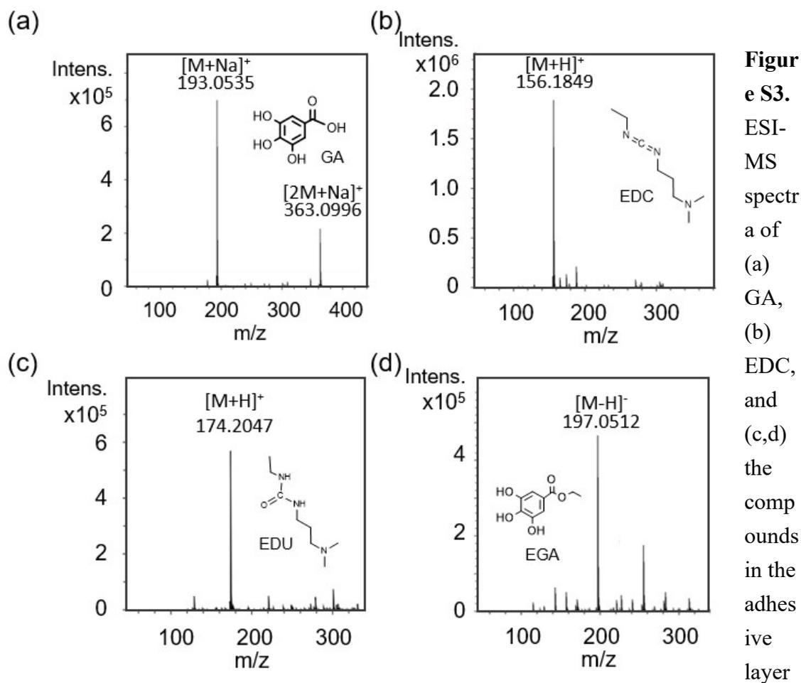
**Figure S3.** ESI-MS spectra of (a) GA, (b) EDC, and (c,d) the compounds in the adhesive layer
