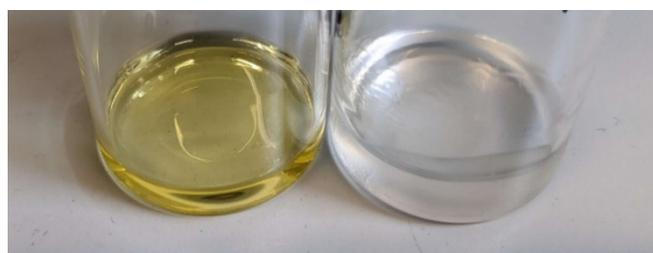
Figure S4. Photograph of poly(hexyl methacrylate-co-trifluoroethyl methacrylate) in THF after initial polymerisation step (left) and after post-polymerisation reduction (right).
