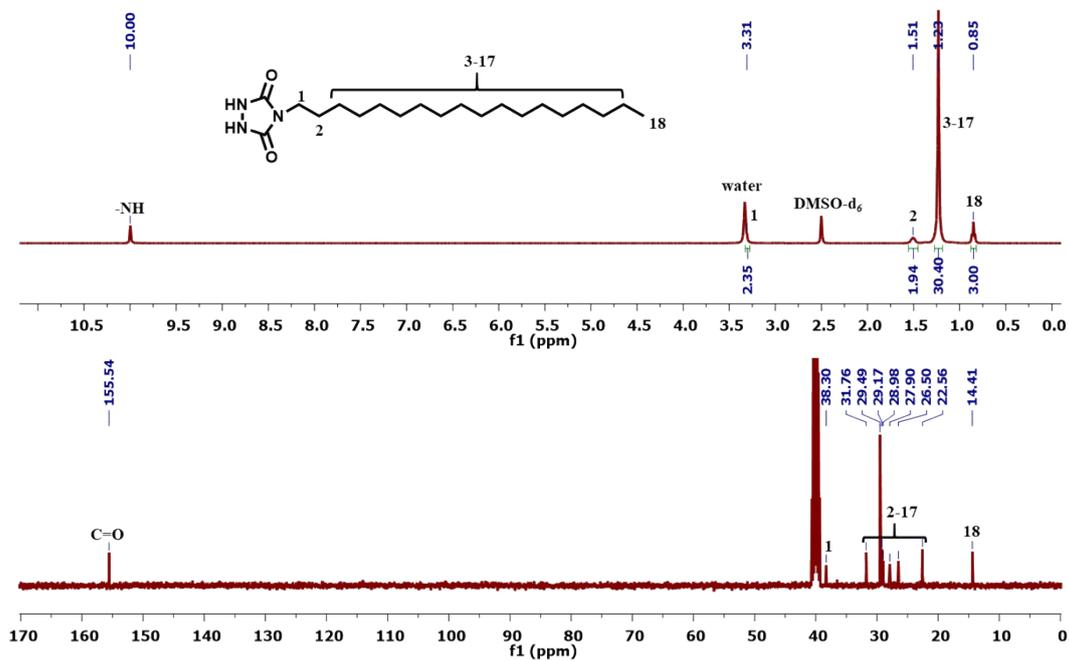
Figure S9:  $^1\text{H}$  &  $^{13}\text{C}$ -NMR spectra of  $\text{C}_{18}$ -urazole.
