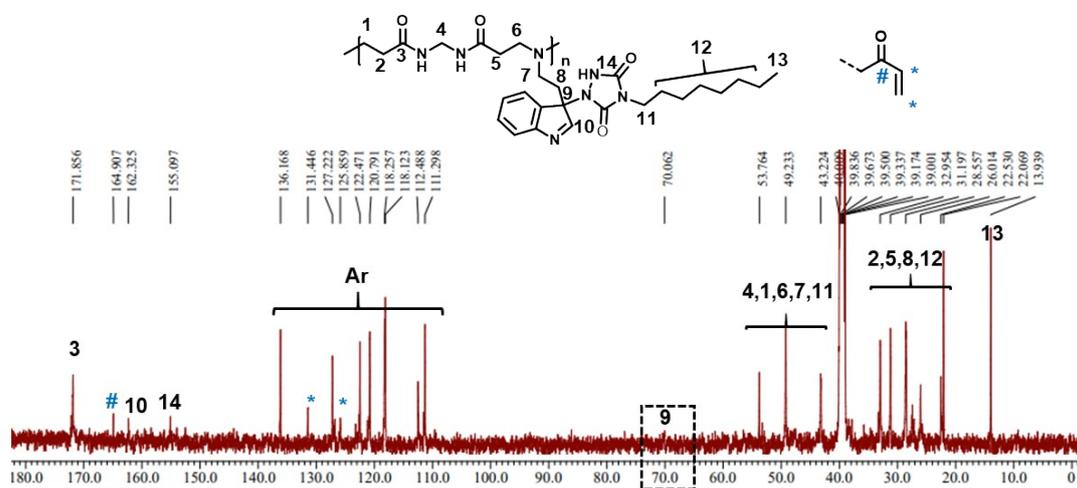
Figure S11:  $^{13}\text{C}$ -NMR spectra of PAA- $\text{C}_8$ -TAD.
