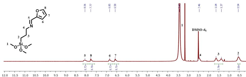
**Figure S20:**  $^1\text{H}$ -NMR spectra of FTMSPM (Note: small fraction of starting material was observed. The FTMSPM coated surface was washed with ethanol to remove this unreacted material).
