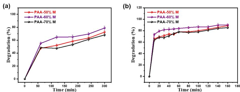
**Figure S22:** Degradation kinetics of crosslinked PAA (PAA-50% M, PAA-60% M and PAA-70% M) at (a) 0.01M NaOH solution (pH 12) and (b) 0.1M NaOH solution (pH 13) via gravimetric method.
