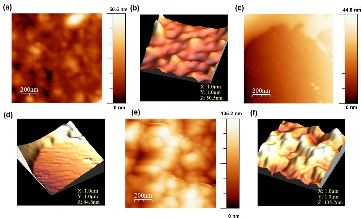
**Figure S21:** (a) & (c) are the 2D AFM image and (b) & (d) are the 3D AFM image of indolized-PAA coated surface at layer-2 and layer-3 respectively, (e) & (f) are the 2D and 3D AFM image of indolized-PAA coated surface (layer-1) functionalized with C<sub>18</sub>-TAD.
