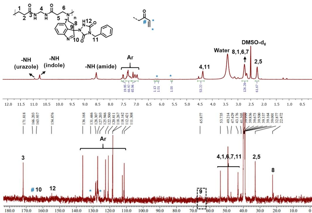
Figure S14:  $^1\text{H}$  &  $^{13}\text{C}$ -NMR spectra of PAA-Benzyl-TAD.
