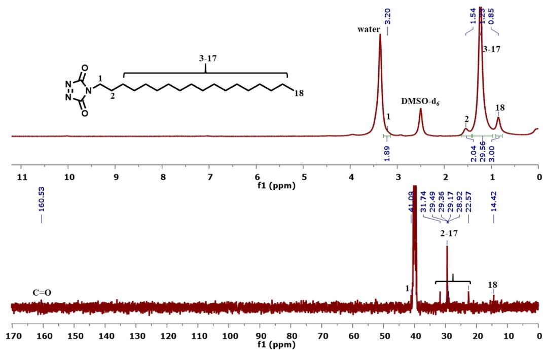
Figure S10:  $^1\text{H}$  &  $^{13}\text{C}$ -NMR spectra of  $\text{C}_{18}$ -TAD.
