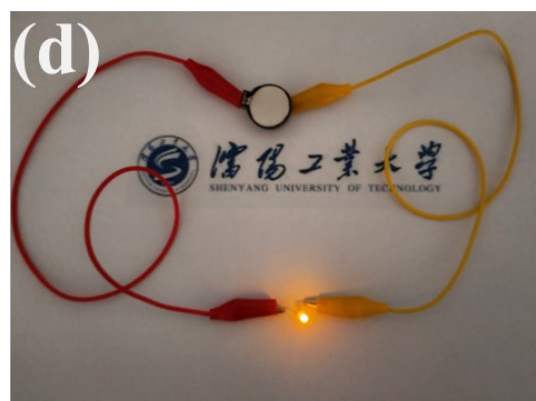
Figure S9 The full cell illuminates different LEDs with different working potentials for red (1.8–2.4 V), blue (2.8–3.4 V), green (1.8–2.4 V), and yellow (1.8–2.4 V).
