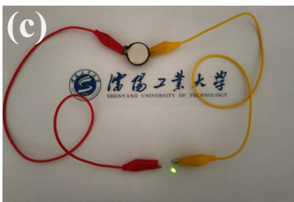
Figure S9 The full cell illuminates different LEDs with different working potentials for red (1.8–2.4 V), blue (2.8–3.4 V), green (1.8–2.4 V), and yellow (1.8–2.4 V).
