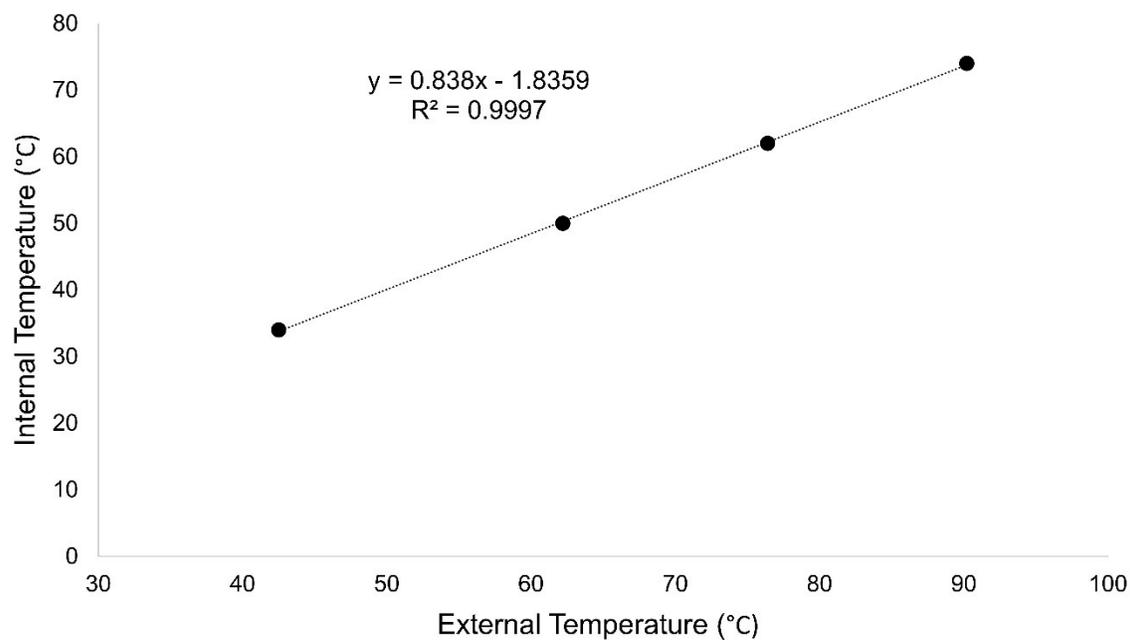
**Figure S135.** Hot plate temperature calibration curve.
