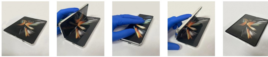
Fig. S32. Photographs showing the IPU-30BC can be used as a film for folding screen phones.
