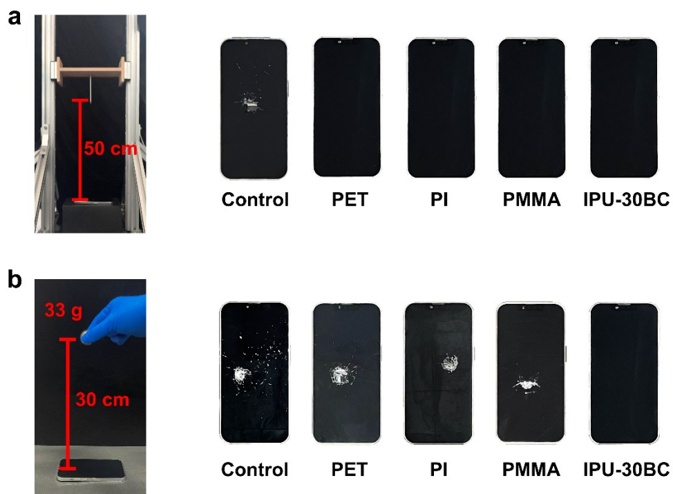
Fig. S33. The protective ability of IPU-30BC and common rigid materials. (a) A needle-shaped impactor fell from a height of 50 cm, The IPU-30BC and other rigid coatings can protect the phone from puncture; (b) A 33g ball fell from a height of 30 cm and hit the phone, only IPU-30BC can protect it.
