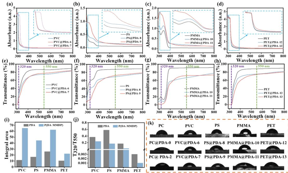
**Figure S11. UV absorption enhancement of MMDP-doped PDA coatings. (a)-(d)**
