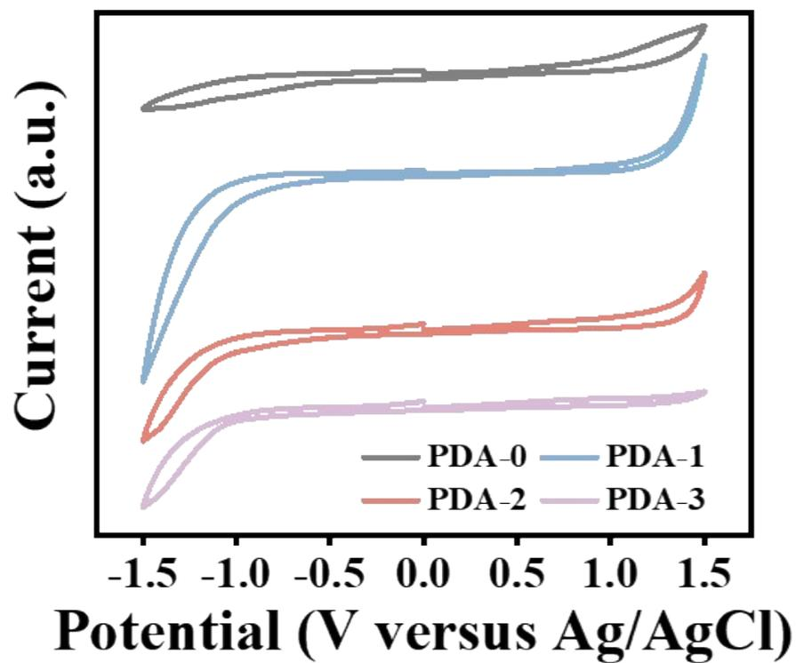
Figure S4. Cyclic voltammograms testing of the PDA coatings.
