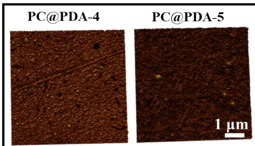
Figure S8. 3D AFM height images of PC@PDA-*i* coating, where *i* = 4-5.
