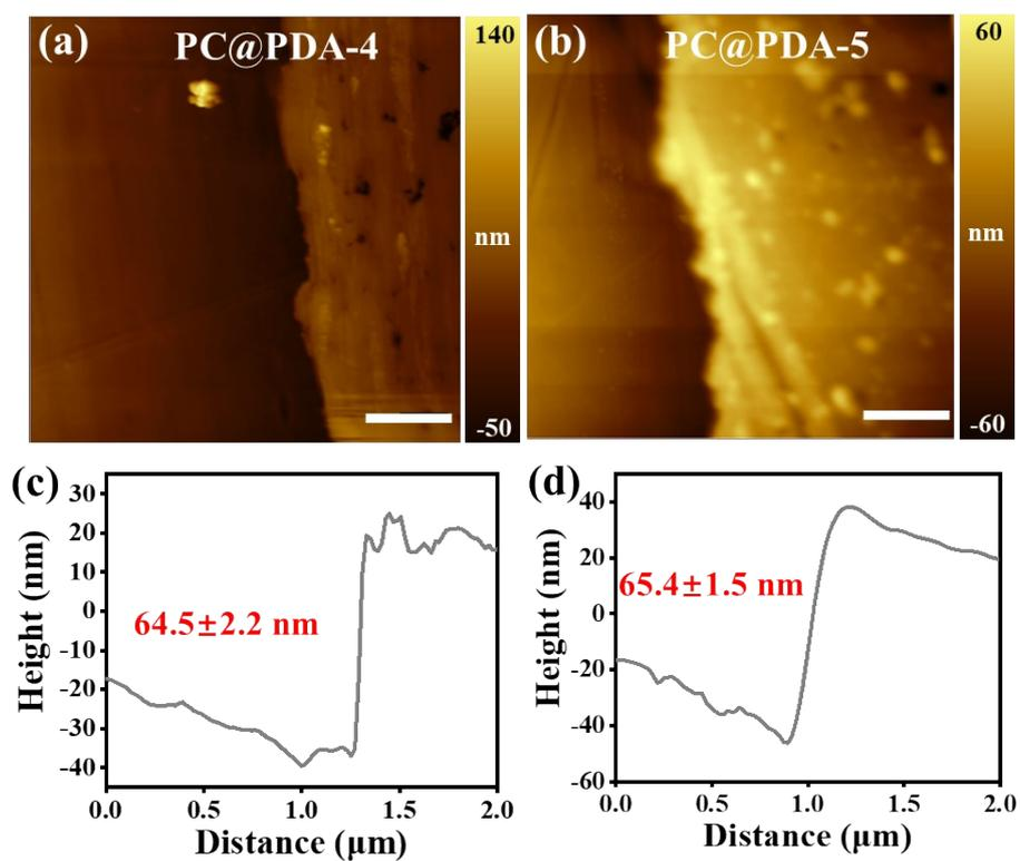
Figure S9. Thickness of PDA coatings. (a)-(b) AFM images of PDA coatings, respectively, (a) PC@PDA-4, (b) PC@PDA-5, scale bars, 1  $\mu\text{m}$ . (c)-(d) Corresponding height chart, respectively, (c) PC@PDA-4, (d) PC@PDA-5.
