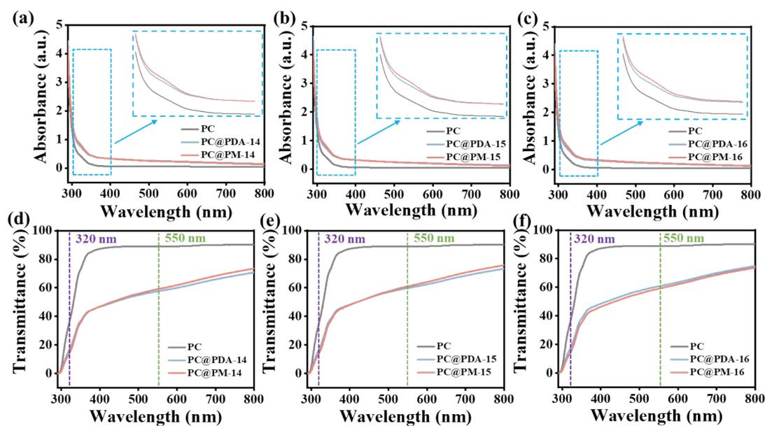
Figure S15. Effect of reaction pH on UV absorption of PDA coatings. (a)-(c) UV-
