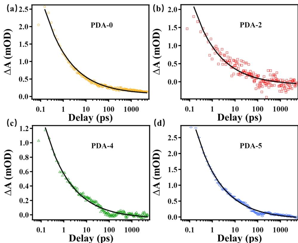
Figure S14. The EIA kinetics traces of PDA-*i* (*i*= 0, 2, 4 and 5). These traces can be described by a power law function with a power of  $-0.377 \pm 0.006$ .
