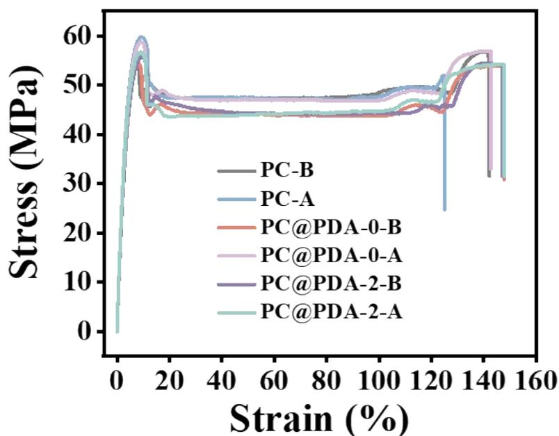
**Figure S20. Stress-strain curves of naked PC and PDA coated PC (PC@PDA-0 and PC@PDA-2) before and after UV irradiation.**
