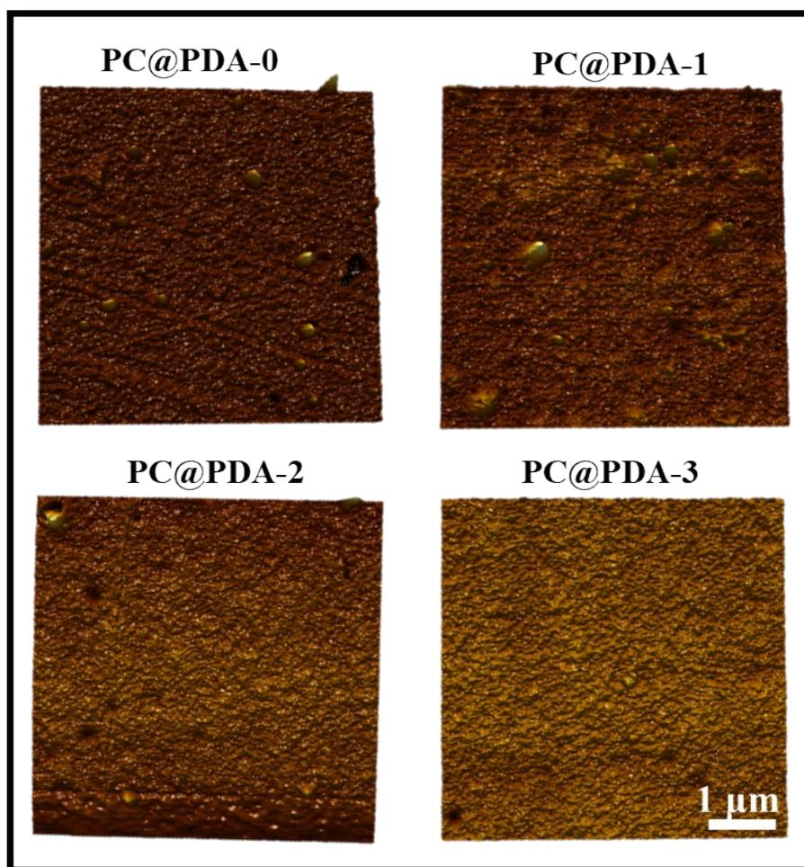
**Figure S1.** 3D AFM height images of PC@PDA-*i* coating, where *i* = 0-3.
