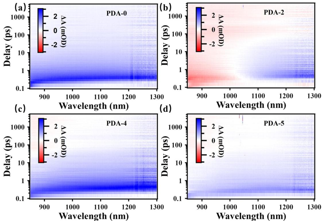
**Figure S12. Pseudocolor images of the TA spectra at all decays.** The horizontal and vertical axes corresponding to the probe wavelength and pump-probe delay, respectively. As indicated by the color scale bar, the color intensity represents the magnitude of the TA signal.
