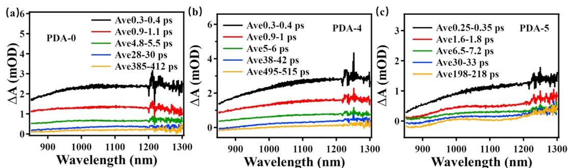
**Figure S13. Transient absorption spectra of PDA-*i* (*i*=0, 4 and 5) at indicated delay times.**
