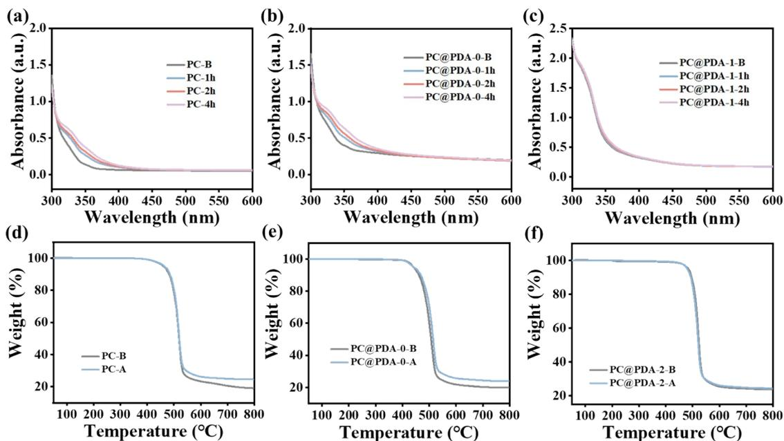
**Figure S19. UV protection of MMDP-doped PDA coatings.** (a)-(c) UV-Vis absorption spectra of naked PC and PDA coated PC (PC@PDA-0 and PC@PDA-2) after UV irradiation for different times, respectively, (a) naked PC, (b) PC@PDA-0, (c) PC@PDA-2. (d)-(f) TGA curves of naked PC and PDA coated PC (PC@PDA-0 and PC@PDA-2).
