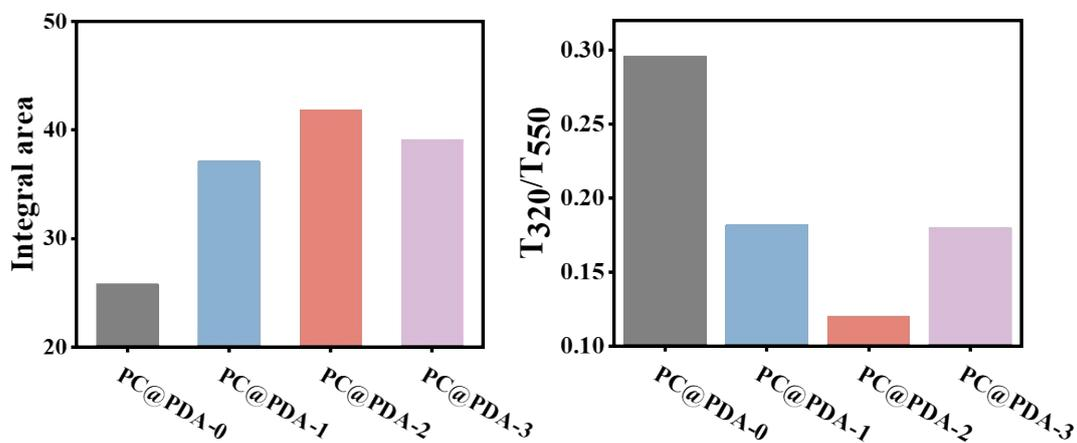
**Figure S3. Quantitative analysis of the UV enhancement of PDA coatings.** (a) Integral area values of UV absorption curve (shown in Figure 2a) from 290 to 400nm. (b) The ratio of transmittance at 320 nm and 550 nm in UV transmittance curve (shown in Figure 2b).
