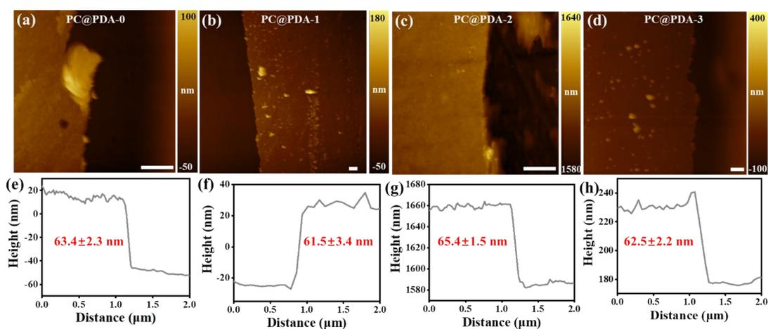
**Figure S2.** Thickness of PDA coatings. (a)-(d) AFM images of PDA coatings, respectively, (a) PC@PDA-0, (b) PC@PDA-1, (c) PC@PDA-2, (d) PC@PDA-3, scale
