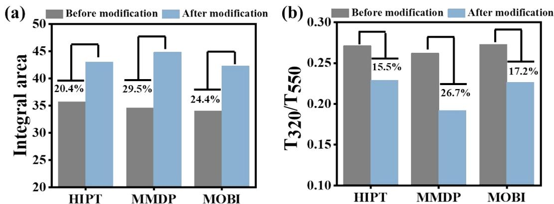
**Figure S18. Quantitative analysis of the UV enhancement.** (a) Integral area values of UV absorption curve (shown in Figure 3e-3g) from 290 to 400nm. (b) The ratio of transmittance at 320 nm and 550 nm in UV transmittance curve (shown in Figure 3h-3j).
