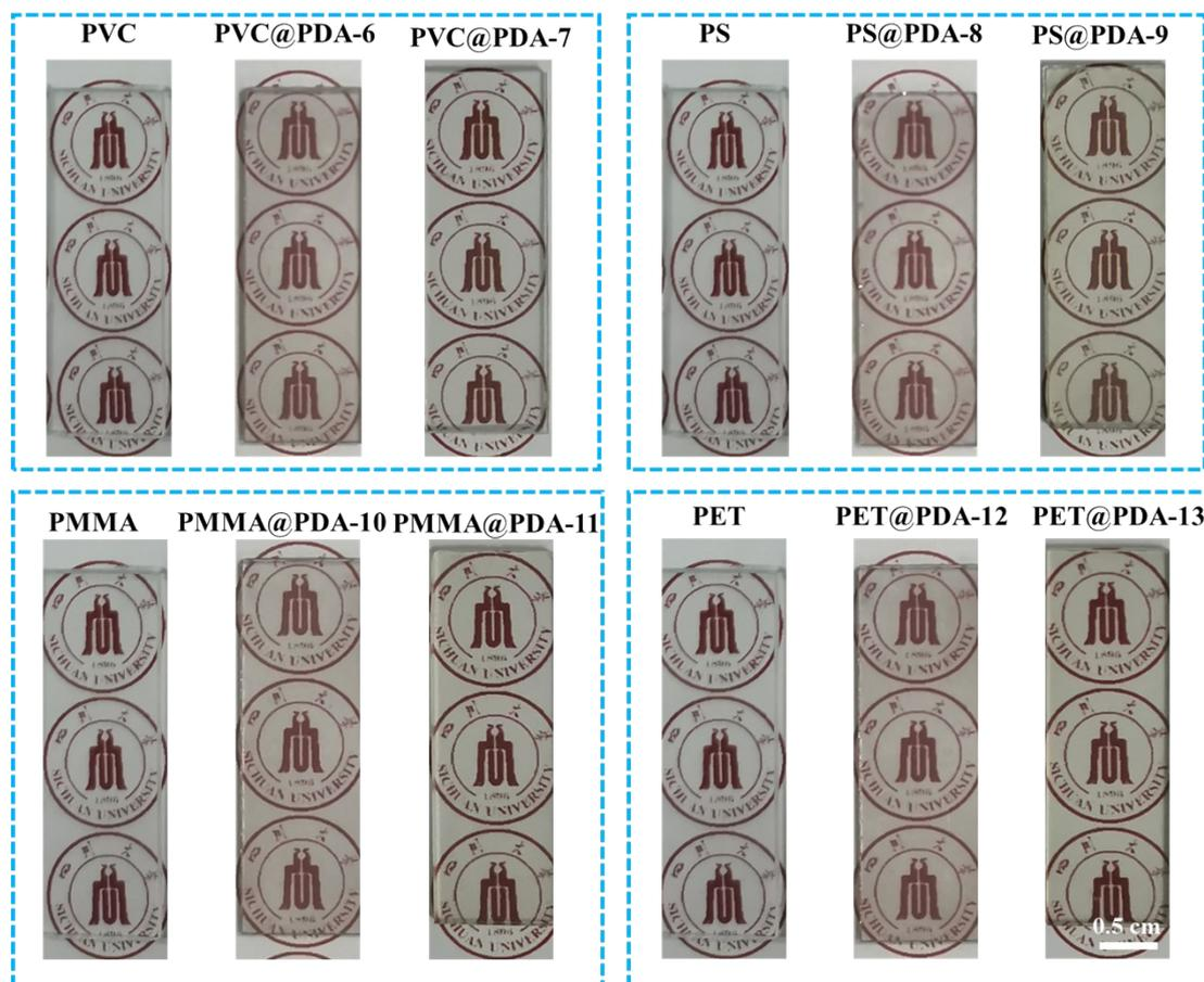
**Figure S10. Optical images of different substrates uncoated and coated with PDA.**
