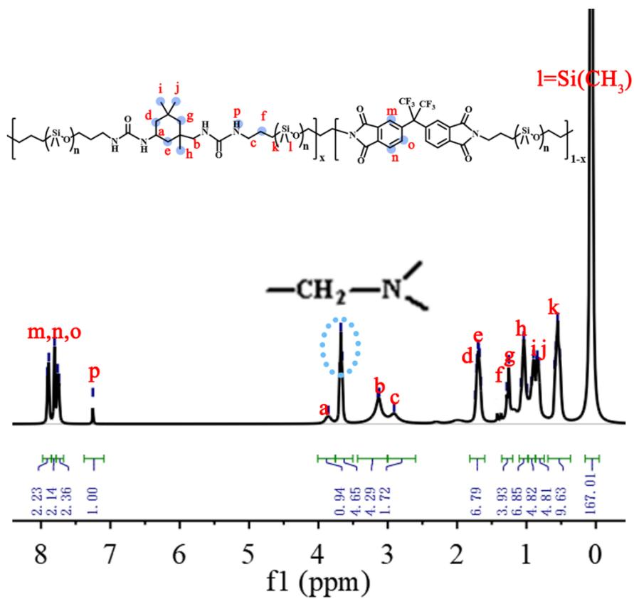
Fig. S4. <sup>1</sup>H NMR of the PSiPI-5 elastomer.
