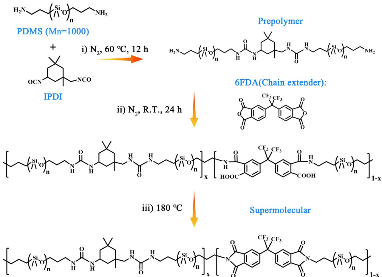
**Fig. S1.** Schematic of the synthetic routes of PSiPI elastomer.
