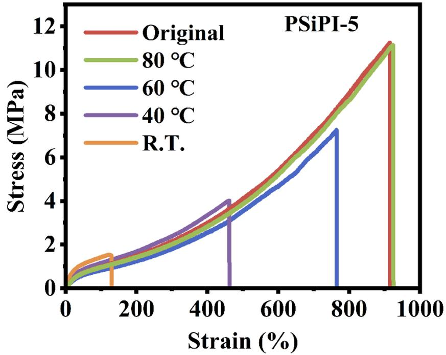
**Fig.S13.** The stress-strain curve of the self-healing properties of PSiPI-5 elastomer at different temperatures.
