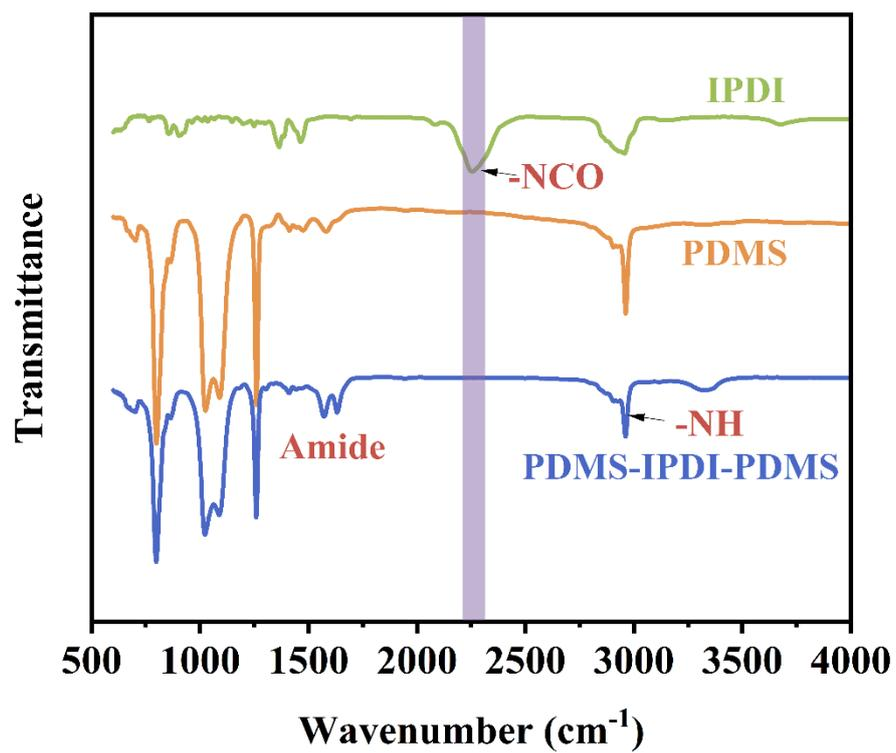
Fig. S2. FTIR spectra of monomer IPDI, PDMS and precursors.
