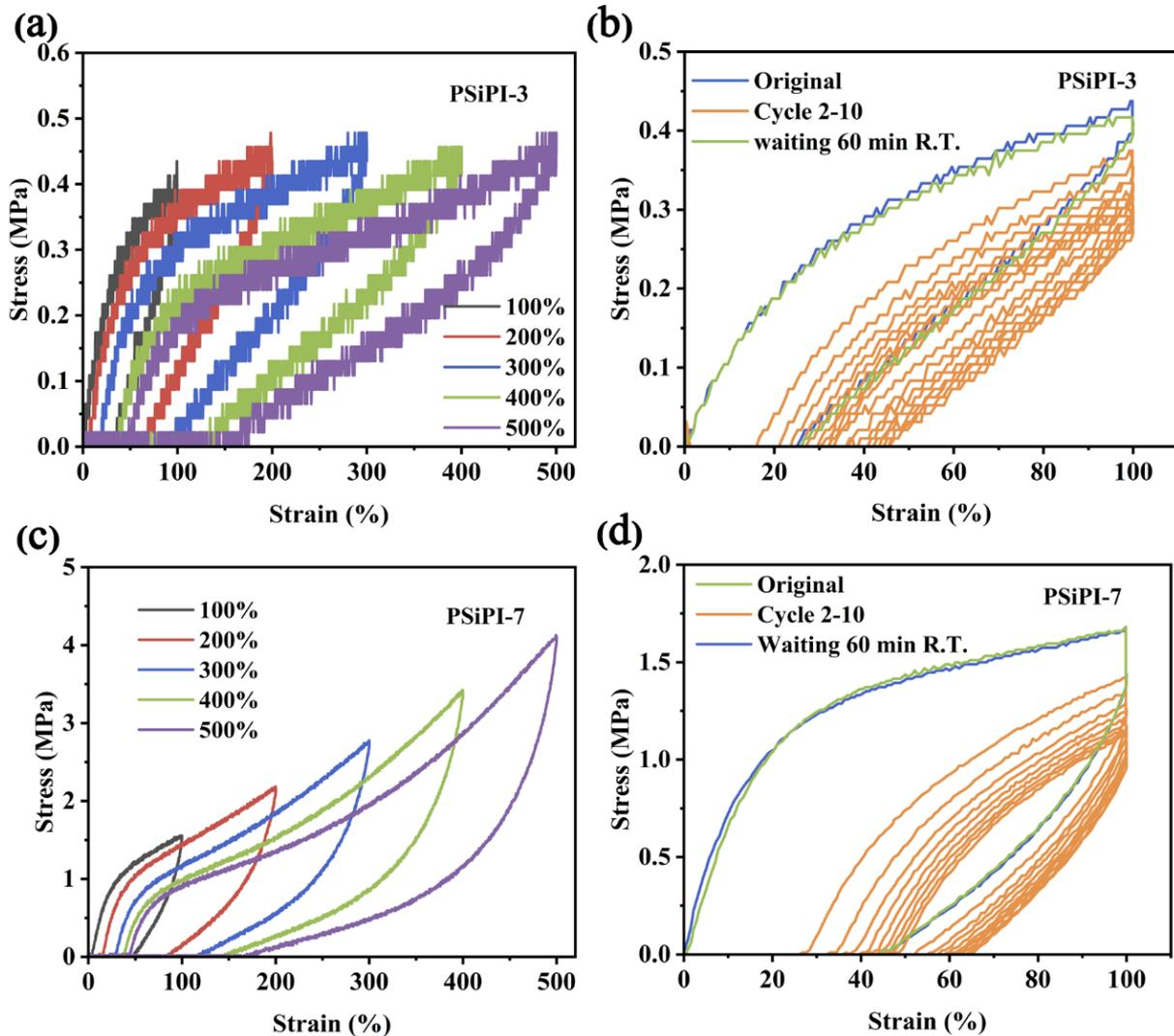
**Fig. S12.** (a) and (c) Cycling loading-unloading curves of PSiPI-3 and PSiPI-7 elatomers at 100%, 200%, 300%, 400%, and 500% strains; (b) and (d) Cycling curve of PSiPI-3 and PSiPI-7 elatomers at 100% strain for 10 cycles, relaxing for 1 hour, with the cycle curve coinciding with the first cycle completely.
