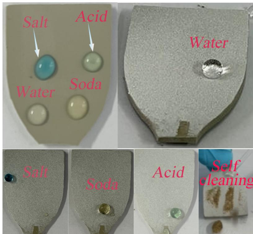
**Fig. S17.** Spraying  $\text{SiO}_2\text{-FSi-PSiPI-5}$  on Silicone Rubber Surfaces Hydrophobic corners obtained by spension (blue: salt droplets, yellow: alkali droplets, green: acid droplets and colourless: water droplets).
