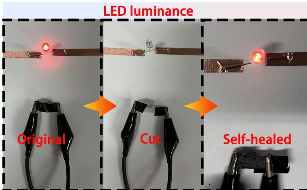
**Fig. S19.** PSiPI-5 doped with MWCNTs forms a closed conductive circuit after connecting to the circuit, which includes an LED that is cut and recovers after healing.
