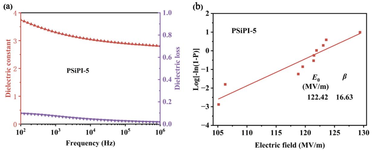
**Fig. S15.** (a) Plot of the dielectric properties of PSiPI-5 and (b) Weibull breakdown strength distribution.
