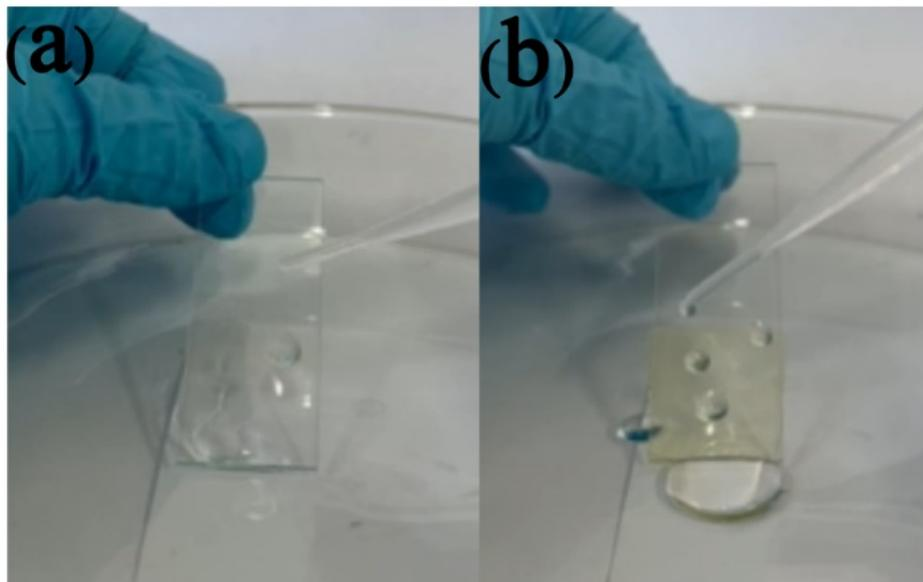
**Fig. S16.** Water sliding test on unlined and P*SiPI*-5 substrates.
