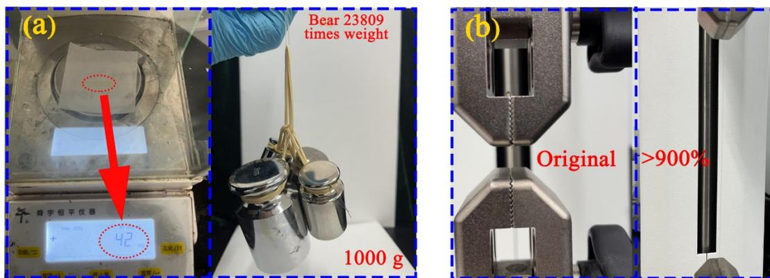
**Fig. S11.** (a) The PSiPI-5 sample can withstand 23809 times its weight. (b) PSiPI-5 has good ductility.
