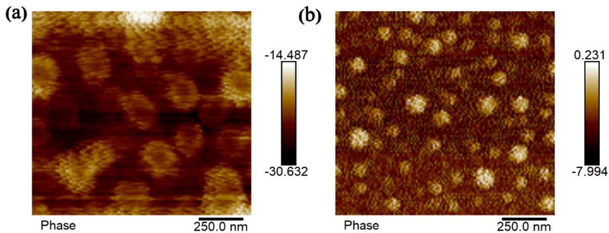
**Fig. S6.** (a) AFM phase diagrams of PSiPI-3 and (b) PSiPI-7. Dark regions represent the soft phase, while bright regions represent the hard phase, indicating the microphase separation structure of both.
