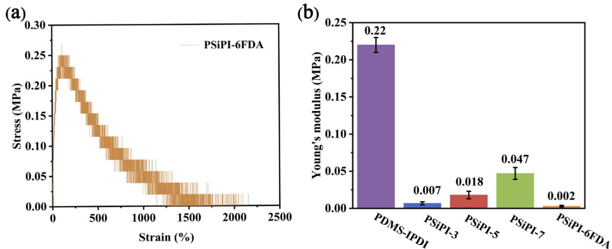
**Fig. S10.** (a) Stress-strain diagram of PSiPI-6FDA. (b) Young's modulus of PSiPI with different molar ratios.
