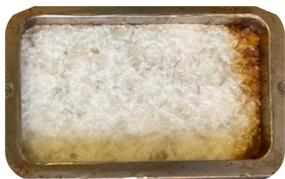
Figure S8. The lack of processability of the reference network (comprising no BAE bonds) was observed through compression molding (2 tons of pressure, at 150 °C, for 30 min).
