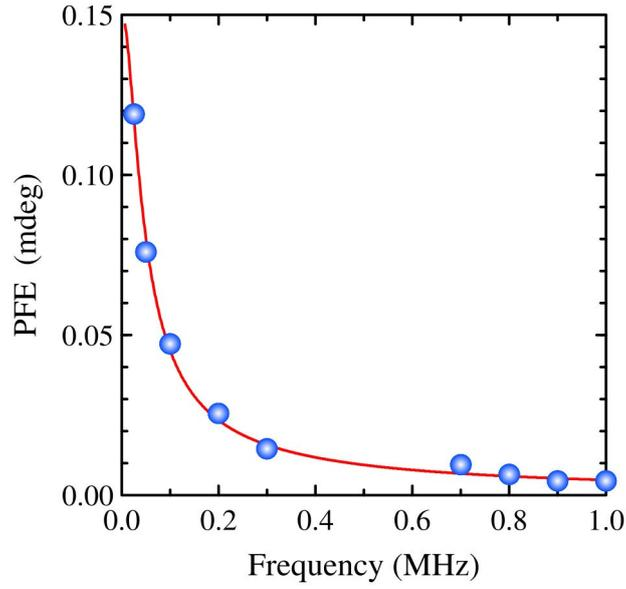
**Fig. S4.** Dependence of the PFE amplitude on the pump modulation frequency  $f$ : experimental values (blue dots) and their fit to  $PFE(f) = PFE(0)/\sqrt{1 + (2\pi f\tau_{pol})^2}$  (red line), where  $\tau_{pol}$  is the MP lifetime ( $\approx 5 \mu\text{s}$ ).
