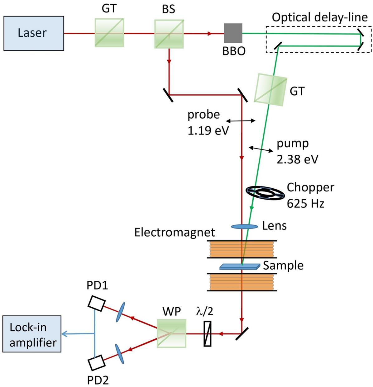
**Fig. S1.** Experimental setup for the PFE studies in EuO; GT is a Glan-Thompson polarizer, BS – a beam splitter, BBO – a crystal of  $\beta$ -BaB<sub>2</sub>O<sub>4</sub>,  $\lambda/2$  – a half-wave plate, WP – a Wollaston prism, PD1 and PD2 – photodiodes.
