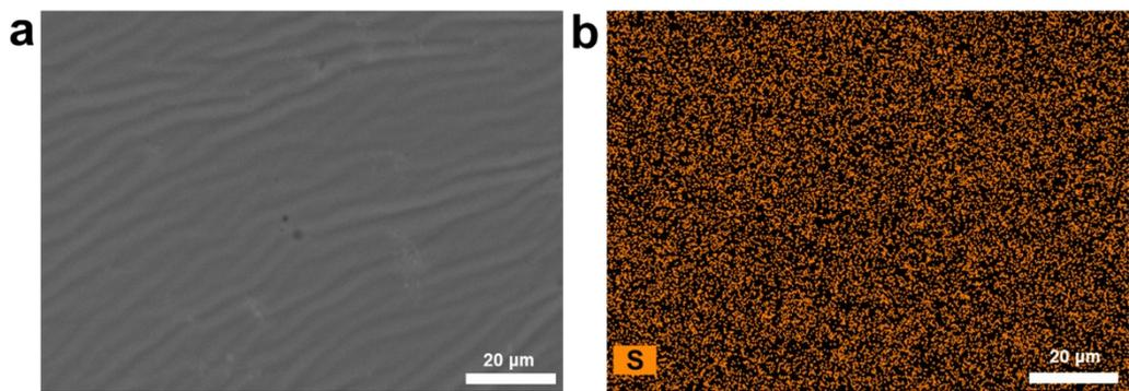
**Figure S2.** (a) SEM image of the PAHCDS-0.50 gel and (b) the EDS mapping of S element.
