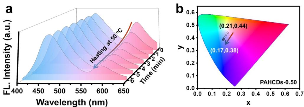
Figure S13. The fluorescence spectra (a) and corresponding CIE (1978) chromaticity diagram of PAHCDs-0.50 gel that was recorded at different time intervals after being heated at 50 °C.
