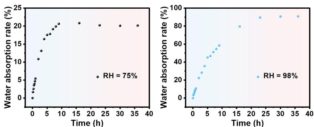
**Figure S3.** The time-dependent water absorption rate of the PAHCDS-0.50 gel in both normal (75% RH) and extreme (98% RH) conditions.
