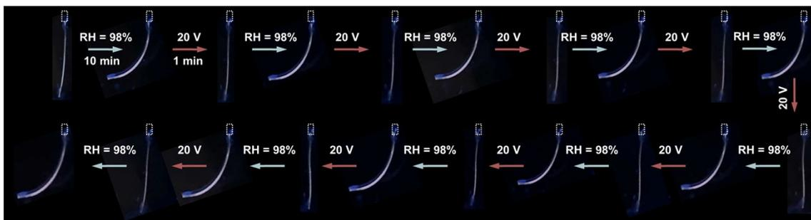
**Figure S18.** Fluorescent photos showing the humidity/electroheat-triggered reversible actuation behavior of HEFC actuator.
