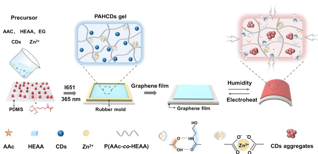
**Figure S15.** Illustration showing the preparation process of HEFC actuator.
