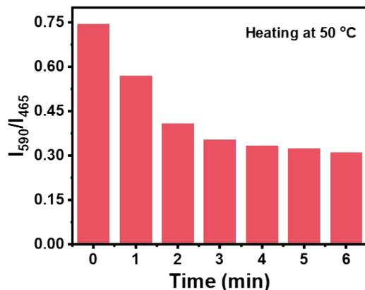
**Figure S14.** Fluorescence intensity ratio ( $I_{590}/I_{465}$ ) of PAHCDS-0.50 gel as the function of the heating time at 50 °C ( $\lambda_{ex} = 365$  nm).
