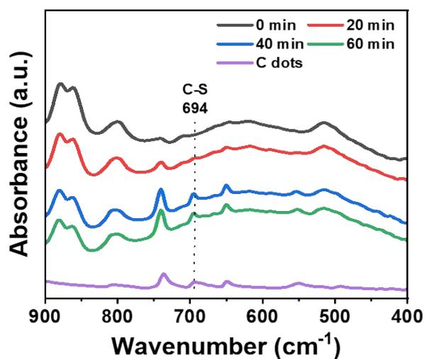
Figure S12. FT-IR spectra of CDs and PAHCDs-0.50 gel that was exposed to 98% RH for different time.
