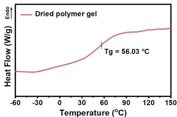
Figure S17. Differential scanning calorimetry (DSC) curve of dried polymer gel.
