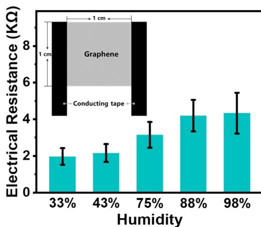
**Figure S16.** The electrical resistance of graphene film under different environmental humidity.
