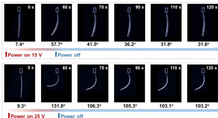
Figure S19. Fluorescent photos showing the actuation behavior of HEFC actuator after 15 V and 25 V voltage were turned off, respectively.
