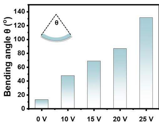
Figure S18. The bending angle of HEFC actuator under different voltage.
