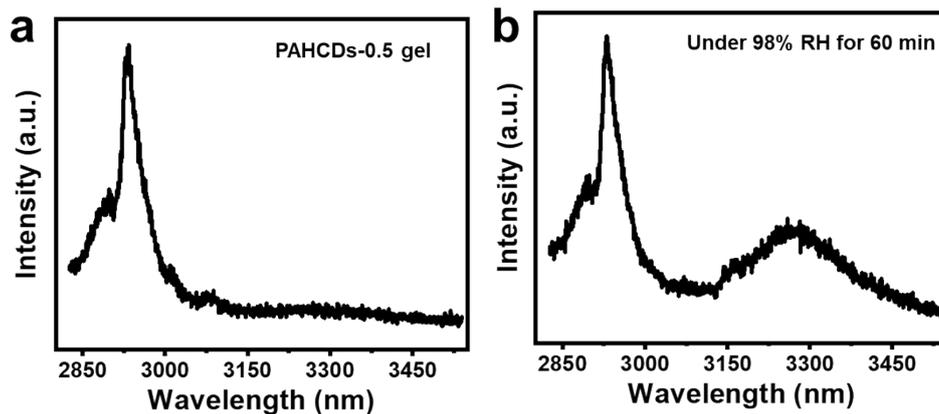
Figure S11. Raman spectra of PAHCDs-0.5 gel before (a) and after (b) being under RH of 98% for 60 min.
