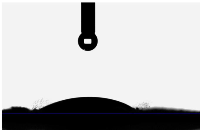
**Fig. S5** The static water contact-angle measurement of Bulk-C<sub>3</sub>N<sub>4</sub>.
