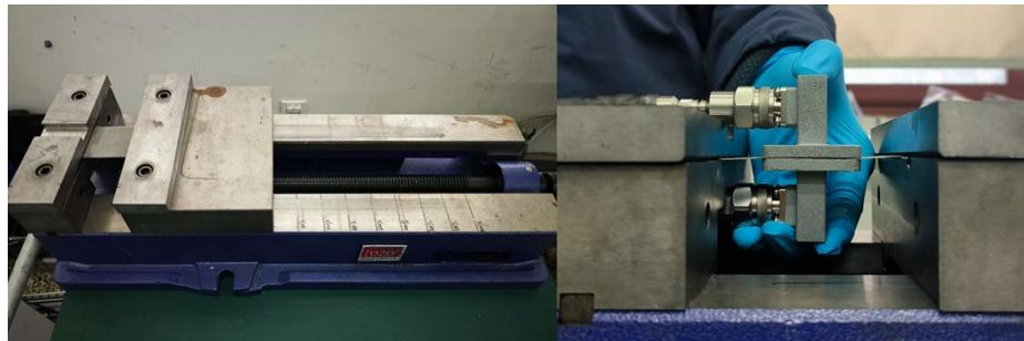
**Figure S7.** Digital photograph of EMI SE testing process during stretching.
