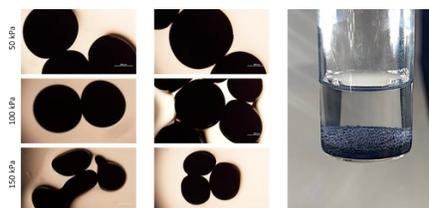
**Figure S6.** Influence of jetting conditions on MXene droplet size. The image shows a series of MXene droplets produced under different jetting conditions, with variations in droplet size evident.
