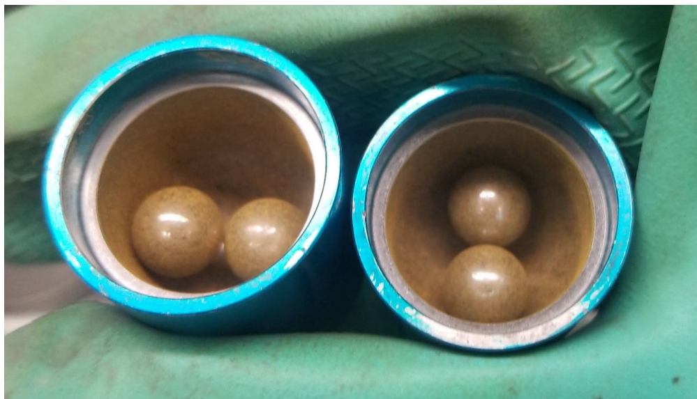
Figure S21. \text{AsI}_3 ground in the mixer mill at 10 Hz for 5 min. (left) or 10 min. (right).
