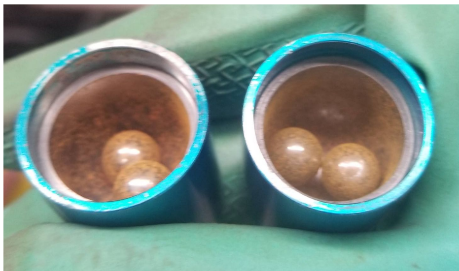
Figure S20. \text{AsI}_3 ground in the mixer mill at 10 Hz for 1 min (left) or 2 min (right).
