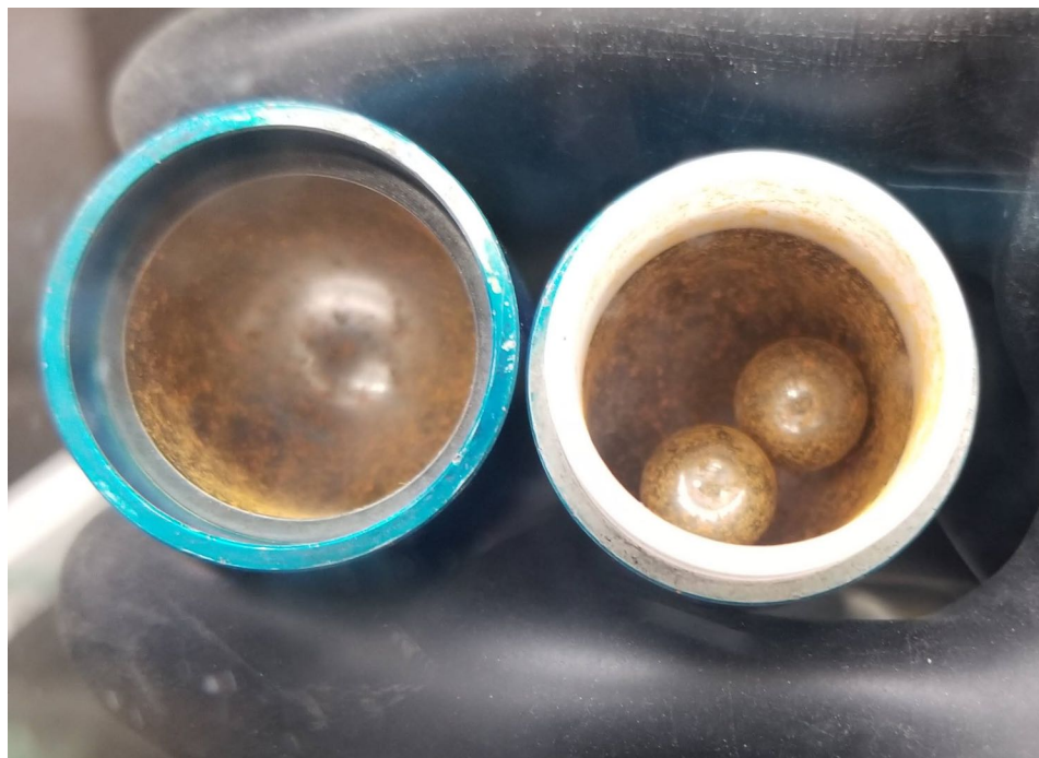
Figure S19. \text{AsI}_3 ground in the mixer mill at 10 Hz for 30 s.
