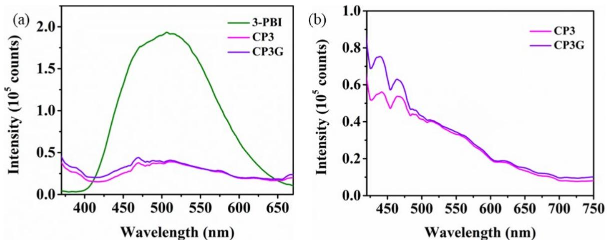
**Figure S7.** Solid state PL spectra of (a) 3-PBI, CP3 and CP3G at 350 nm excitation, (b) CP3 and CP3G at 400 nm excitation.
