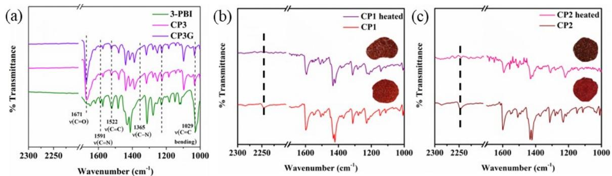
**Figure S4.** Comparison of FT-IR spectra of (a) 3-PBI, **CP3** and **CP3G**, (b) **CP1** before and after heating and (c) **CP2** before and after heating.
