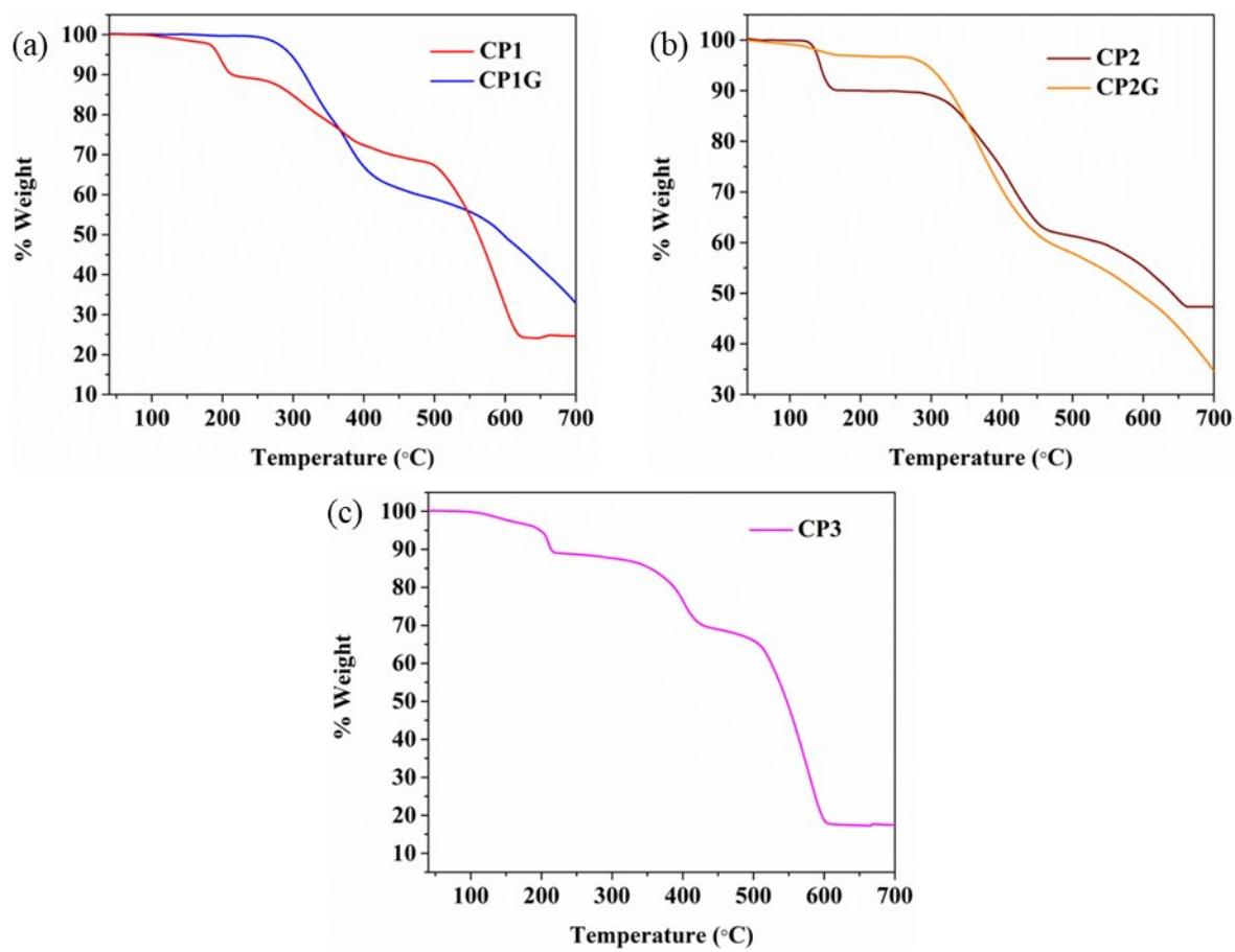
**Figure S5.** Thermogravimetric Analysis of (a) CP1 and CP1G, (b) CP2 and CP2G and (c) CP3.
