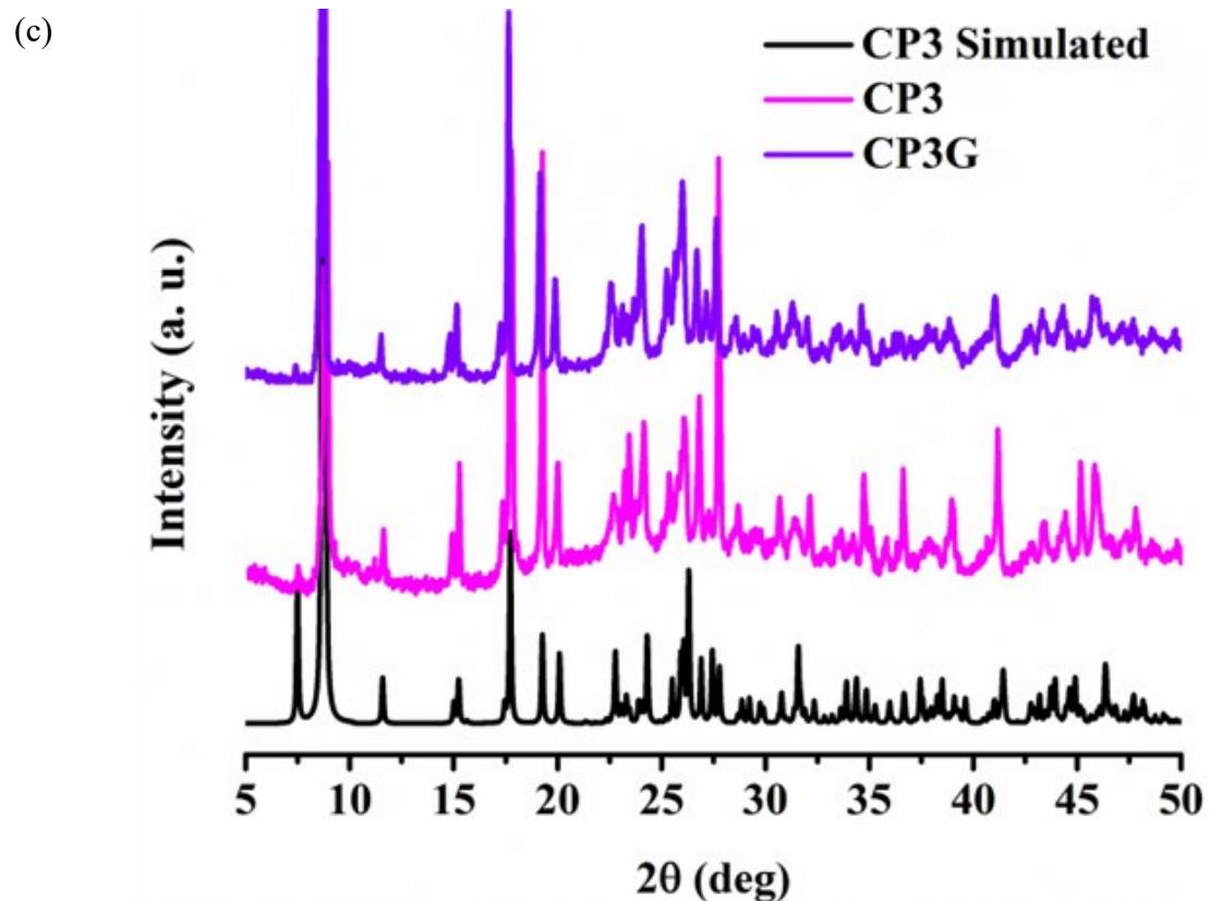
**Figure S3.** PXRD patterns of simulated, as-synthesized and ground CPs- (a) CP1, (b) CP2, (c) CP3.
