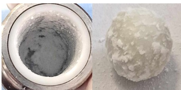
Figure S9 : Picture of the bead and milling jar after 60minutes of milling by using NaOH as racemizing agent and NaCl as solid lubricant
