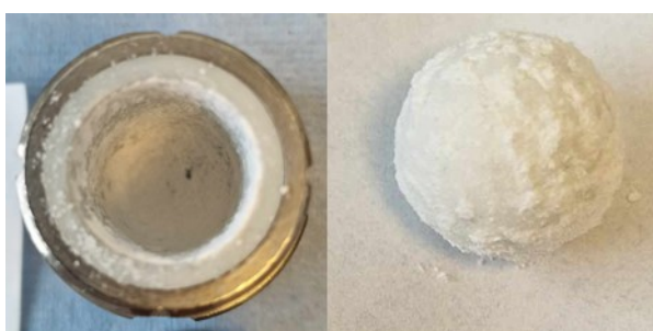
Figure S10 : Picture of the bead and milling jar after 60minutes of milling by using NaOH as racemizing agent and NaCl as solid lubricant. Glove bag has been used for the filling step.
