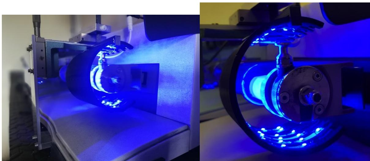
Figure S1. Modified vibratory ball-mill with LEDs
