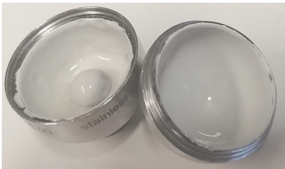
Figure S5. Photograph of the product of milling PET (704 mg), NaOH (294 mg), and 667 \mu\text{L} of \text{H}_2\text{O} at a frequency of 50 Hz for 2 h. 10 mL stainless steel milling jar with one 10 mm stainless steel milling ball was used.
