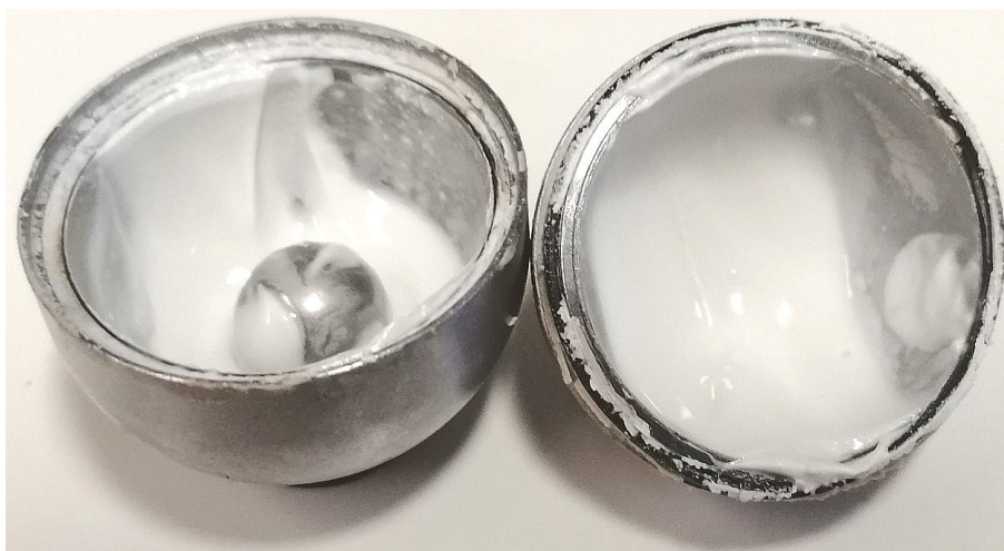
Figure S6. Photograph of the product of milling PET (631 mg), KOH (369 mg), and 667 \mu\text{L} of \text{H}_2\text{O} at a frequency of 50 Hz for 2 h. 10 mL stainless steel milling jar with one 10 mm stainless steel milling ball was used.
