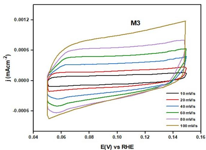
**Figure S3.** Non-faradic region cyclic voltammogram at various scanning rates of (a) M1, (b) M2 and (c) M3.
