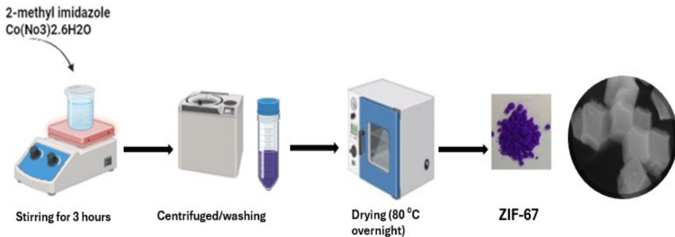
**Scheme S3** Synthesis scheme for Zif67 preparation
