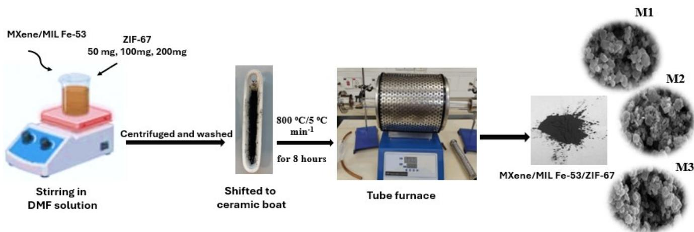
**Scheme S4.** Schematic diagram for the synthesis of MXene/MIL Fe-53/ZIF67 composite.
