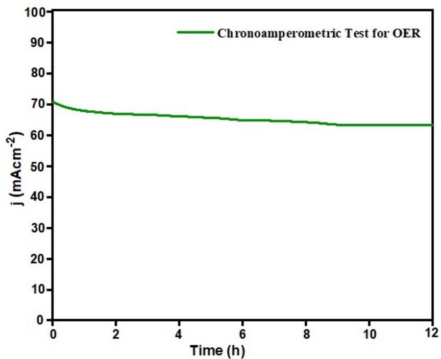
**Figure S4.** Chronoamperometric test for OER in 1 M KOH electrolyte
