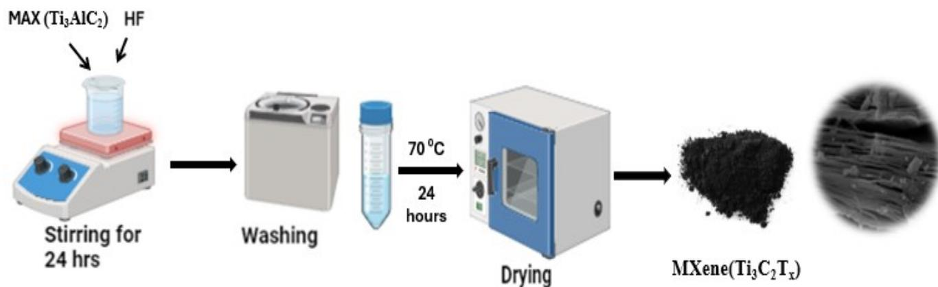
Scheme S1 synthesis scheme for MXene preparation from MAX phase.
