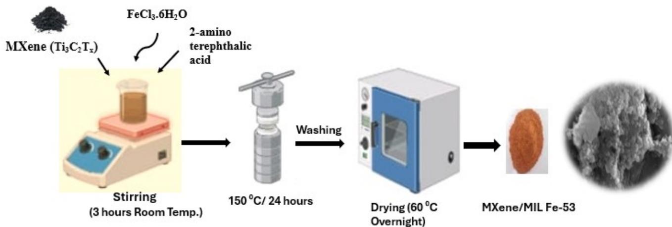
Scheme S2 Synthesis scheme for MILFe53/MXene hybrid preparation
