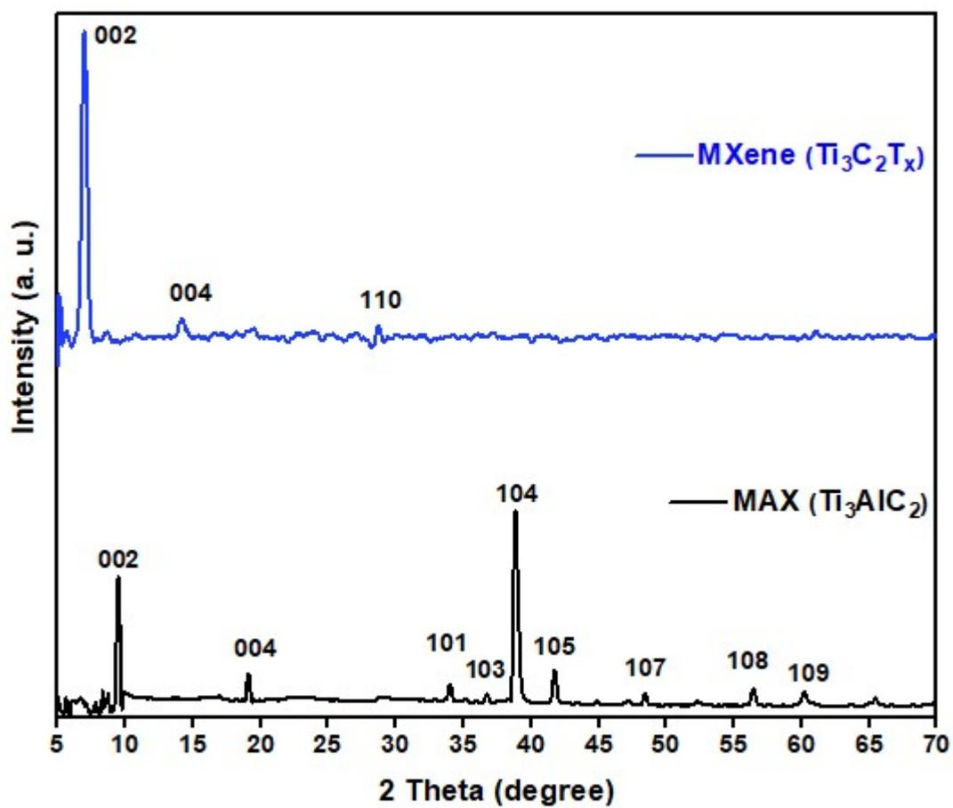
**Figure S1.** XRD pattern of MAX ( $\text{Ti}_3\text{AlC}_2$ ) and MXene ( $\text{Ti}_3\text{C}_2\text{T}_x$ ).
