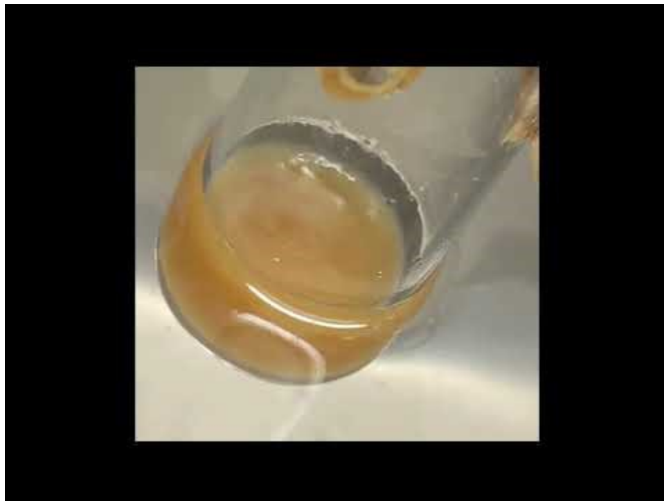
Figure S2: A 15x timelapse of the sonochemical hydrosilylation of 9 nm Si NPs with AIBN and 1-dodecene, showing the transition from opaque orange/brown to a transparent dark red solution.
