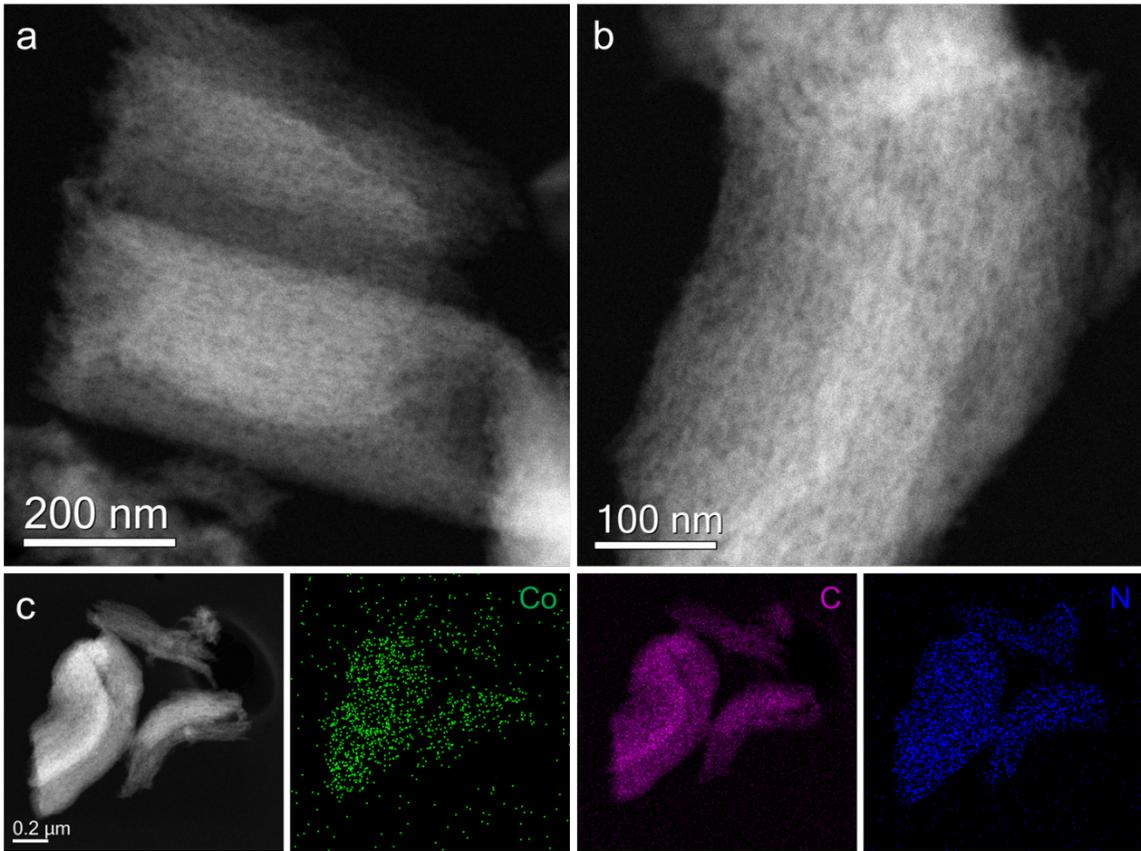
**Figure S2.** STEM and EDS mapping images of the as-synthesized Co-100-NAC-800. (a,b) STEM images showing order pore structure; (c) EDS mapping images showing the uniform distribution of Co, N, and C.
