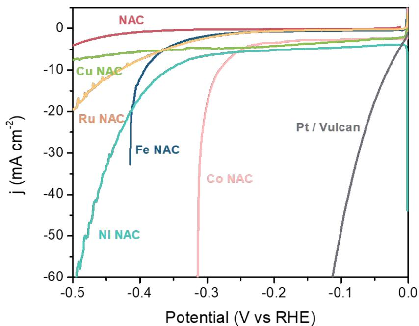
**Figure S8.** LSV of different transition metal single-atom on NAC for HER. 1 M KOH as electrolyte, M-NAC on carbon fiber paper as working electrode, Pt as counter electrode, Ag/AgCl as reference electrode. A Nafion membrane separates working and counter electrodes.
