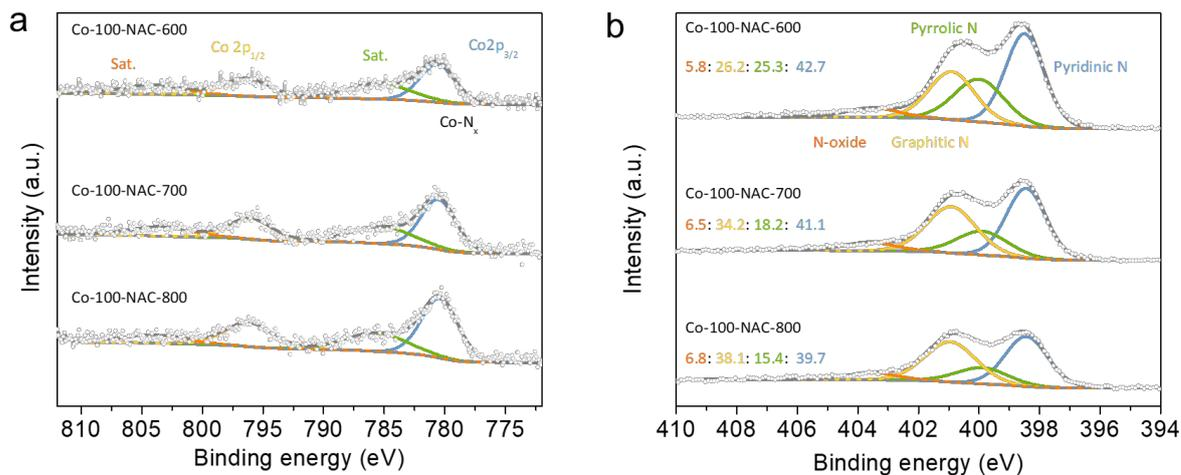
**Figure S7.** XPS of Co-NAC prepared at different temperatures. (a) Co<sub>2</sub>p Spectre and (b) N<sub>1</sub>s Spectre.
