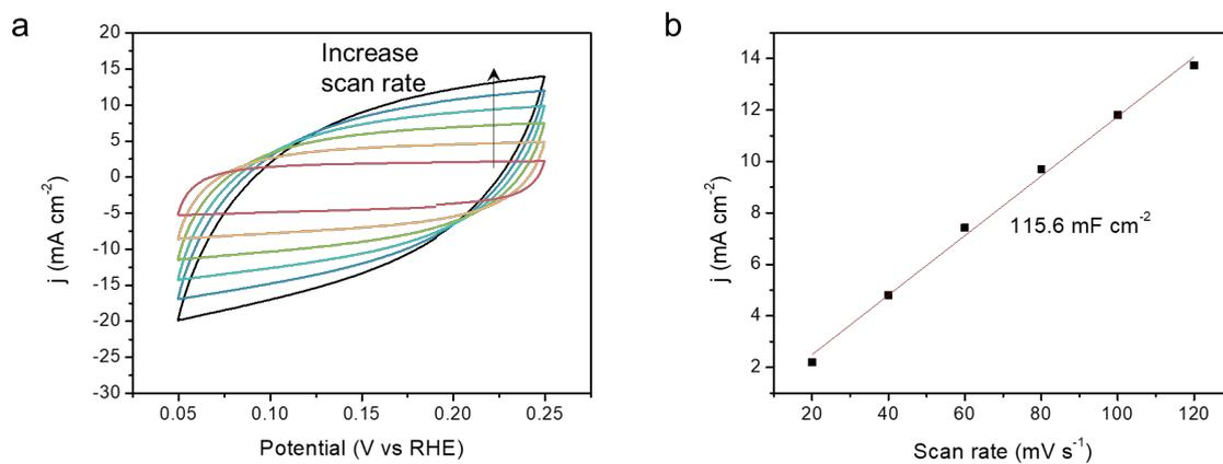
**Figure S13.** ECSA estimation of Co-100-NAC-700. (a) CV curve at potential range 0.05-0.25 V vs RHE; (b) linear relationship between current density and scan rate.
