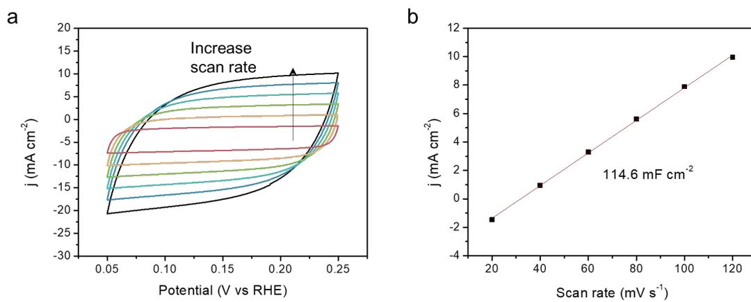
**Figure S10.** ECSA estimation of Co-50-NAC-800. (a) CV curve at potential range 0.05-0.25 V vs RHE; (b) linear relationship between current density and scan rate.
