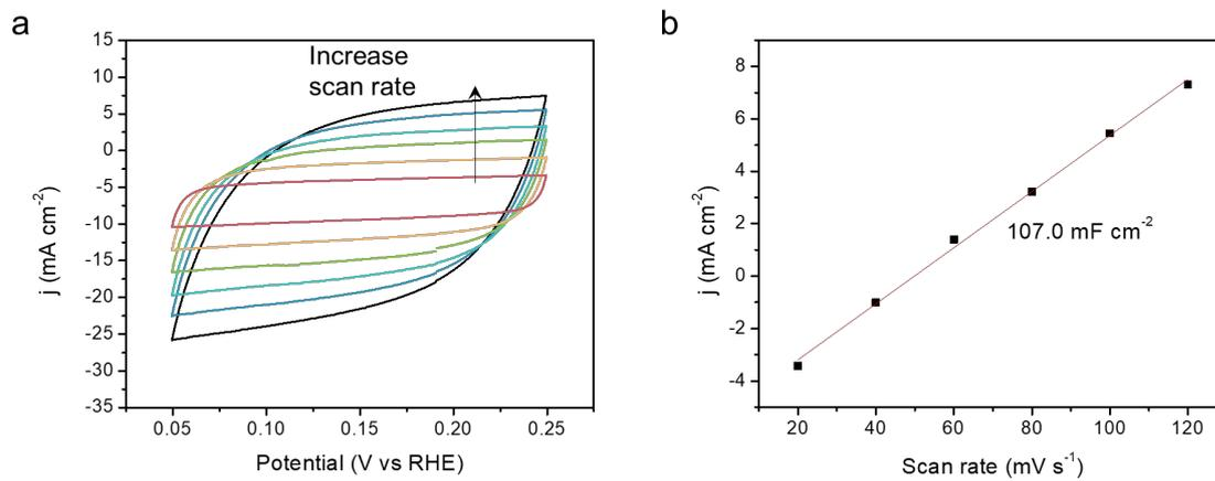
**Figure S9.** ECSA estimation of Co-25-NAC-800. (a) CV curve at potential range 0.05-0.25 V vs RHE; (b) linear relationship between current density and scan rate.
