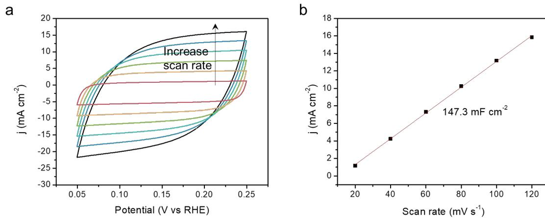
**Figure S11.** ECSA estimation of Co-100-NAC-800. (a) CV curve at potential range 0.05-0.25 V vs RHE; (b) linear relationship between current density and scan rate.
