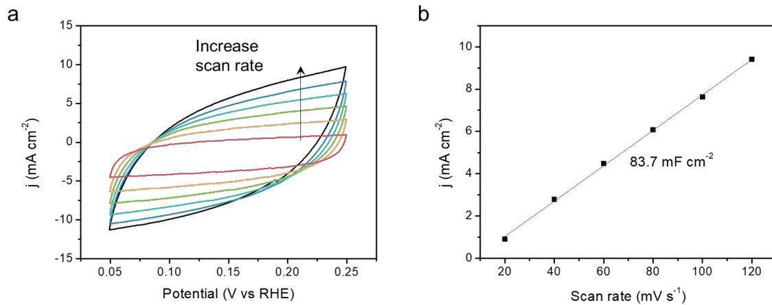
**Figure S12.** ECSA estimation of NAC-800. (a) CV curve at potential range 0.05-0.25 V vs RHE; (b) linear relationship between current density and scan rate.
