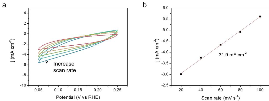
**Figure S14.** ECSA estimation of Co-100-NAC-600. (a) CV curve at potential range 0.05-0.25 V vs RHE; (b) linear relationship between current density and scan rate.
