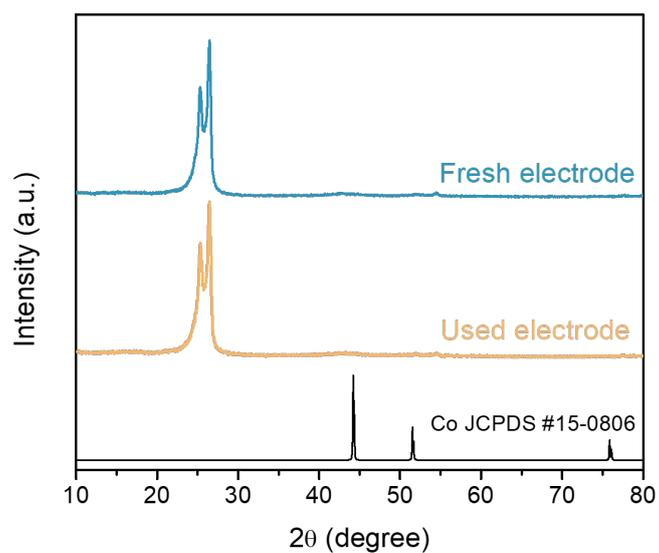
**Figure S16.** XRD characterization of the Co-100-NAC-800 electrode before and after HER test. Blue line: fresh Co-100-NAC-800 electrode; orange line: Co-100-NAC-800 after 20 h stability test. No diffraction pattern change or Co aggregation was observed.
