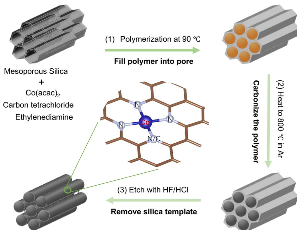
**Scheme S1.** Synthesis procedure for single-atom Co-NAC with aligned pore structure using mesoporous silica template.
