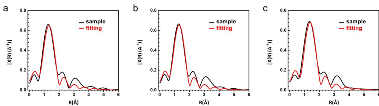
**Figure S6.** EXAFS spectra of (a) Co-100-NAC-800; (b) Co-100-NAC-700; (c) Co-100-NAC-600. The data of Co-NAC-800 had been published in our previous work and added here for comparison purposes.<sup>1</sup>
