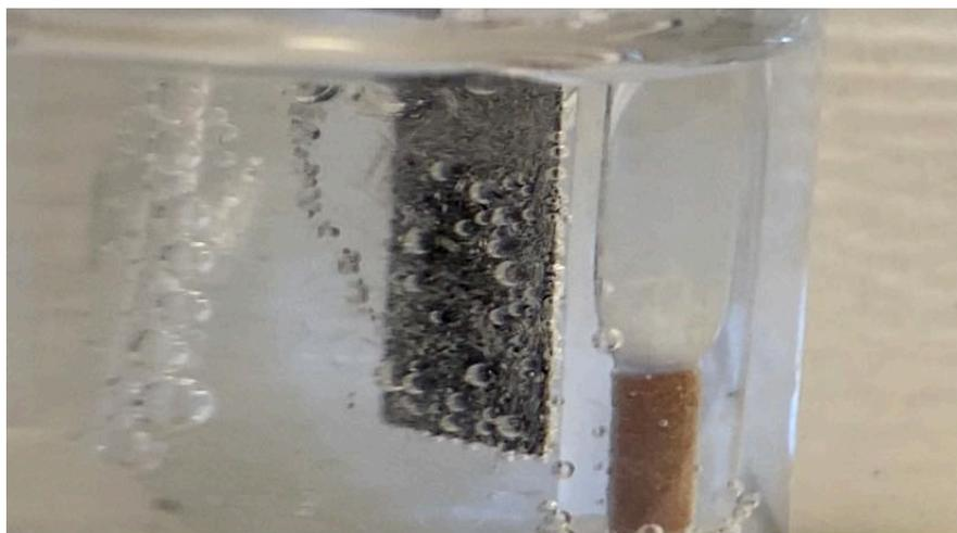
**Figure S15.** Photo showing hydrogen production during the stability test.
