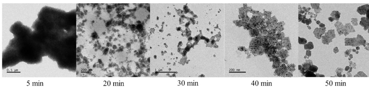
**Figure S7.** TEM images of aliquots collected during the formation of 2D-MNCs with 12nm iron oxide nanocubes at different time points, after: a) 5 min, b) 20 min, c) 30 min, d) 40 min and e) 50 minutes. The choice of 40 minutes was the selected one for better 2D MNC ordering.
