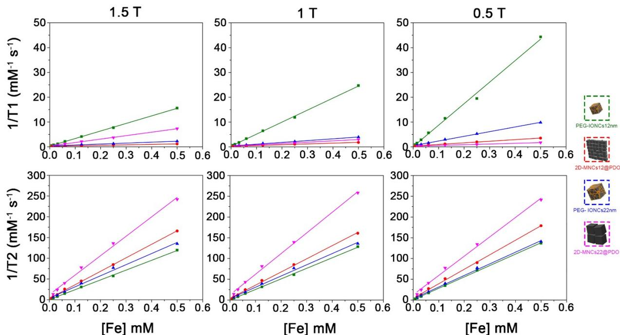
**Figure S13.**  $r_1$ ,  $r_2$  as a function of the applied magnetic field for PEG-IONCs12nm (green line), 2D-MNCs12@PDO (red line), PEG-IONCs22nm (blue line) and 2D-MNCs22@PDO (purple line). Data were fitted with linear fit and plotted as continuous lines.
