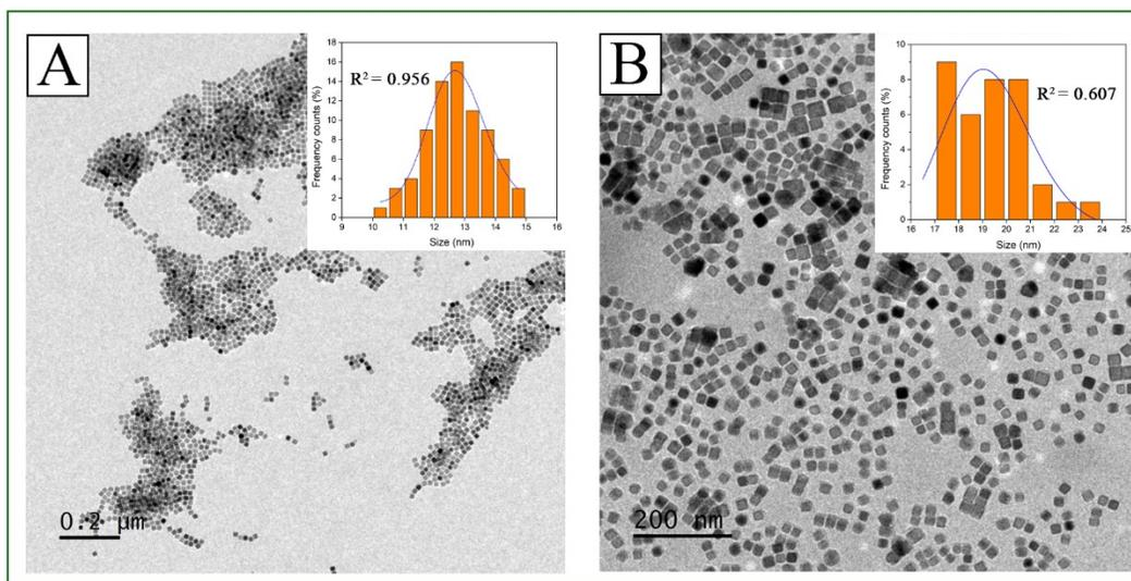
**Figure S1.** TEM images of IONCs with a corresponding diameter of A) PEG-IONCs 12nm and B) PEG-IONCs 22nm. In inset are reported the particle size distribution histograms observed in TEM images.
