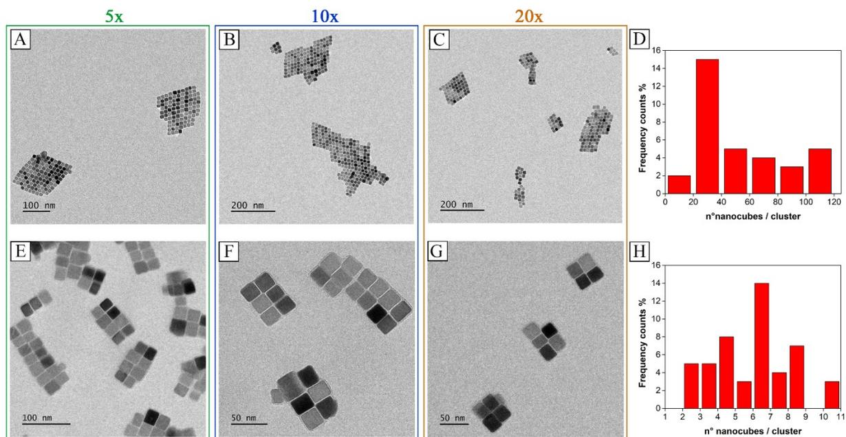
**Figure S8.** TEM images of 2D-MNCs12nm and 2D-MNCs22nm scaled up A and E) 5 fold; B and F) 10 fold , C) and G) 20 fold, respectively. Number of IONCs per clusters histograms of D) 2D-MNCs12@PDO and H) 2D-MNCs22@PDO observed in TEM images scaled up 20 fold.
