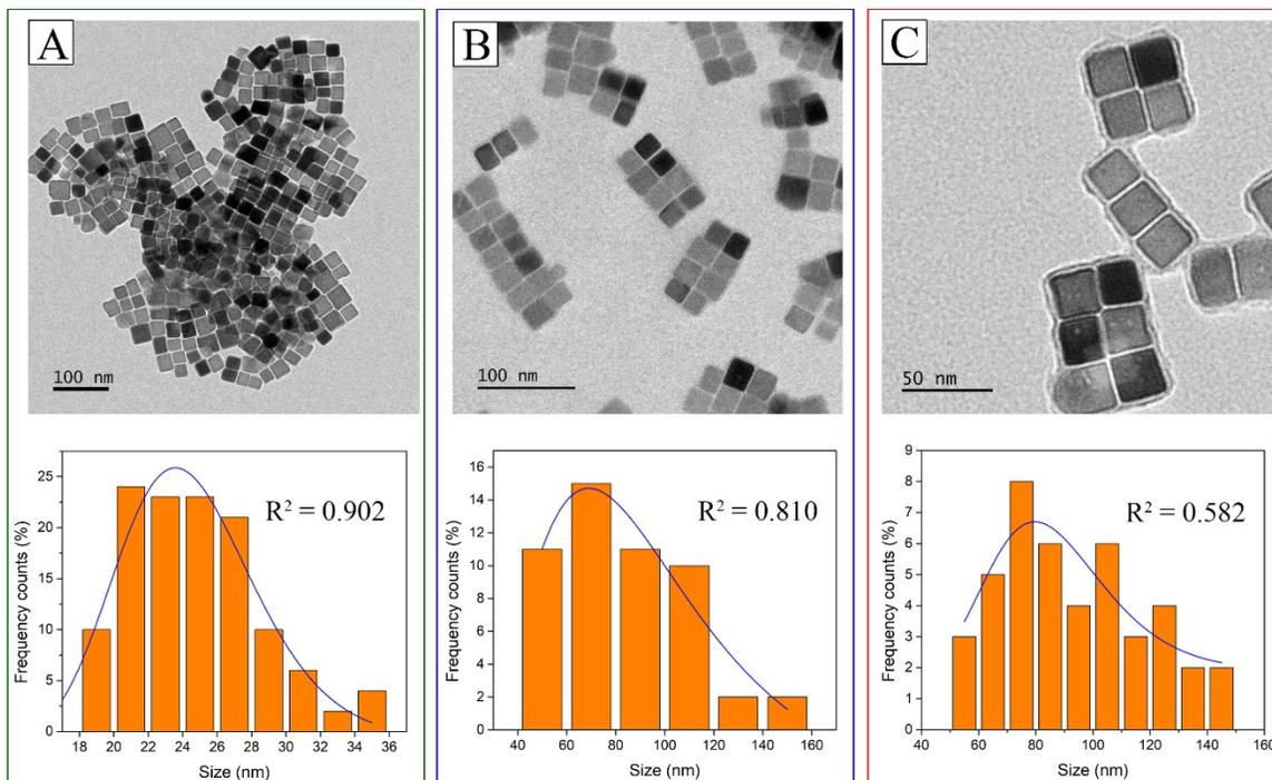
**Figure S11.** TEM images of A) IONCs24nm, B) 2D-MNCs24nm and C) 2D-MNCs24@PDO and their respective particle size distribution histograms as measured by statistics on TEM images.
