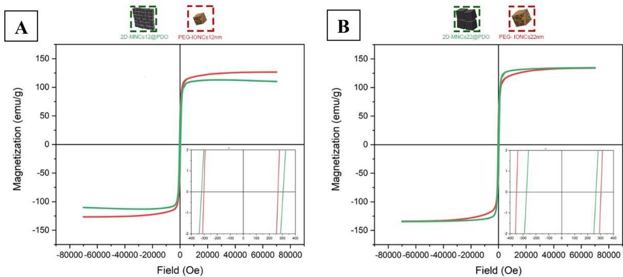
**Figure S12.** Normalized magnetization curves measured at 5K for A) PEG-IONCs12nm and 2D-MNCs12@PDO and B) PEG-IONCs22nm and 2D-MNCs22@PDO. The inset represents a detail of the low field region for each of the curves.
