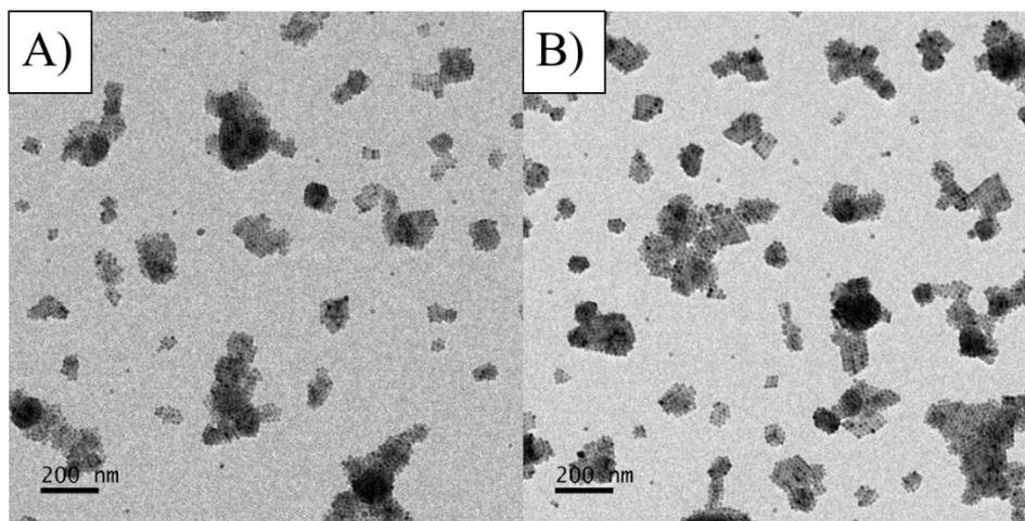
**Figure S6.** TEM images of MNCs obtained by setting the temperature of the water-bath sonicator at room temperature. Under these conditions 2D and 3D clusters are seen.
