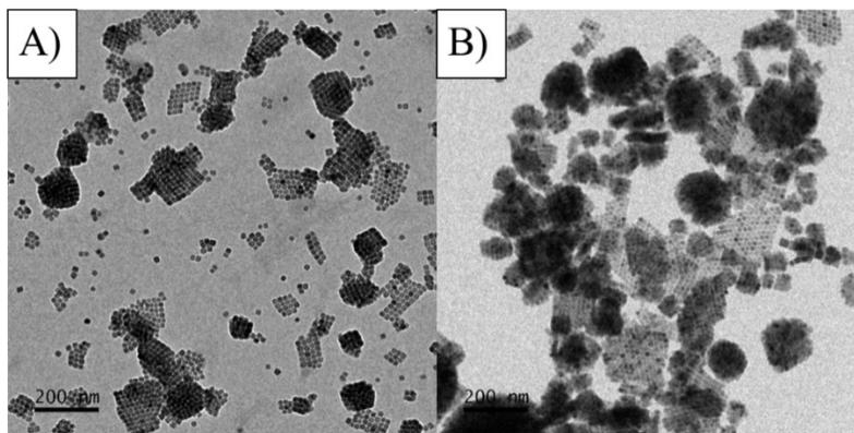
**Figure S5.** TEM images of: a) MNCs obtained by using SDS of 1.1 mg/mL and b) MNCs by using SDS of 2.6 mg/mL. 2D and 3D clusters arrangements are both evident in both samples.
