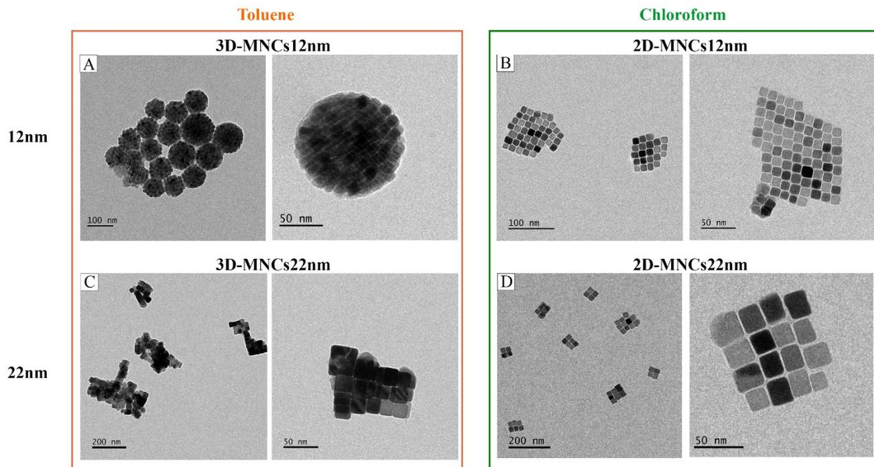
**Figure S3.** TEM images of: MNCs obtained by starting from IONCs12nm dispersed in A) toluene (3D-MNCs12nm) or in B) chloroform (2D-MNCs12nm), and corresponding clusters obtained by starting from IONCs22nm dispersed in C) toluene (3D-MNCs12nm) and D) chloroform (2D-MNCs12nm).
