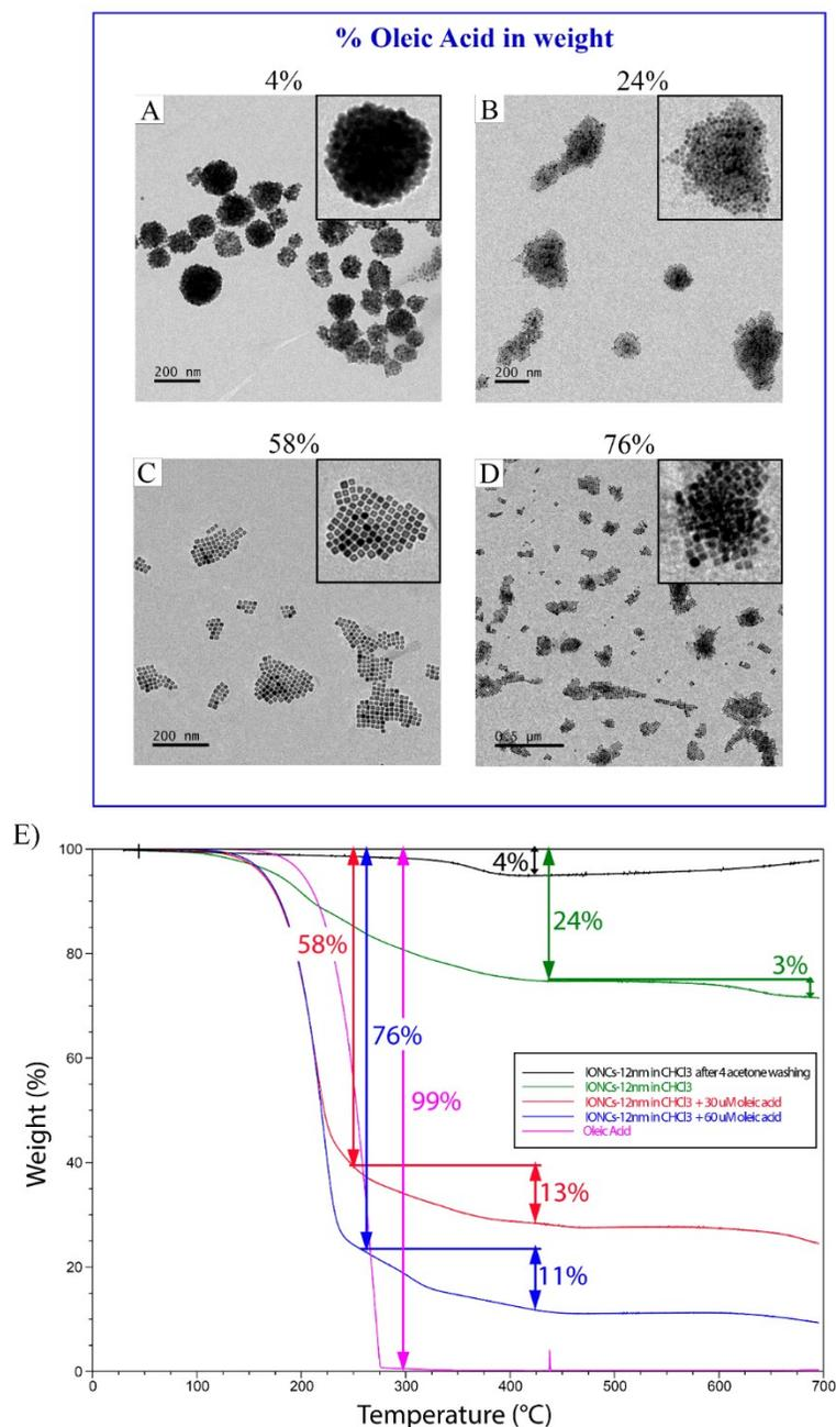
**Figure S4.** TEM images of MNCs12nm obtained using IONCs12nm: A) after four acetone washing to remove the oleic acid (4% in weight) and after the addition of oleic acid in the solution reaching three different percentage in weight, B) 24% C) 58% and D) 76%. E) TGA analysis of IONCs-12nm (green spectra) obtained after by adding different oleic acid concentration: 30  $\mu$ M
