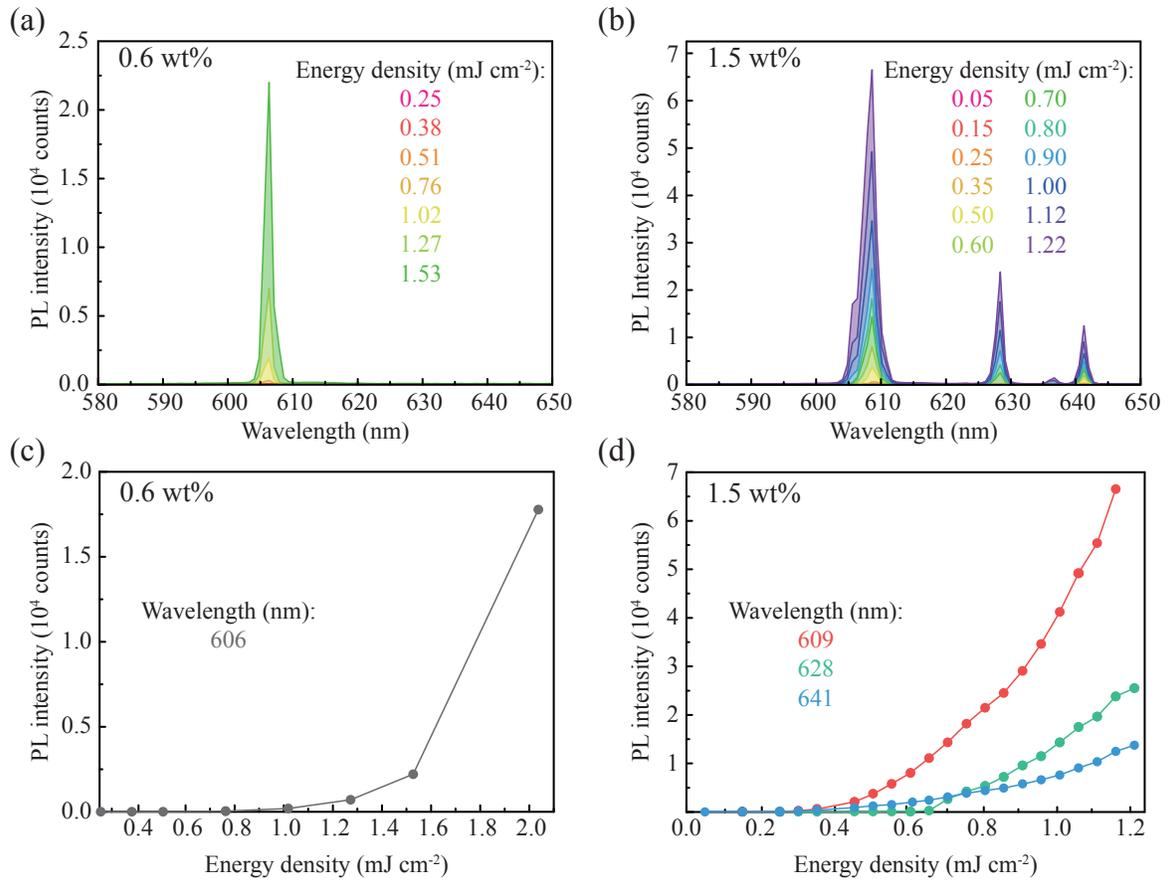
Figure S6: (a,b) PL spectra for the  $\Lambda = 400$  nm array with a layer of Rhodamine B-doped SU-8 at dye concentrations of 0.6 wt% (a) and 1.5 wt% (b), measured for increasing excitation energy densities. (c,d) PL intensity at each mode peak wavelength as a function of the energy density, showing the lasing threshold for the samples in (a,b).
