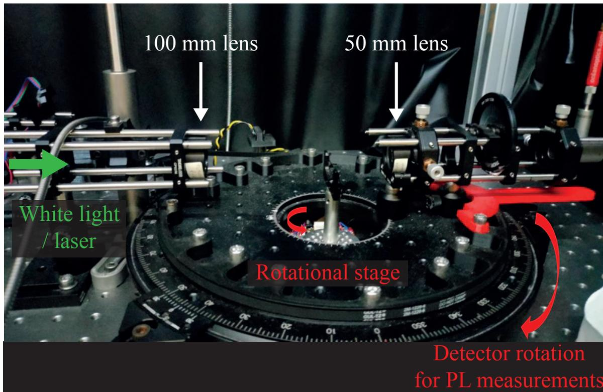
Figure S7: Photograph of the setup used for the angular-resolved transmittance and PL measurements. The sample is mounted on a rotatory stage adjusted to measure the transmittance. The position of the detector can also be adjusted, allowing for the measurement of the angle-resolved PL and the divergence of the lasing emission.
