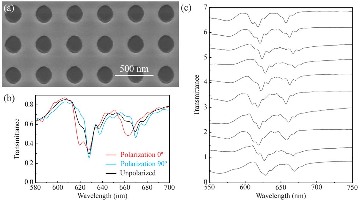
Figure S4: (a) SEM micrograph showing the asymmetric deposition of  $\text{TiO}_2$  inside the holes of the array with  $\Lambda = 400$  nm. (b) Transmittance measured at normal incidence using light with different polarization characteristics. (c) Change in the transmittance spectrum when scanning the illumination spot across the system.
