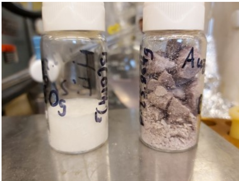
Figure S100: Triphenyl borate from the toluene process (left) and xylene process a couple weeks after it was made (right).
