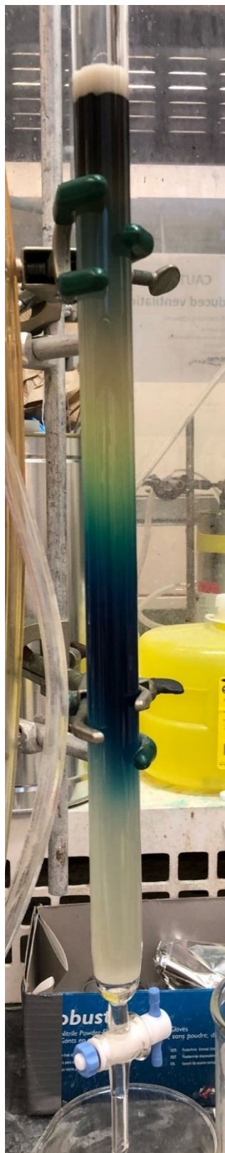
Figure S83: Column chromatography of PhO-BsubNc reaction crude.
