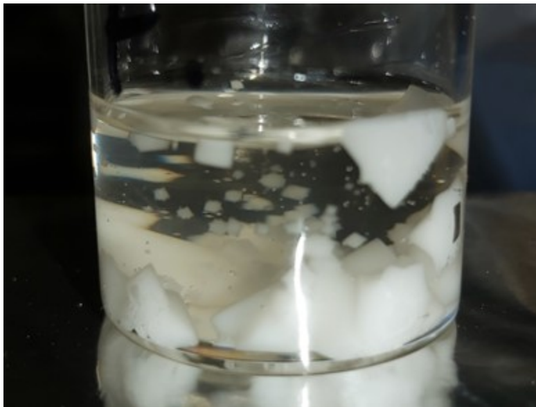
Figure S99: Crystallization of \text{B(OPh)}_3 from the toluene process.
