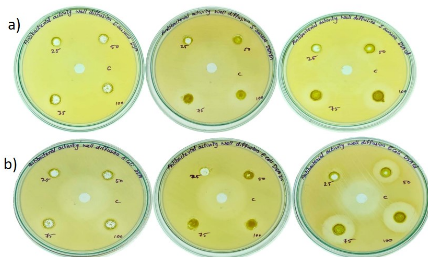
Figure S13. Zone of inhibition of (a) S.aureus (b) E.coli against ligand, complex 1 and complex 2.
