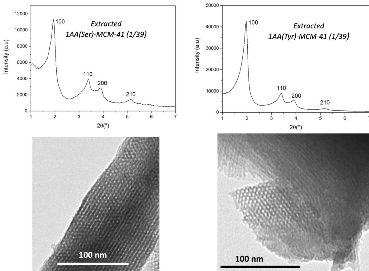
**Fig. S4** XRD patterns and TEM of extracted AA-functionalized MCM-41 with (left) 1 AA (Ser) and (right) 1 AA (Tyr) for the molar ratio organosilane/SiO<sub>2</sub> = 1/39.
