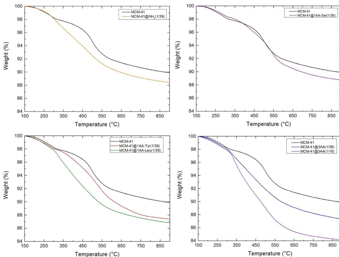
**Fig. S6** Normalized ATG curves of surfactant extracted MCM-41 and organo-functionalized MCM-41 materials with aminopropyl ( $\text{NH}_2$ ) or AA groups (1 AA or a mixture of 3 AA in ratio 1/3, 1/3, 1/3) for molar ratio organosilane/ $\text{SiO}_2 = 1/19$  or 1/39.
