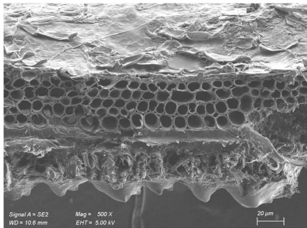
**Fig. S2 SEM images of RH washed with water and treated with HCl.**
