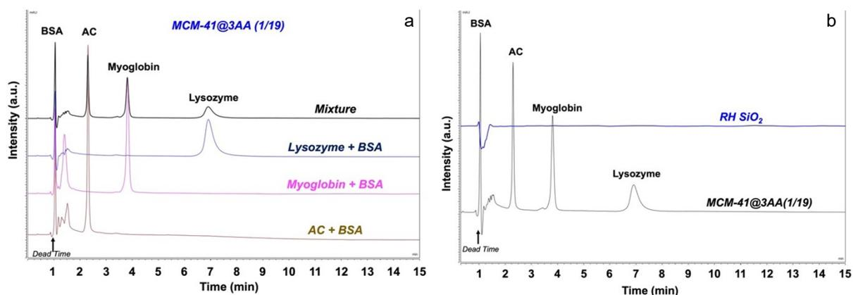
**Fig. S9** Comparison of proteins separations with MCM-41@3AA(1/19) (a) for the mixture of the four proteins and for each protein mixed with BSA and (b) with a column filled with silica from RH for the mixture of the four proteins. Conditions: particles 50-100  $\mu\text{m}$ , mobile phase H<sub>2</sub>O/ACN 98/2 (v/v), flow rate 1 mL min<sup>-1</sup>.
