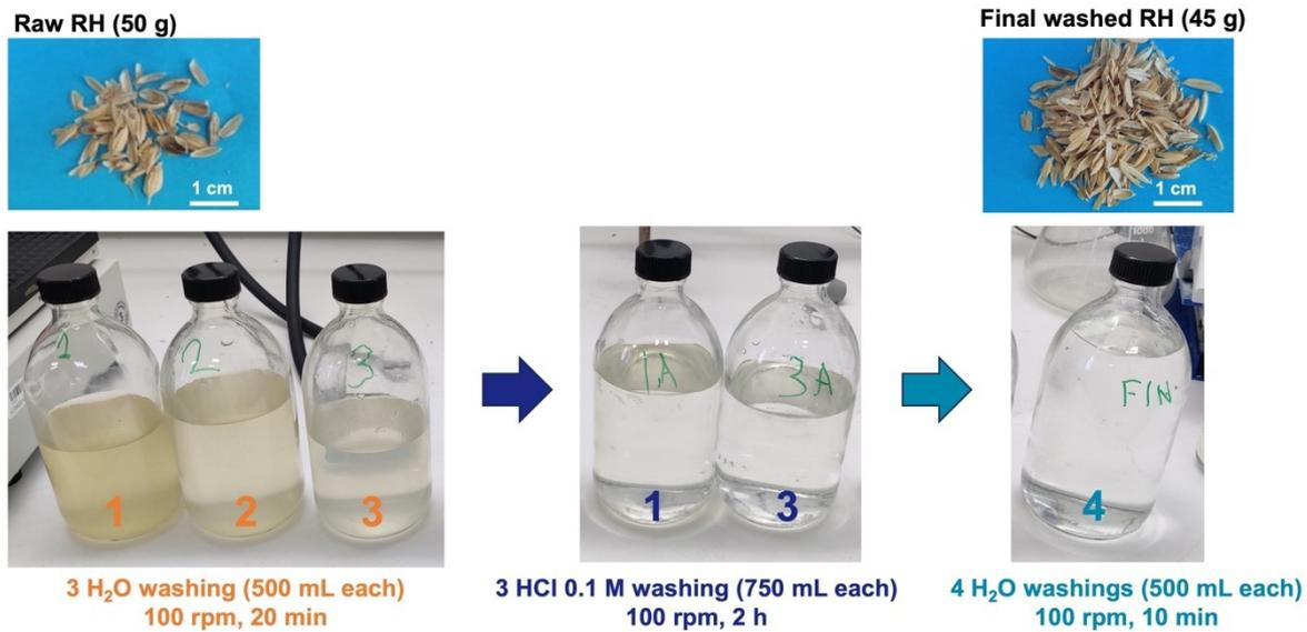
**Fig. S1** Pictures of raw and final washed RH and of the supernatant solutions after the different washings: first three H<sub>2</sub>O washings, first and third HCl 0.1 mol L<sup>-1</sup> washings at 25 °C, final H<sub>2</sub>O washing (4<sup>th</sup> H<sub>2</sub>O washing).
