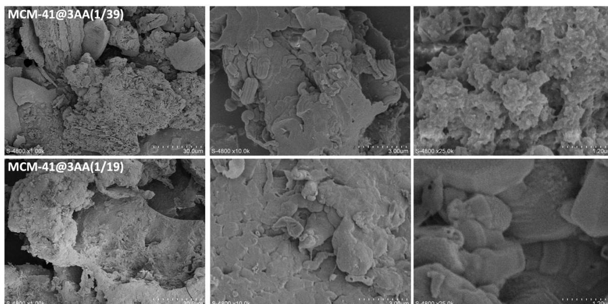
**Fig. S7** SEM images of extracted AA-functionalized MCM-41 prepared with the mixtures of 3 AA (Leu, Ser, Tyr).
