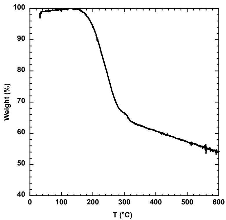
**Fig. S5** TGA curve of as-synthesized MCM-41 obtained by pseudomorphic transformation of silica from RH.
