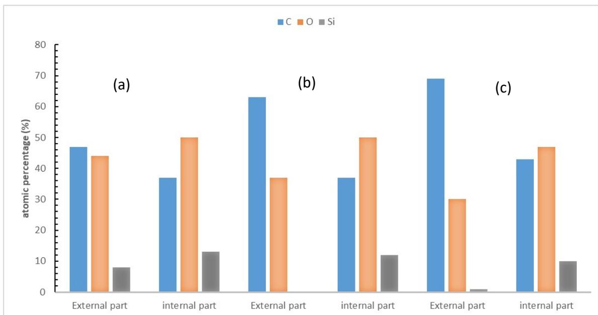
**Fig. S3** EDS analysis (atomic percentage) of the internal and external parts of (a) raw rice husk, (b) rice husk washed with water and (b) HCl treated rice husk (HCl 0.1 mol L<sup>-1</sup>, shaking) followed by water washing. Carbon content should not be taken into account as carbon stick was used to maintain particles on EDS supports.
