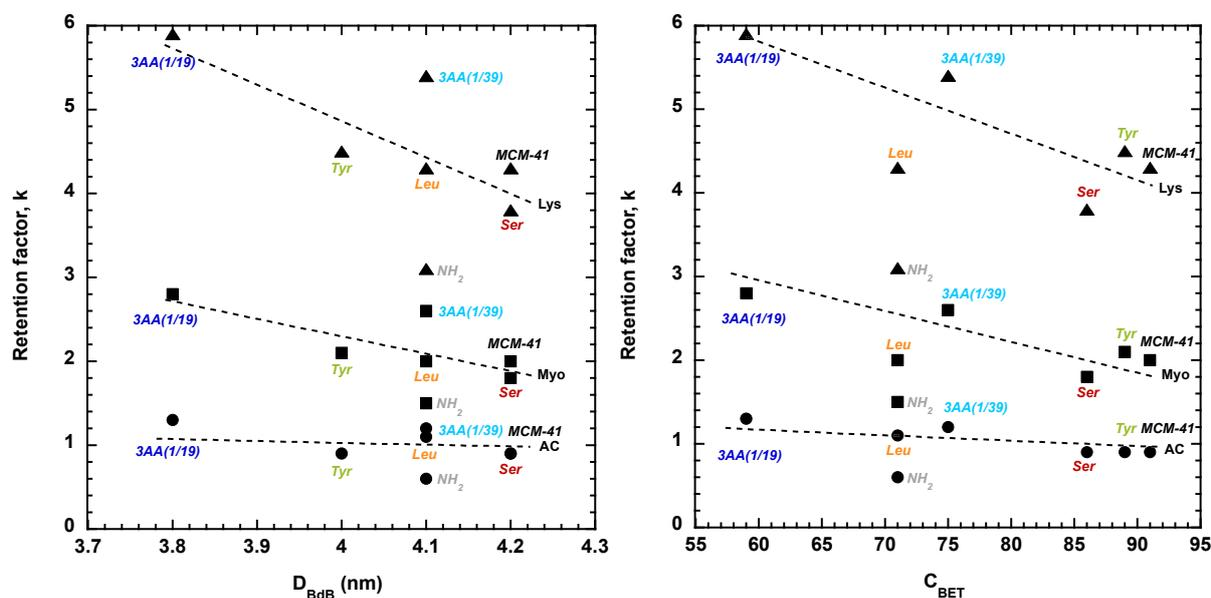
**Fig. S8** Retention factors of proteins (circle) Carbonic Anhydrase (AC), (square) Myoglobin, (triangle) Lysozyme, as a function of (left) material mesopore diameter ( $D_{BdB}$ ) and (right) material surface hydrophobicity ( $C_{BET}$ ).
