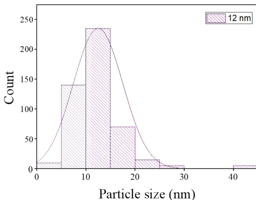
**Figure 1S:** Size distribution curve for g-C<sub>3</sub>N<sub>4</sub>@ZnHCC nanoparticles (using imageJ software)
