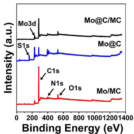
**Fig. S8** XPS survey scan of Mo@C/MC, Mo@C and Mo/MC catalysts.
