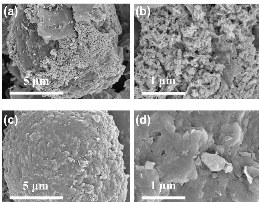
**Fig. S4** SEM image of Mo@C/MC catalyst (a, b) and Mo/MC catalyst (c,d).
