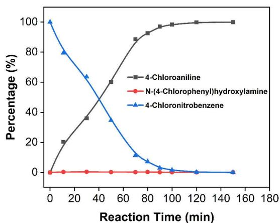
**Fig. S19** The yields of *p*-CNB and *p*-CAN upon Mo@C/MC catalyst. Reaction conditions: 0.25 mmol *p*-CNB in 5 mL ethanol/H<sub>2</sub>O (V/V = 1: 4) with 50 mg catalyst reacted at 100 °C, 5 bar H<sub>2</sub> for 3 h. The identity of the products was further determined by HPLC.
