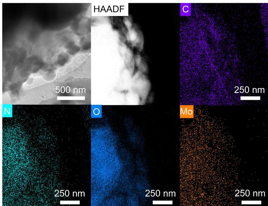
**Fig. S16** TEM and mapping profiles of the Mo@C/AC catalyst
