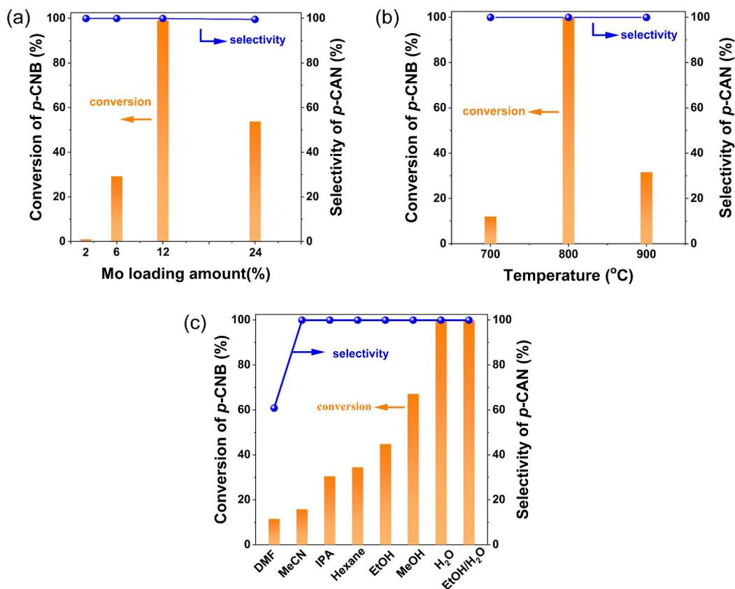
**Fig. S10** Impact of Mo amount (a), calcination temperature (b) and solvent (c) on the hydrogenation of *p*-CNB. Reaction conditions: 0.25 mmol *p*-CNB in 5 mL ethanol/H<sub>2</sub>O (V/V = 1:4) with 50 mg catalyst reacted at 100 °C, 5 bar H<sub>2</sub> for 3 h. The identity of the products was further determined by HPLC.
