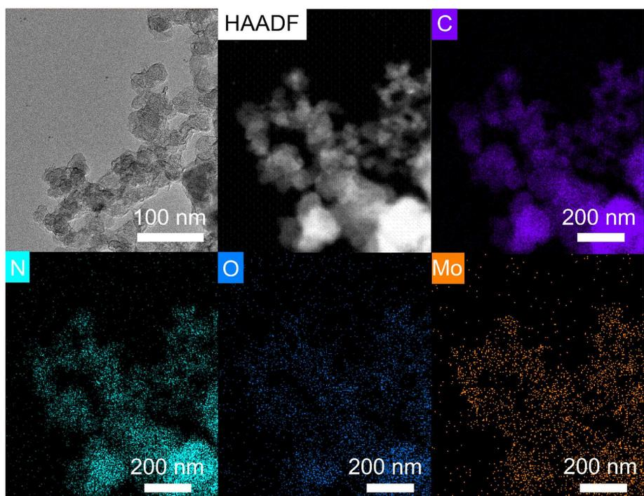
**Fig. S14** TEM and mapping profiles of the Mo@C/PC catalyst
