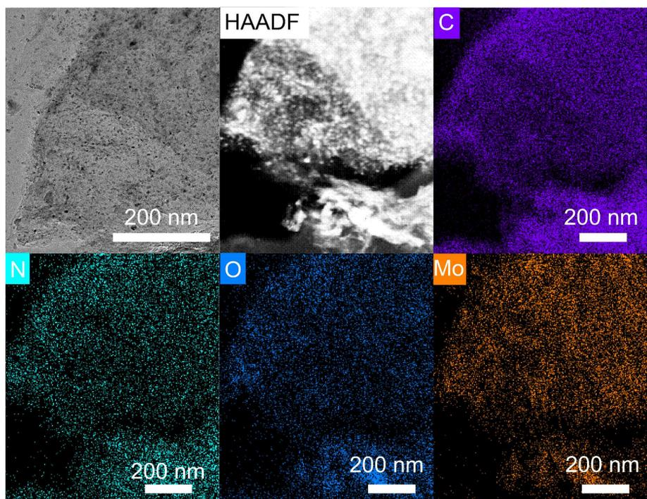
**Fig. S15** TEM and mapping profiles of the Mo@C/GO catalyst
