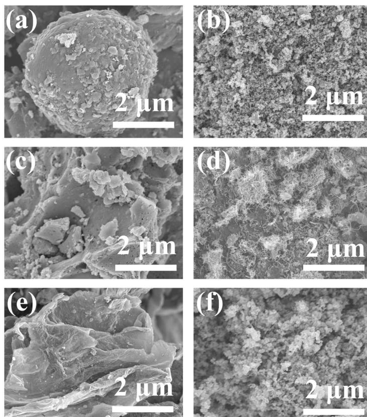
**Fig. S12** SEM image of Mo@C/MC (a), Mo@C/VC (b), Mo@C/AC (c), Mo@C/CNTs (d), Mo@C/GO (e), Mo@C/PC (f) catalyst.
