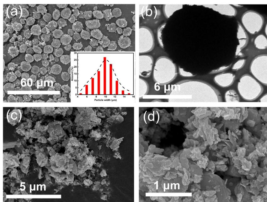
**Fig. S2** SEM image and particle width distribution of commercial microsphere carbon support (a). TEM image of Mo@C/MC catalyst (b). SEM images of Mo@C catalysts(c,d).
