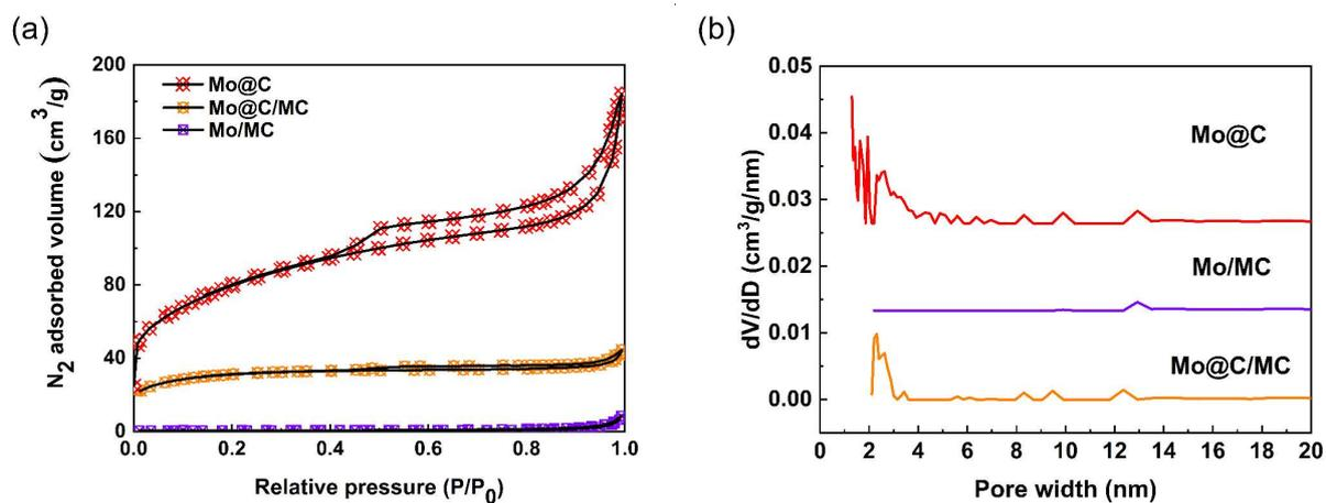
**Fig. S7** Nitrogen adsorption and desorption isotherms (a) and pore size distribution (b) of three catalysts.
