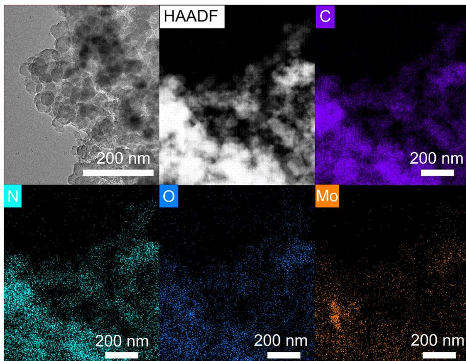
**Fig. S17** TEM and mapping profiles of the Mo@C/VC catalyst
