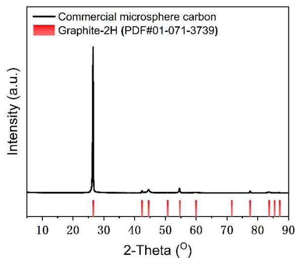
**Fig. S1** XRD pattern of the pure commercial microsphere carbon (MC) support.
