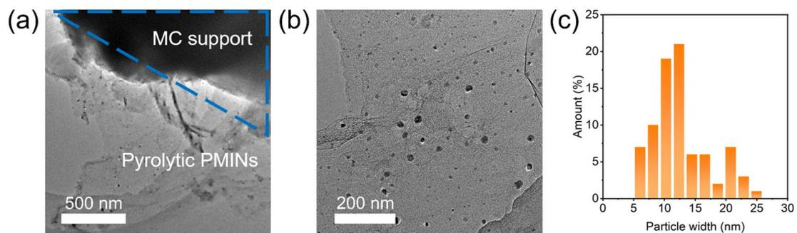
**Fig. S3** TEM images of the edge of Mo@C/MC catalyst (a, b) and particle width distribution of Mo@C/MC catalysts (c).
