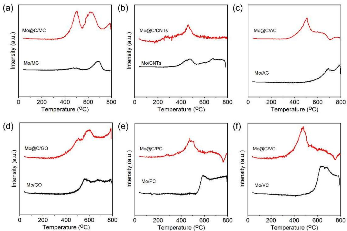
**Fig. S18** H<sub>2</sub>-TPR profiles of the catalysts containing different carbon matrices
