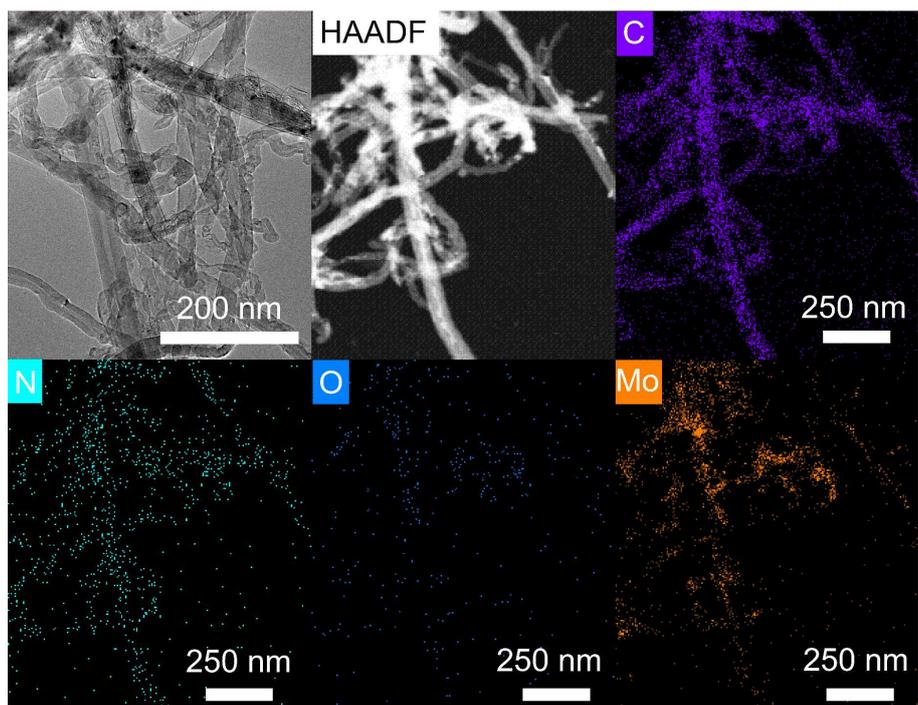
**Fig. S13** TEM and mapping profiles of the Mo@C/CNTs catalyst.
