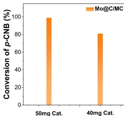
**Fig. S20** Catalyst usage on Mo@C /MC. Reaction conditions: 0.25 mmol *p*-CNB in 5 mL ethanol/H<sub>2</sub>O (V/V = 1:4) with catalyst reacted at 100 °C, 5 bar H<sub>2</sub> for 3 h. The identity of the products was further determined by HPLC.
