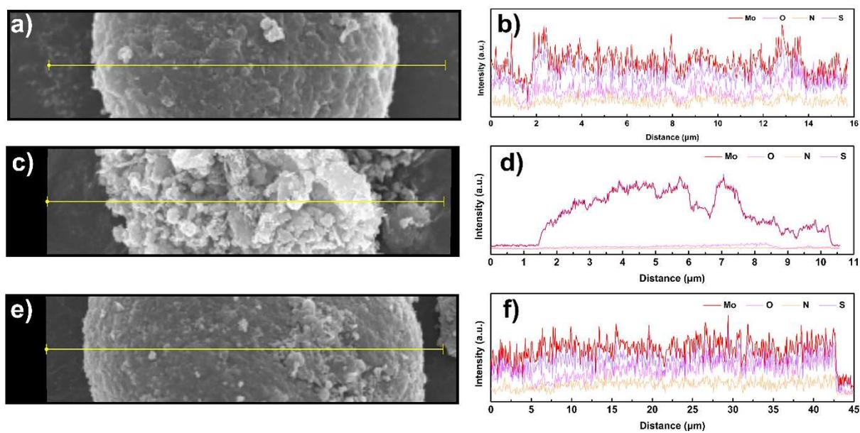
Fig. S6 Line scan EDS image of Mo@C/MC (a, b), Mo@C (c, d) and Mo/MC (e, f) catalysts.
