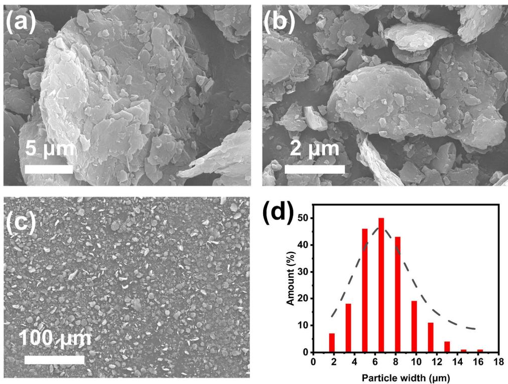
**Fig. S9** SEM images of Mo@C/MC catalyst after ball milling (a, b and c) and its particle width distribution (d).
