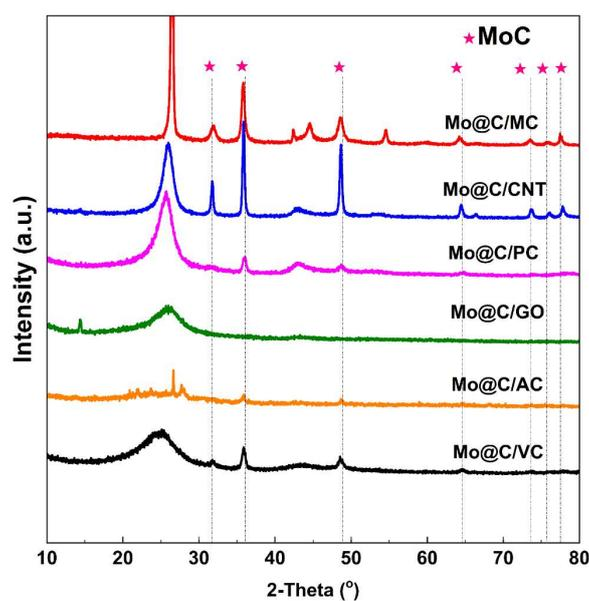
**Fig. S11** XRD pattern of different types of protein-coated carbon matrices (including carbon
