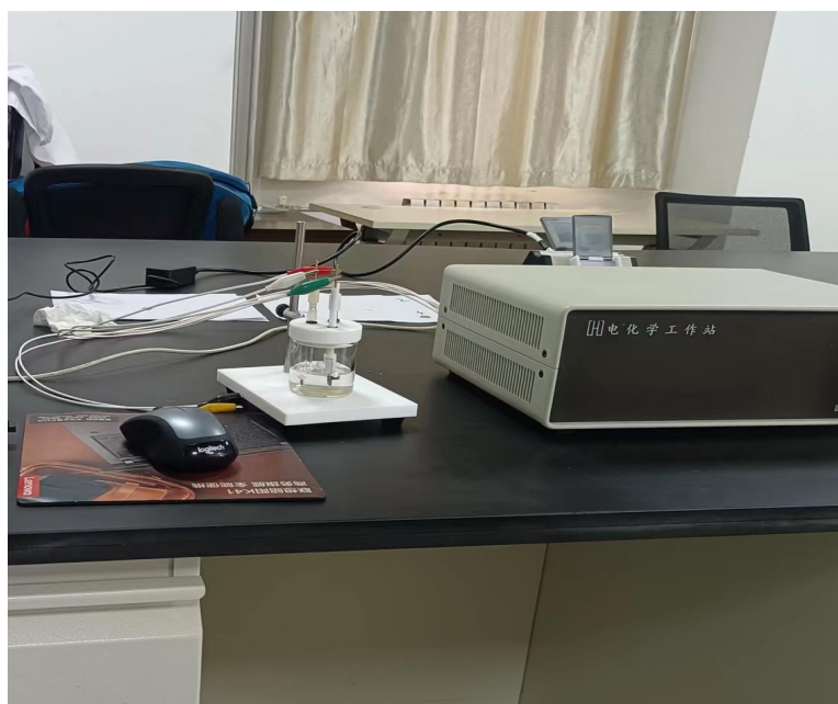
Fig. S2 A photograph showing electrocatalytic test on the CuCo 2 O 4 /NF electrodes.
