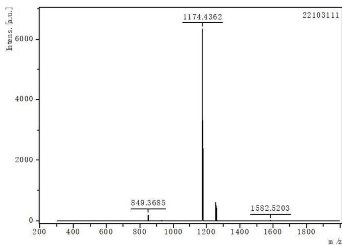
Figure S5 MALDI-TOF HRMS spectrum of (TPA)<sub>2</sub>DPP (calcd for C<sub>74</sub>H<sub>70</sub>N<sub>4</sub>O<sub>2</sub>S<sub>4</sub>:1174.4376)
