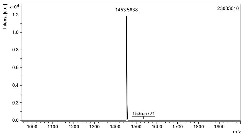
Figure S17 MALDI-TOF HRMS spectrum of  $(\text{DPP})_2\text{TPA}$  (calcd for  $\text{C}_{86}\text{H}_{95}\text{N}_5\text{O}_4\text{S}_6$ :1453.5703)
