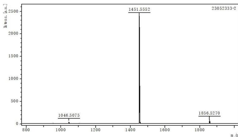
Figure S20 MALDI-TOF HRMS spectrum of  $(\text{DPP})_2\text{PCZ}$  (calcd for  $\text{C}_{86}\text{H}_{93}\text{N}_5\text{O}_4\text{S}_6$ :1451.5546)
