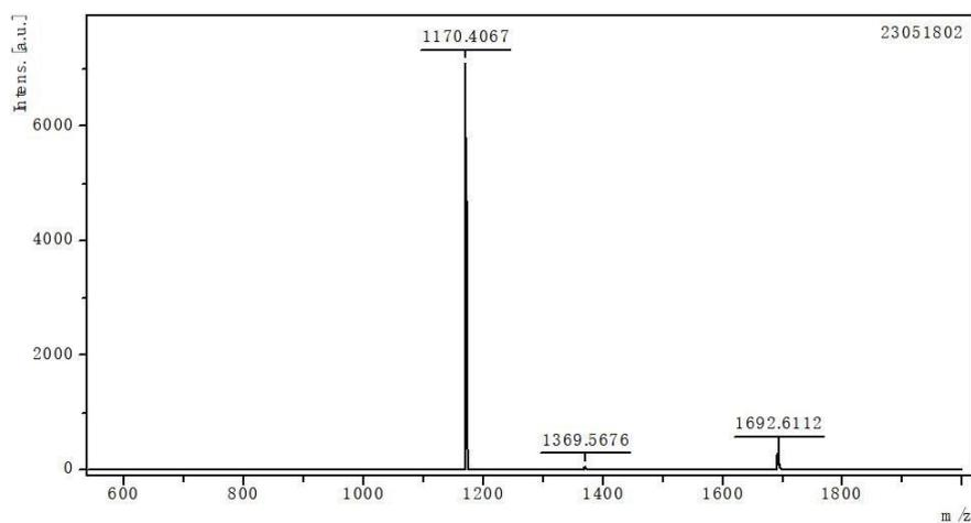
Figure S8 MALDI-TOF HRMS spectrum of  $(\text{PCZ})_2\text{DPP}$  (calcd for  $\text{C}_{74}\text{H}_{66}\text{N}_4\text{O}_2\text{S}_4$ :1170.4063)
