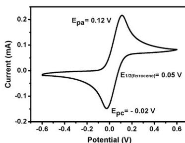
Figure S22 The CV curve of  $\text{Fc}/\text{Fc}^+$  in 0.1 M  $\text{Bu}_4\text{NBF}_4/\text{CH}_2\text{Cl}_2$  solution at a scan rate of  $100 \text{ mV s}^{-1}$  under nitrogen.
