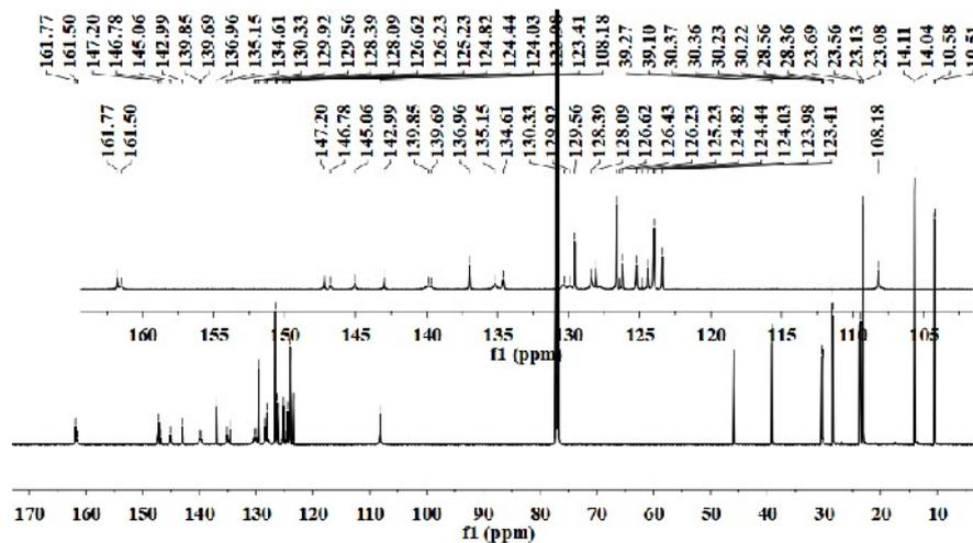
Figure S18  $^{13}\text{C}$  NMR spectrum of  $(\text{DPP})_2\text{TPA}$
