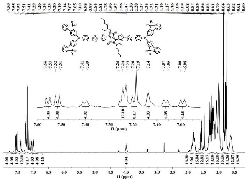
Figure S13  $^1\text{H}$  NMR spectrum of compound  $(\text{FPA})_2\text{DPP}$
