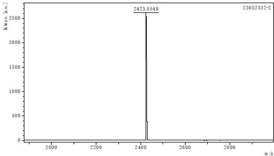
Figure S14 MALDI-TOF HRMS spectrum of  $(\text{FPA})_2\text{DPP}$  (calcd for  $\text{C}_{166}\text{H}_{214}\text{N}_4\text{O}_2\text{S}_4$ : 2423.5650)
