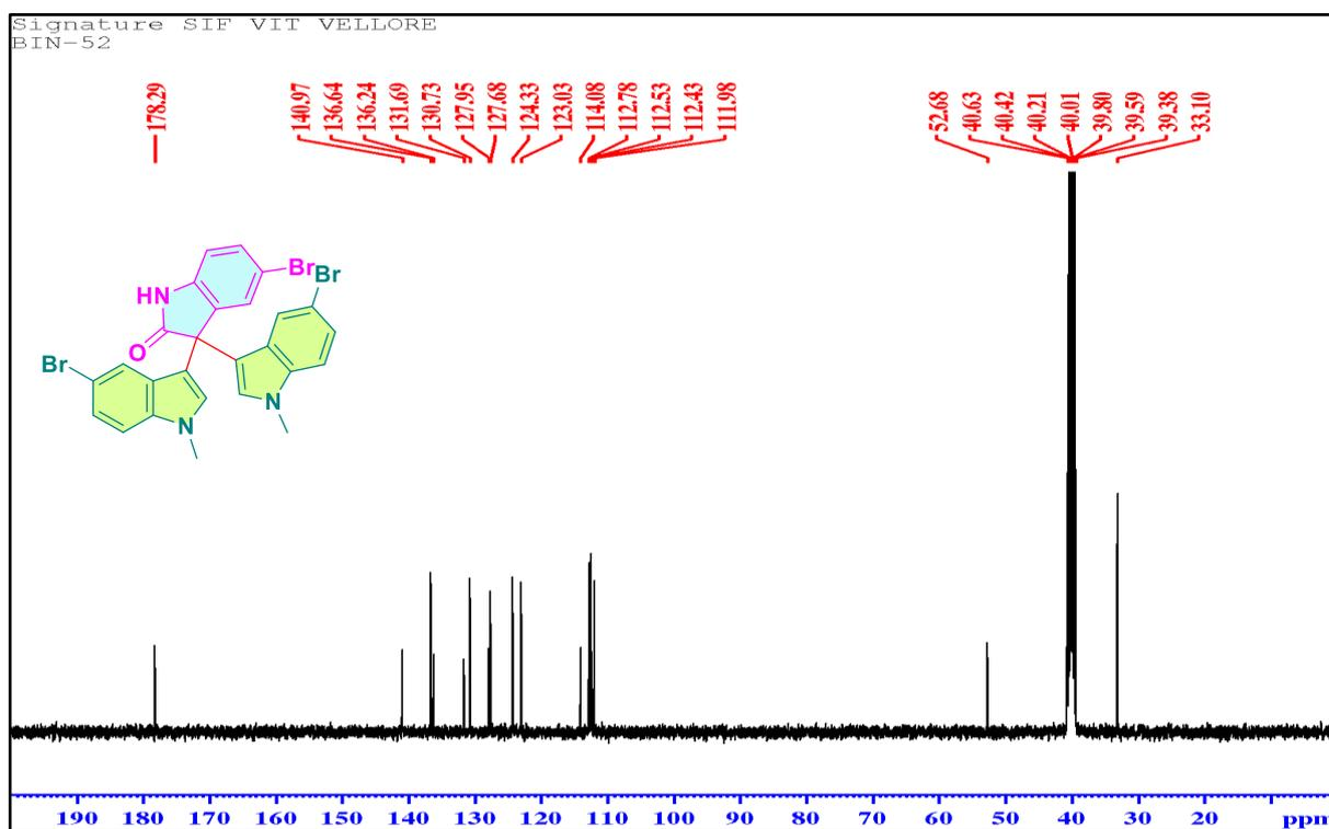
Fig. S65  $^{13}\text{C NMR}$  spectrum (100 MHz) of 7gd in DMSO- $d_6$ .
