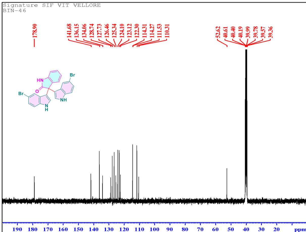
Fig. S39  $^{13}\text{C}$  NMR spectrum (100 MHz) of 7ea in DMSO- $\text{d}_6$ .
