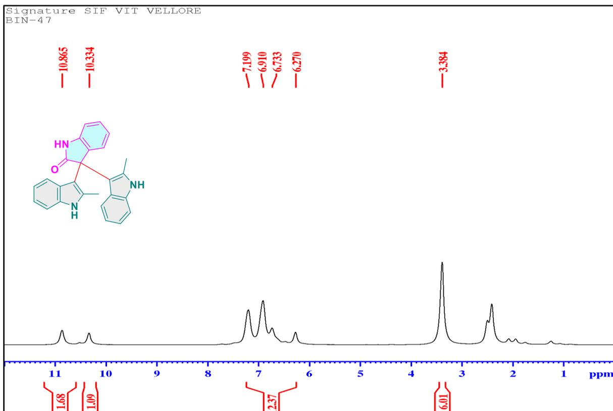
**Fig. S35**  $^1\text{H}$  NMR spectrum (400 MHz) of **7da** in  $\text{DMSO-d}_6$ .
