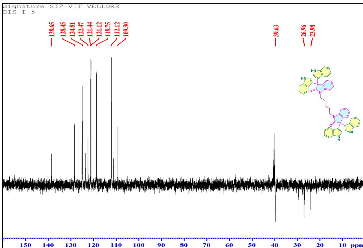
Fig. S113 DEPT-135 NMR spectrum (400 MHz) of **10ac** in DMSO- $d_6$
