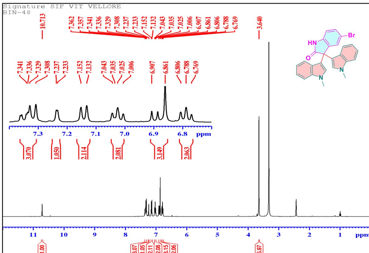
Fig. S53  $^1\text{H}$  NMR spectrum (400 MHz) of **7fd** in  $\text{DMSO-d}_6$ .
