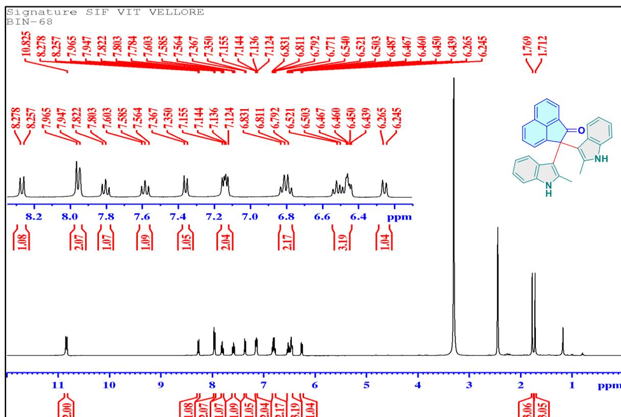
Fig. S82  $^1\text{H}$  NMR spectrum (400 MHz) of 7dj in  $\text{DMSO-d}_6$ .
