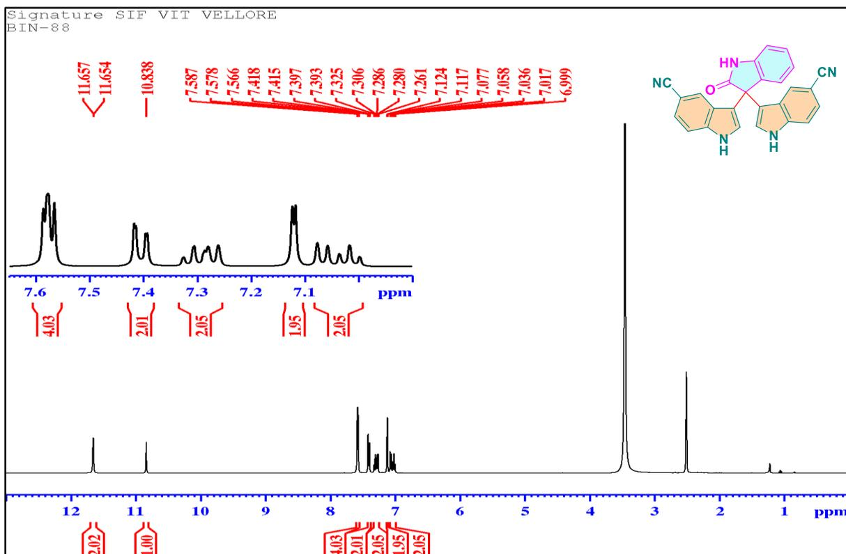
Fig. S29  $^1\text{H}$  NMR spectrum (400 MHz) of **7ba** in DMSO- $d_6$ .
