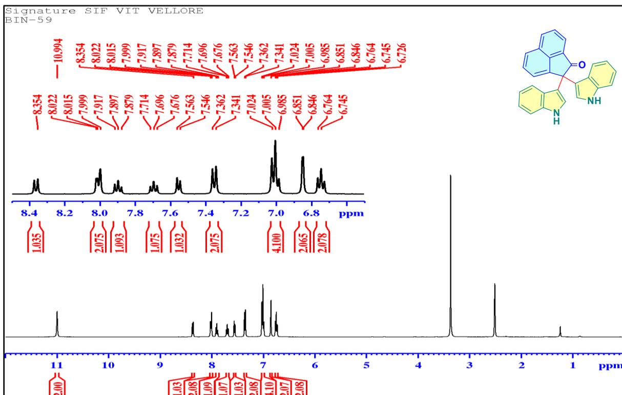
Fig. S76  $^1\text{H}$  NMR spectrum (400 MHz) of 7aj in DMSO- $d_6$ .
