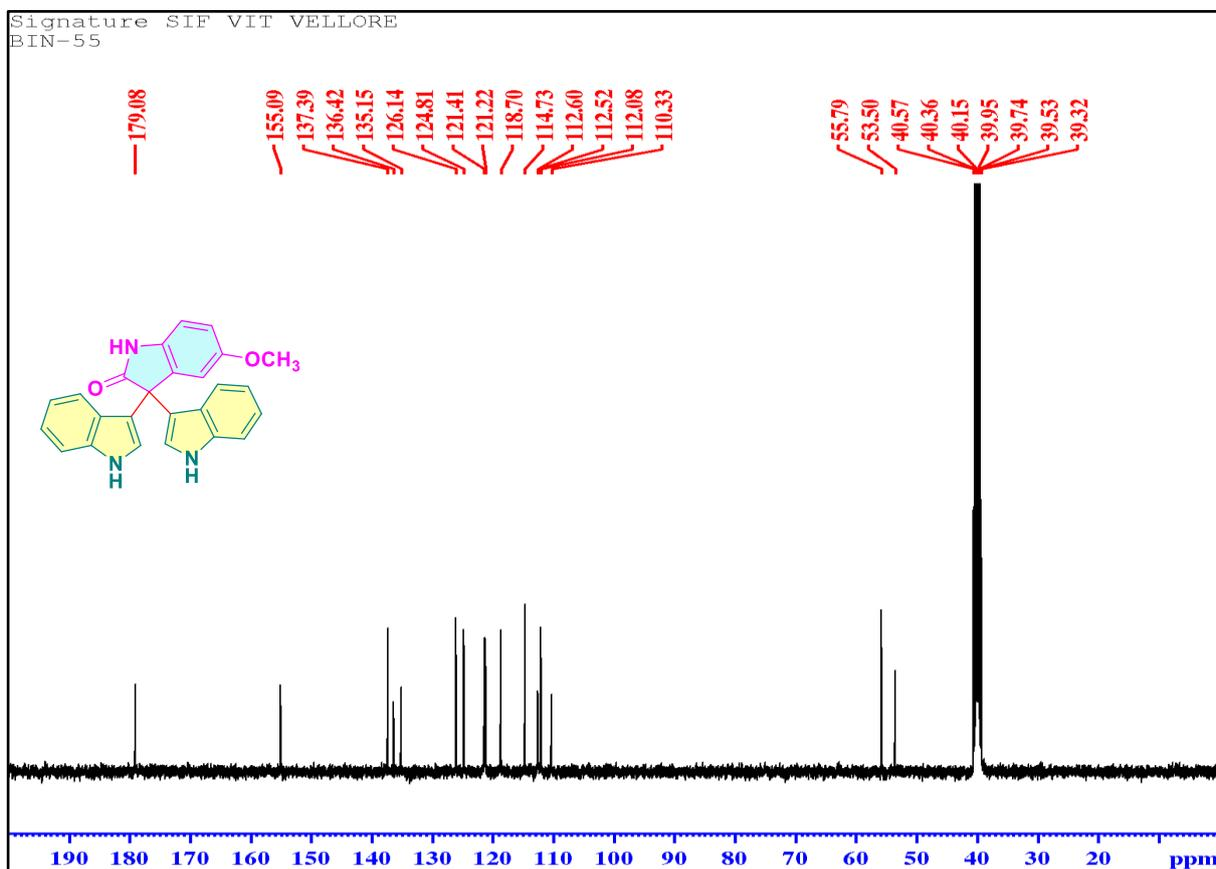
Fig. S24  $^{13}\text{C}$  NMR spectrum (100 MHz) of **7ag** in  $\text{DMSO-d}_6$ .
