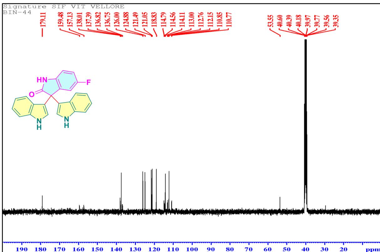
Fig. S12  $^{13}\text{C}$  NMR spectrum (100 MHz) of 7ac in DMSO- $d_6$ .
