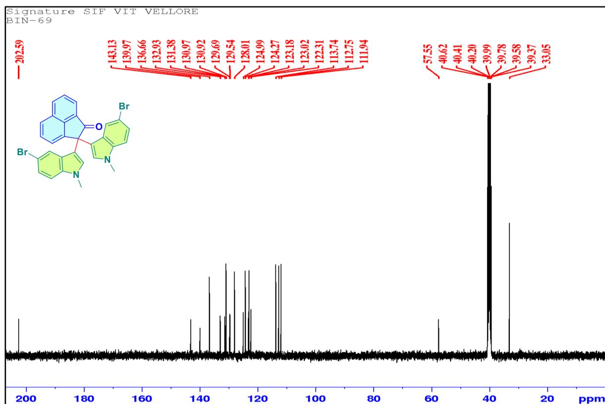
Fig. S92  $^{13}\text{C}$  NMR spectrum (100 MHz) of **7gj** in  $\text{DMSO-d}_6$ .
