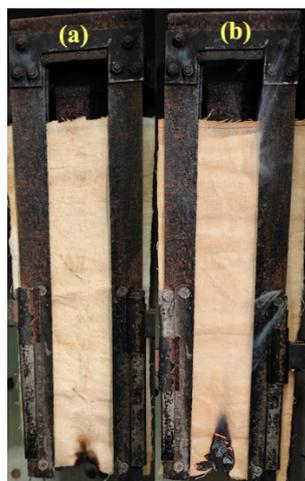
Figure S5: Photos of vertically flammability test: (a) P-CBPS-C (b) Washing fastness after 3<sup>rd</sup> washed (P-CBPS-C)
