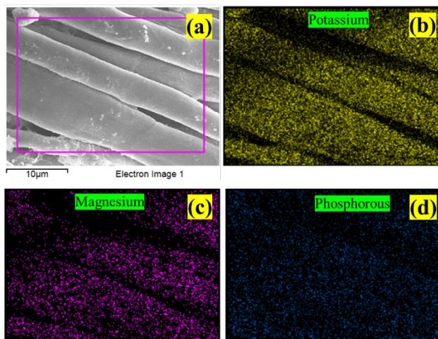
**Figure S3:** EDX elemental mapping of the BPS-C
