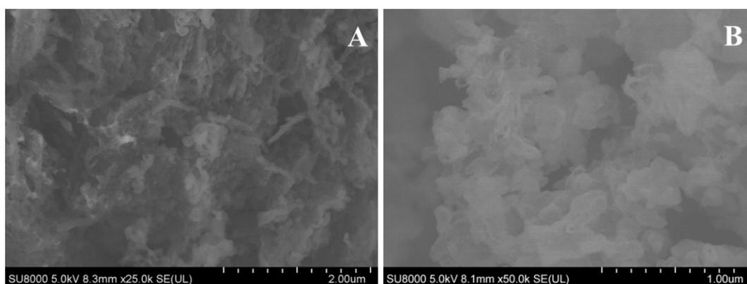
**Figure S1.** SEM images of bulk g-C<sub>3</sub>N<sub>4</sub> (A) and porous g-C<sub>3</sub>N<sub>4</sub> (B).
