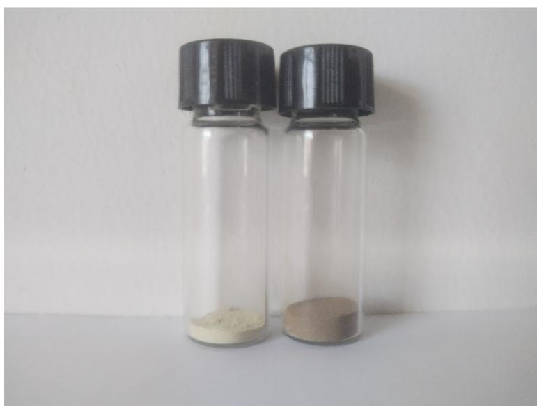
**Figure S2.** photographs of bulk and porous g-C<sub>3</sub>N<sub>4</sub> with same mass.
