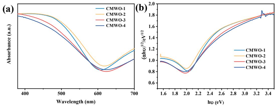
**Fig. S2.** (a) DRS spectra of CMWO-1, CMWO-2, CMWO-3 and CMWO-4 catalysts; (b) Tauc plots of CMWO-1, CMWO-2, CMWO-3 and CMWO-4 catalysts
