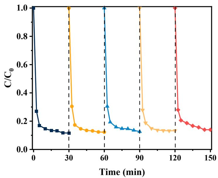
Fig. S1. Cyclic test for TC degradation by CMWO-3.
