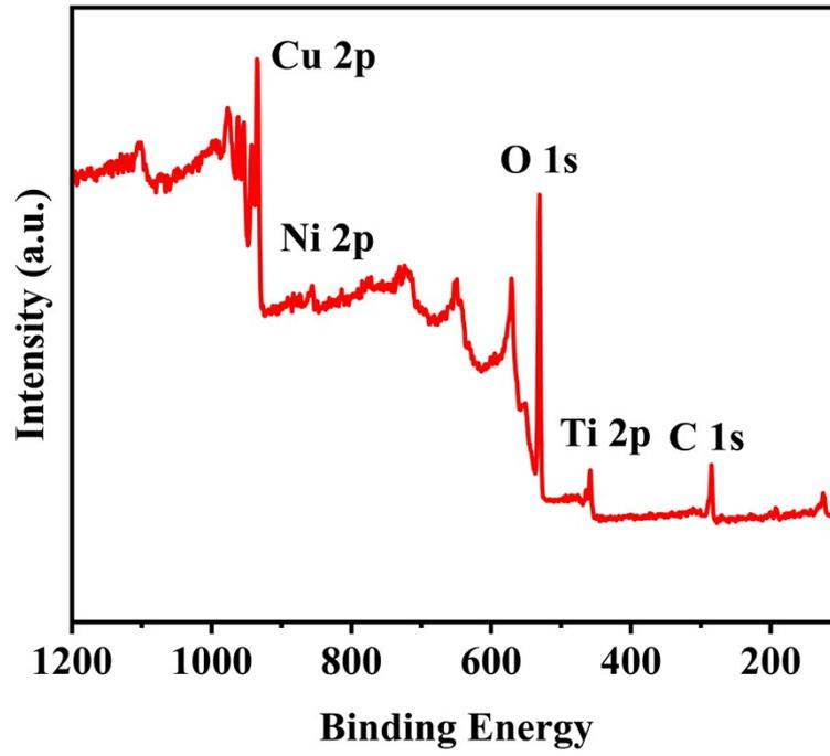
Fig. S4 Survey spectrum of  $\text{Cu}_{0.9}\text{Ni}_{0.1}/\text{Ti}_3\text{C}_2\text{T}_x$
