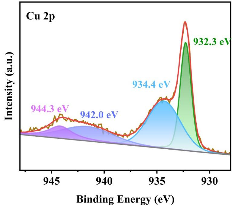
Fig. S5 Cu 2p XPS spectrum of  $\text{Cu}_{0.9}\text{Ni}_{0.1}$
