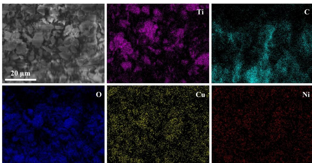
Fig. S2 The mapping of  $\text{Cu}_{0.9}\text{Ni}_{0.1}/\text{Ti}_3\text{C}_2\text{T}_x$
