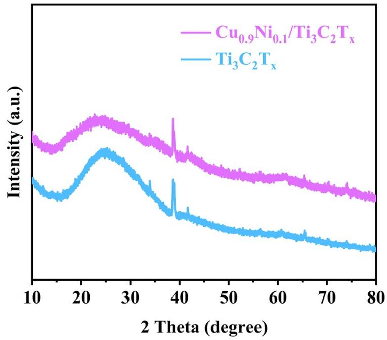
Fig. S3 XRD pattern of  $\text{Cu}_{0.9}\text{Ni}_{0.1}/\text{Ti}_3\text{C}_2\text{T}_x$  and  $\text{Ti}_3\text{C}_2\text{T}_x$
