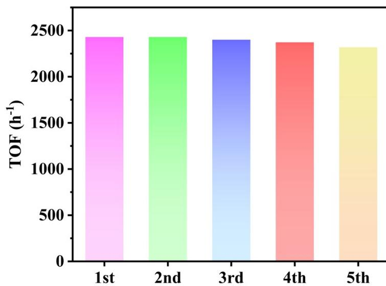
Fig. S9 TOF value of  $\text{Cu}_{0.9}\text{Co}_{0.1}/\text{Ti}_3\text{C}_2\text{T}_x$  for five consecutive catalytic cycles
