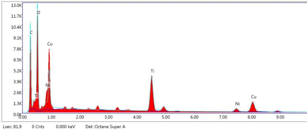
Fig. S1 EDAX Spectrum of  $\text{Cu}_{0.9}\text{Ni}_{0.1}/\text{Ti}_3\text{C}_2\text{T}_x$
