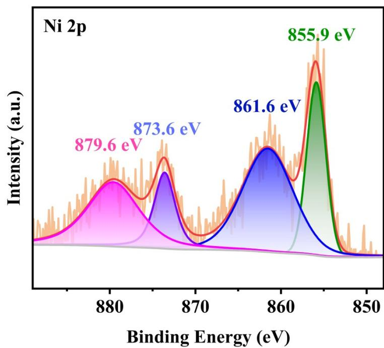
Fig. S6 Ni 2p XPS spectrum of Cu<sub>0.9</sub>Ni<sub>0.1</sub>
