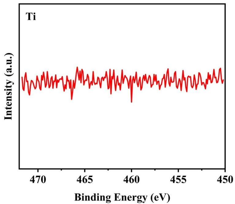
Fig. S7 Ti 2p XPS spectrum of Cu<sub>0.9</sub>Ni<sub>0.1</sub>.
