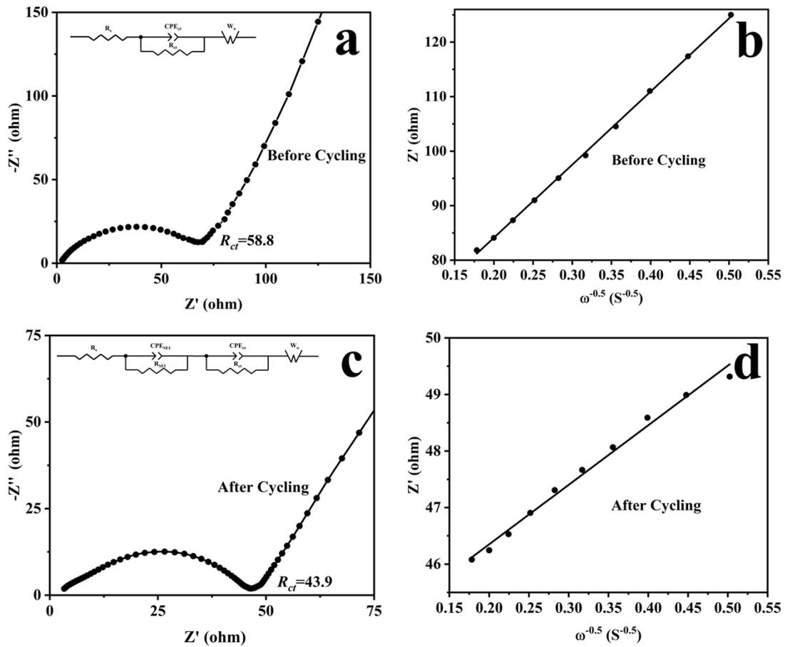
Fig. S8. (a) EIS curve before cycle and (b) linear fittings in low frequency region, (c) EIS curve after cycle and (d) linear fittings in low frequency region.
