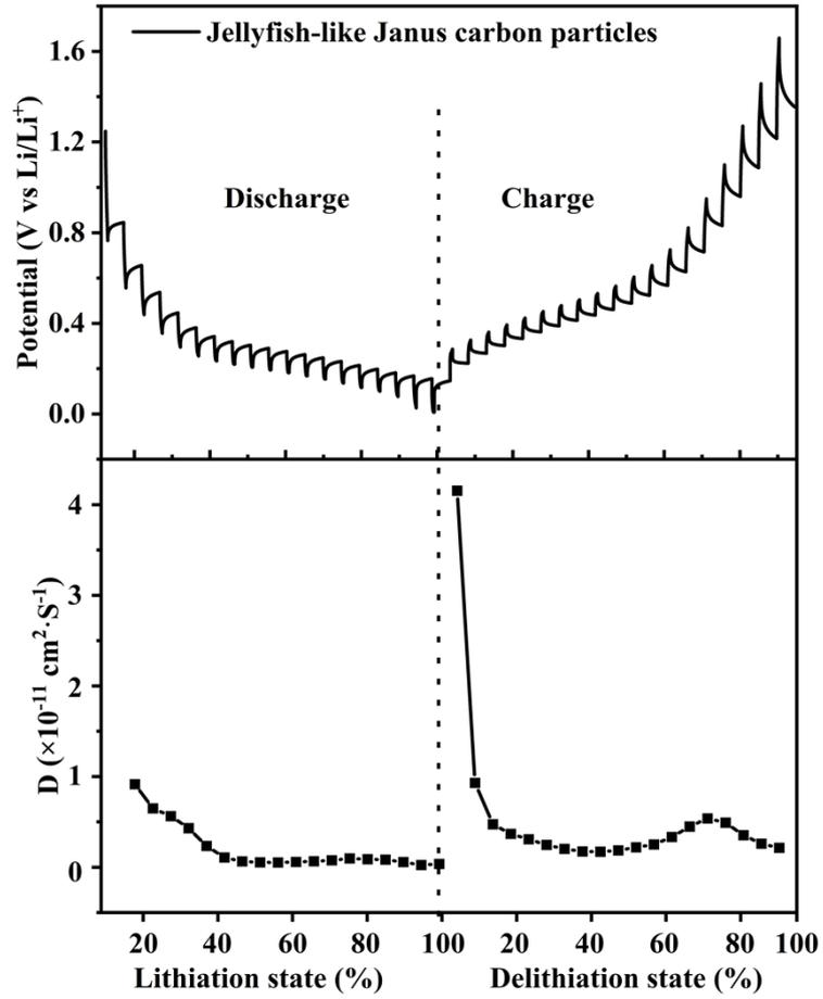
Fig. S9. GITT curves and the corresponding Li<sup>+</sup> diffusion coefficient  $D$  for jellyfish-like Janus carbon particles during charge-discharge process at  $0.1 \text{ A} \cdot \text{g}^{-1}$ .
