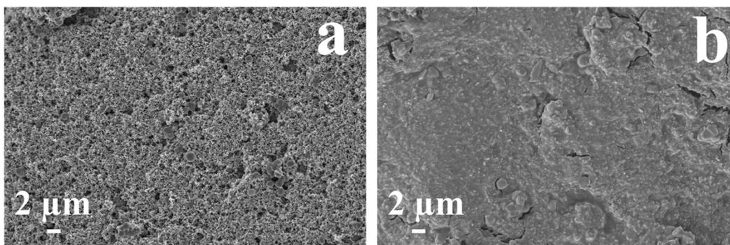
Fig. S7. (a) SEM images of jellyfish-like Janus carbon particles electrode before cycling, (b) jellyfish-like Janus carbon particles electrode after 100 cycles at 0.5  $A \cdot g^{-1}$ .
