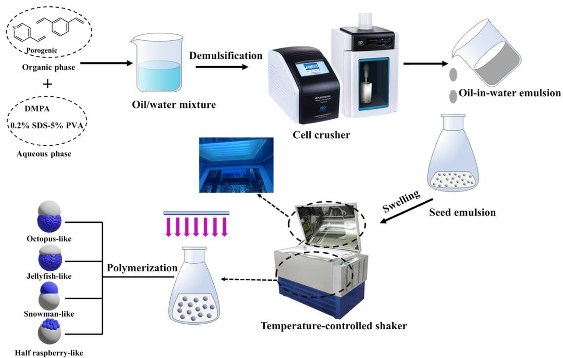
Fig. S2. Janus particle synthesis equipment and process flowchart.
