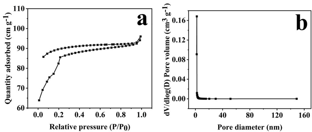
Fig. S6. (a) N<sub>2</sub> adsorption-desorption isotherms and (b) pore size distributions of jellyfish-like Janus carbon particles.
