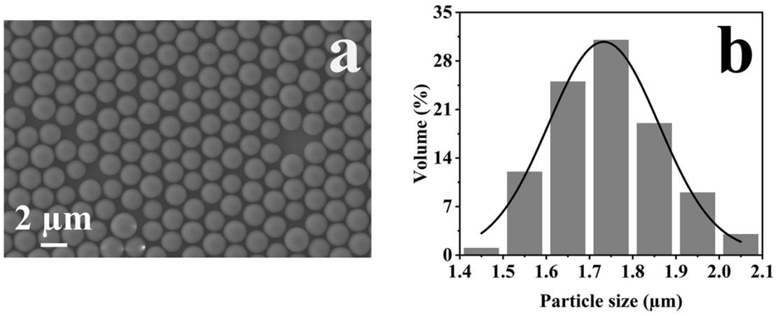
Fig. S1. (a) SEM image and (b) particle size distribution of poly(GMA) seed.
