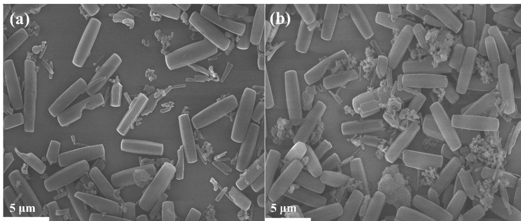
**Fig. S1** SEM images showing the physical mixture of SBA-15 and NU-1000.
