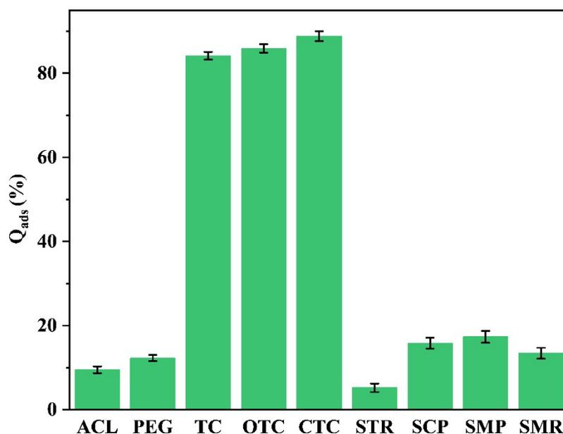
**Fig. S5** Removal efficiency ( $Q_{ads}$  (%)) of SBA-15@NU-1000 toward various antibiotics (5 mg of SBA-15@NU-1000, 40 mg/L of the investigated antibiotics).
