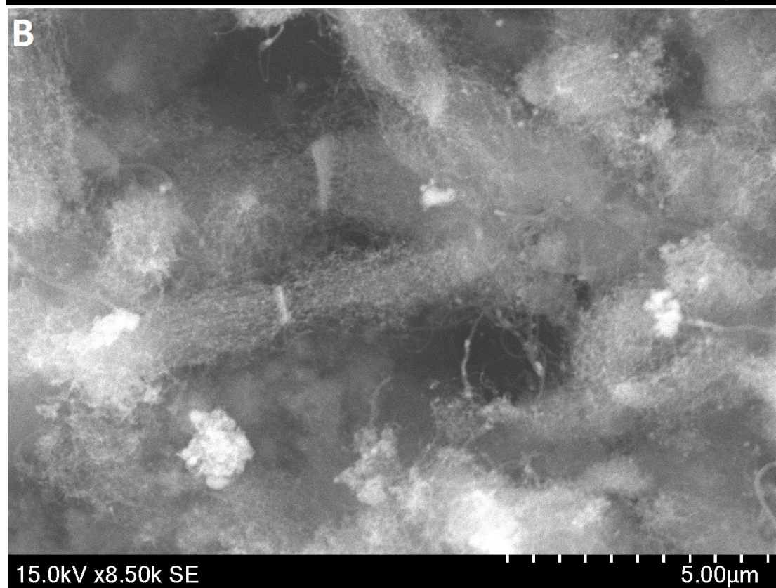
Figure S1: SEM micrographs acquired with backscattered (A) and secondary (B) electrons revealing the nucleation of large amounts of radial CNT structures.
