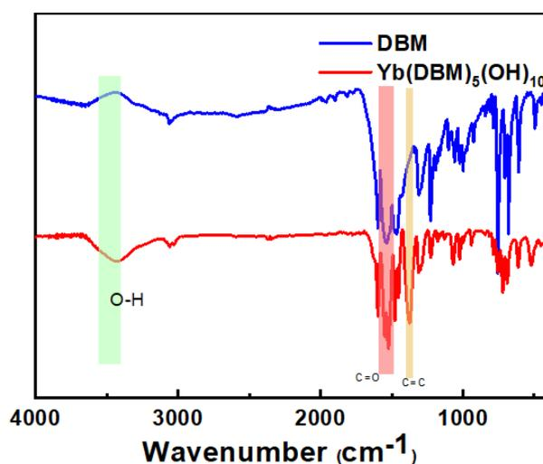
**Fig. S2** FTIR spectra of  $\text{Yb}_5(\text{DBM})_{10}(\text{OH})_5$  and DBM ligand.
