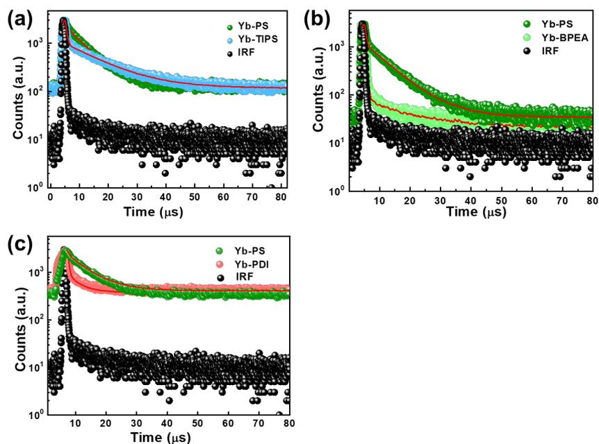
**Fig. S8** Time-resolved emission of Yb5(DBM)10(OH)5 in polystyrene (PS) film and in Yb-TIPS (1:1), Yb-BPEA (1:30), Yb-PDI (1:10) microcrystals, respectively ( $\lambda_{ex} = 980$  nm).
