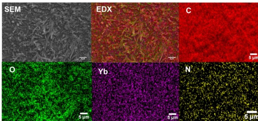
**Fig. S13** The SEM and EDX-mapping image of mixed TTA-UC microcrystal (Yb-BPEA/Yb-PDI (1:4 w/w)) and the elemental mapping of C, O, N and Yb. The chemical composition of the mixed TTA-UC microcrystal of (Yb-BPEA/Yb-PDI) was tested using Energy Dispersive X-ray Spectroscopy (EDX) as shown in Fig. S13 and S14. The EDX spectrum of the mixed microcrystal shows the uniformly distribution of all four elements at the current resolution, indicating no obviously segregation in the doped microcrystals.
