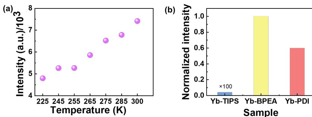
**Fig. S10** The peak emission intensity of the solid Yb complex-doped TIPS microcrystal (molar ratio = 1:1) at various temperatures excited at 980 nm from 223 to 300 K (a) and the relative peak intensity of Yb-TIPS, Yb-BPEA and Yb-PDI excited at same power density (b).
