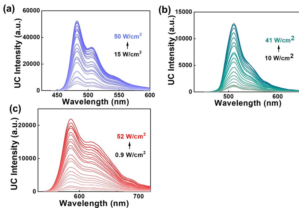
**Fig. S5** UC emission spectra of Yb-TIPS (6:1) (a), Yb-BPEA (9:1) (b), Yb-PDI (36:1) (c) with various excitation in DMF ( $\lambda_{\text{ex}} = 980$  nm).
