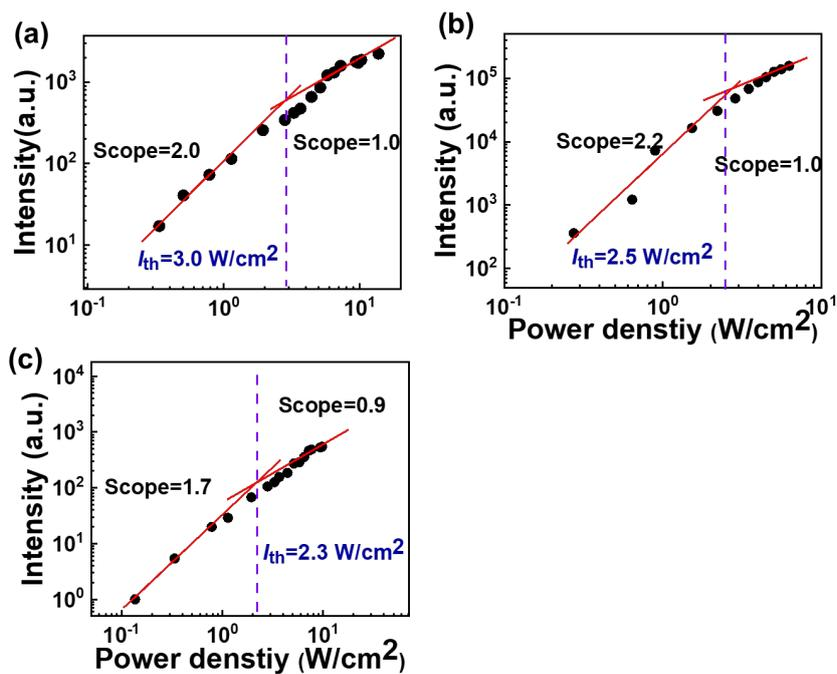
**Fig. S9** Dependence of the TTA-UC intensity on the incident power densities of microcrystals: (a) Yb-TIPS (1:1), (b) Yb-BPEA (1:30), (c) Yb-PDI (1:10) ( $\lambda_{\text{ex}} = 980 \text{ nm}$  with a CW laser diode).
