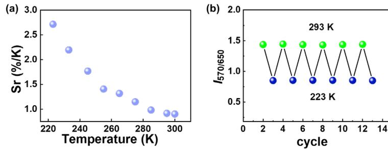
**Fig. S12** The relative thermal sensitivity (a) and the reversibility of ratiometric upconversion emission (b) of microcrystal Yb-BPEA/Yb-PDI (1:4 w/w) from 223 to 293 K ( $\lambda_{ex} = 980$  nm).
