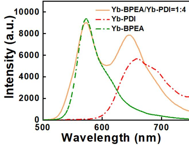
**Fig. S11** UC emission spectra of the mixed microcrystals (orange), Yb-BPEA (green, 1:30) and Yb-PDI (red, 1:10). The mixed microcrystal containing Yb-BPEA microcrystal (1:30) and Yb-PDI crystal (1:10). The mass ratio of Yb-BPEA /Yb-PDI is 1:4.
