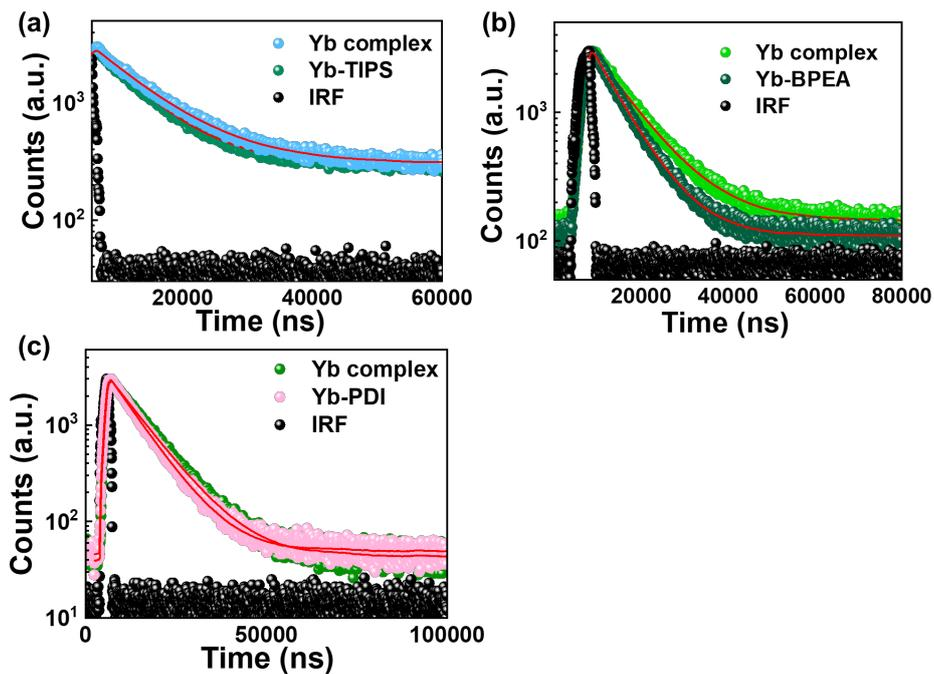
**Fig. S4** Time-resolved decay curves of photosensitizer  $\text{Yb}_5(\text{DBM})_{10}(\text{OH})_5$  and TTA-UC system of Yb-TIPS (6:1), Yb-BPEA (18:1), Yb-PDI (18:1) at 1010 nm in DMF ( $\lambda_{\text{ex}} = 980$  nm).
