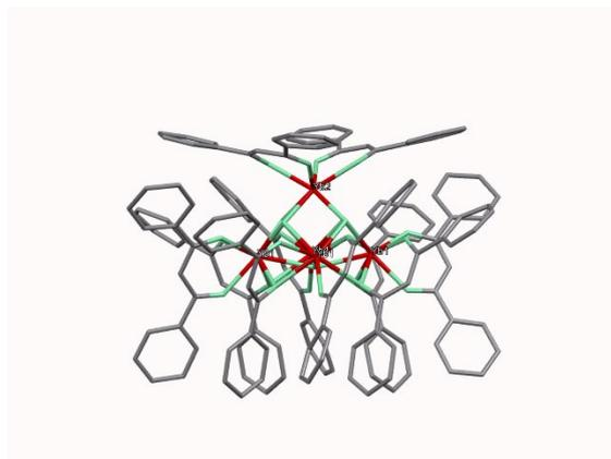
**Fig. S1** Single-crystal XRD structure of  $\text{Yb}_5(\text{DBM})_{10}(\text{OH})_5$  complex. Hydrogens have been omitted for clarity.
