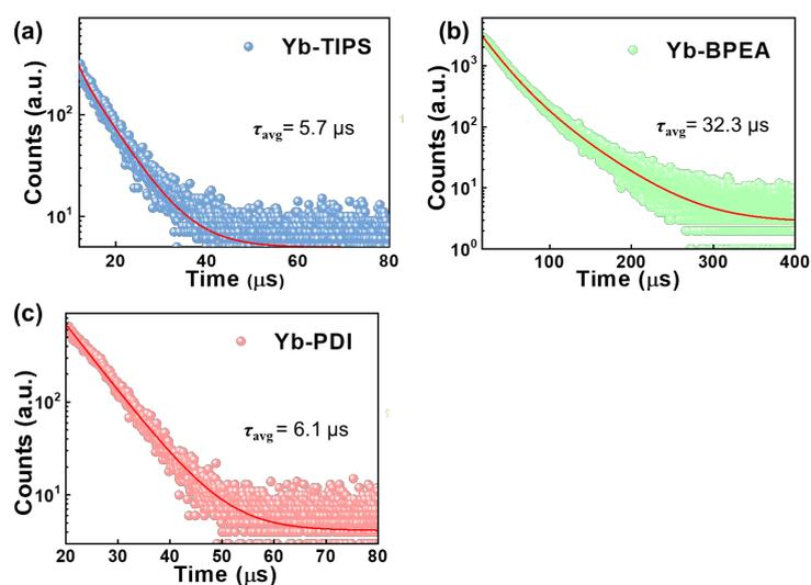
**Fig. S3** The delayed fluorescence decay and tail-fitting curves of solid microcrystals Yb-TIPS (1:1) at 500nm (a), Yb-BPEA (1:30) at 560 nm (b), Yb-PDI (1:10) at 650 nm (c) ( $\lambda_{\text{ex}} = 980$  nm with a CW laser diode).
