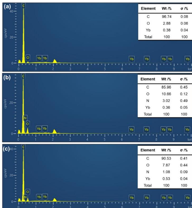
**Fig. S14** The EDX spectra of Yb-BPEA (1:30) (a), Yb-PDI (1:10) (b) and mixed TTA-UC microcrystal (Yb-BPEA/Yb-PDI (1:4 w/w)) (c). The insert table is the corresponding elements content.
