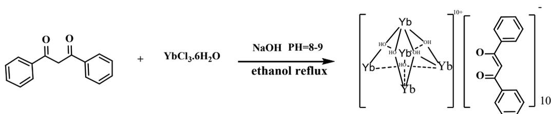
**Scheme S1** Synthesis route of  $\text{Yb}_5(\text{DBM})_{10}(\text{OH})_5$
