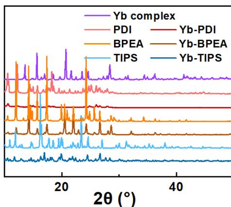
**Fig. S7** The PXRD of PDI, Yb-PDI (1:10), BPEA, Yb-BPEA (1:30), TIPS and Yb-TIPS (1:1) microcrystals.
