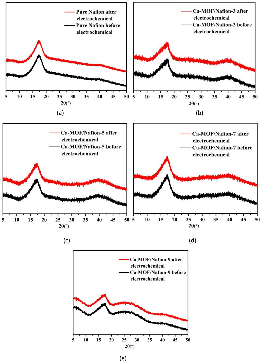
Fig. S1 (a) The PXRD patterns of pure nafion membrane before and after the electrochemical experiment; (b, c, d and e) The PXRD patterns of Ca-MOF/Nafion composite membranes before and after the electrochemical experiment.
