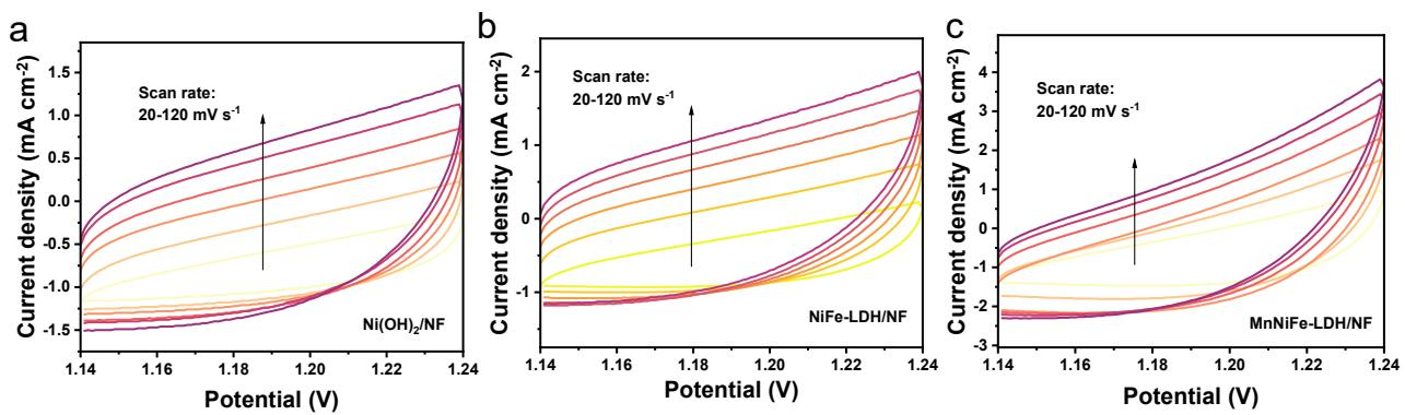
**Figure S6.** Cyclic voltammetry (CV) curves of (a)  $\text{Ni(OH)}_2/\text{NF}$ , (b)  $\text{NiFe-LDH}/\text{NF}$  and (c)  $\text{MnNiFe-LDH}/\text{NF}$  electrodes in the non-faraday double layer region at scan rates of 20-120  $\text{mV s}^{-1}$  in 1M KOH.
