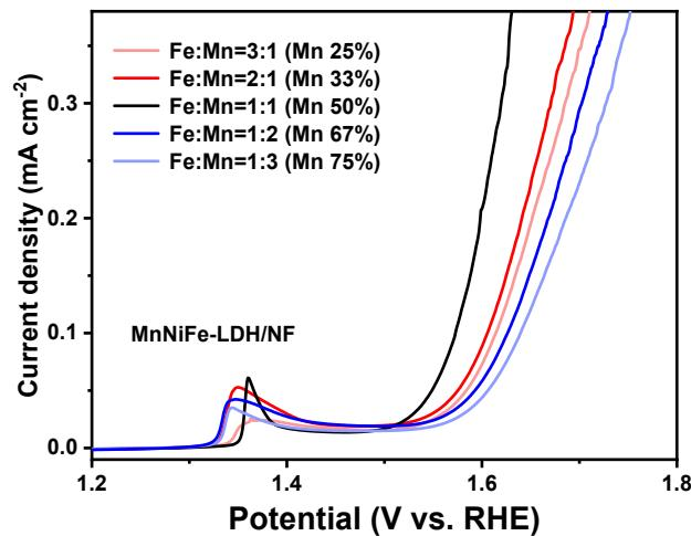
**Figure S4.** OER activity of MnNiFe-LDH/NF electrocatalysts different Mn doping concentration with corresponding doping concentration at 30 °C in 1M KOH.
