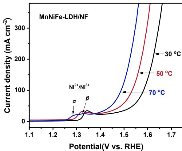
**Figure S5.** OER activity of MnNiFe-LDH electrocatalyst on NF at 30-70 °C with 85% iR compensation.
