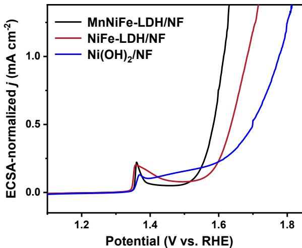
**Figure S7.** ECSA-normalized LSV curves.
