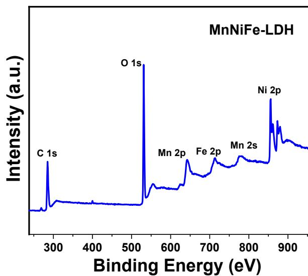
**Figure S3.** Full high-resolution XPS spectrum of Mn-doped NiFe-LDH.
