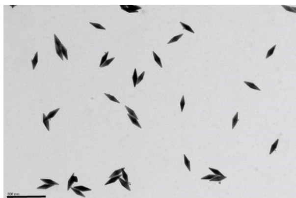
Fig. S2. TEM image of Au NBP (scale bar: 500 nm).
