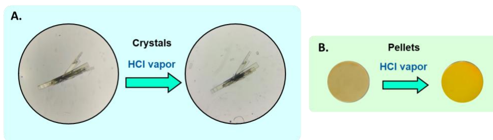
Fig. S9 (A) Microscopic images of rod-shaped crystals and (B) Digital images of the pellets before and after keeping in aqueous HCl environment.
