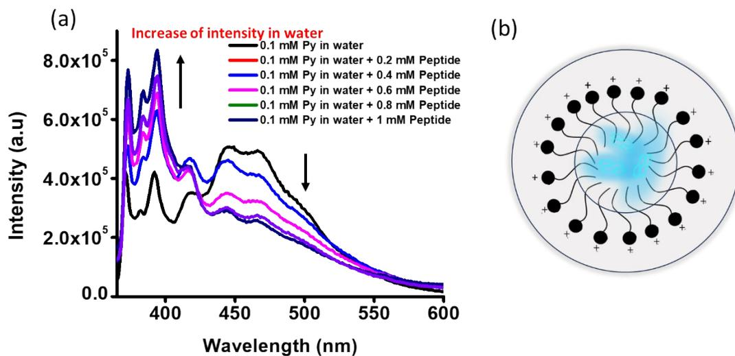
**Fig.S6:** (a) The change in the emission spectra of the pyrene in water with the gradual addition of P. Showing the increase in intensity of Pyrene; (b) probable aggregation of P and the presence of the pyrene moieties into the hydrophobic pocket of the aggregate.
