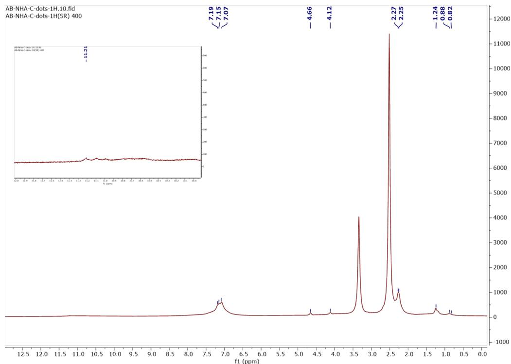
Fig. S8: The  $^1\text{H-NMR}$  of the C-dots ( $\text{DMSO-D}_6$ )
