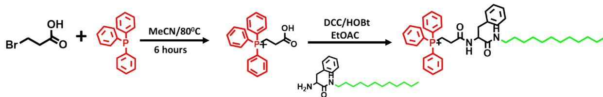
**Fig.S1:** The schematic presentation of the synthetic route of the P.
