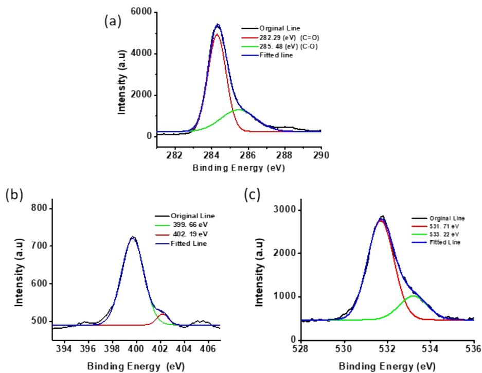
**Fig.S3:** The XPS spectra of the C-dots (a) C1S (b) N1S (c) O1S.
