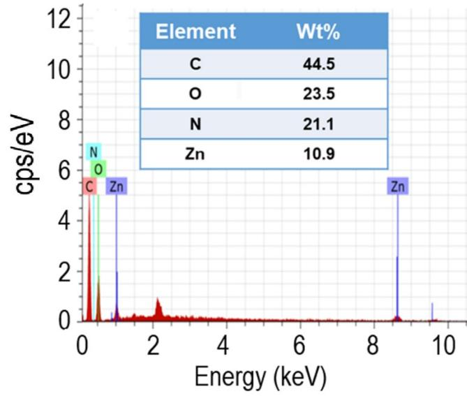
Fig. S1. EDX based elemental composition of Bio-MOF-1
