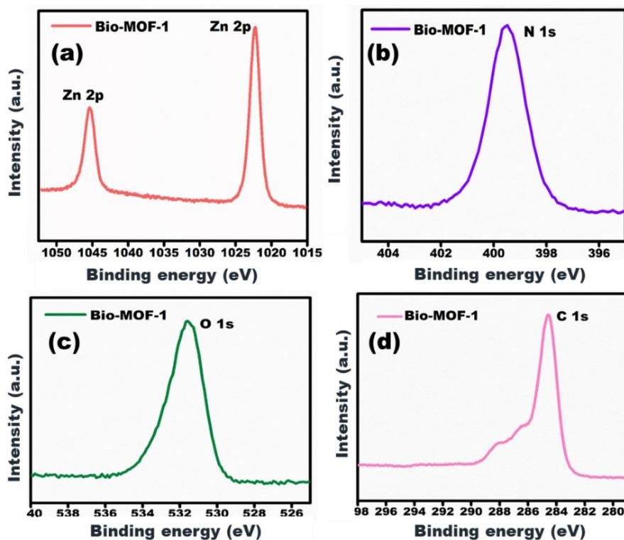
Fig. S5. XPS spectra of Bio-MOF-1. (a): Zn2p; (b): N1s; (c): O1s; (d): C1s
