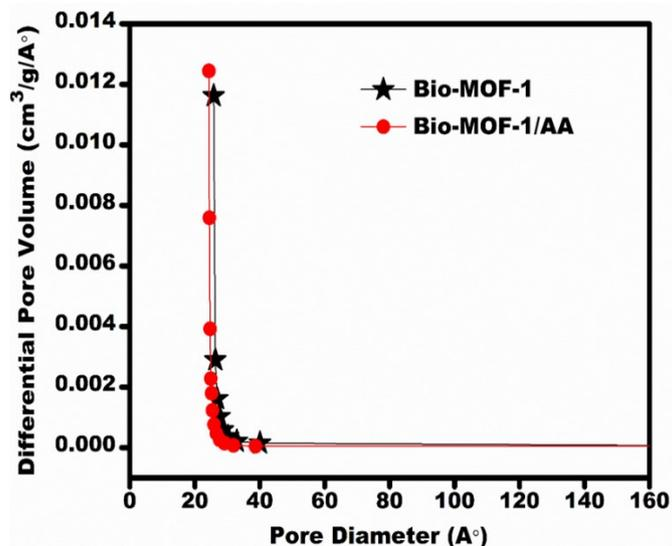
Fig. S3. BJH adsorption pore-size distributions for Bio-MOF-1 and Bio-MOF-1/AA.
