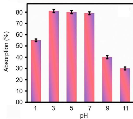
**Fig. S11.** Dependence of pH on the adsorption of Cr(VI) ( $1 \mu\text{g/mL}$ ) with Bio-MOF-1/AA complex ( $1 \text{ mg/mL}$ ), *Time of incubation = 5 min*
