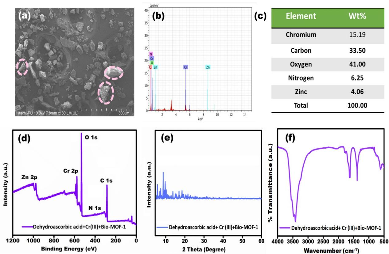
**Fig. S9.** Characterization of reaction product formed between Bio-MOF-1/AA and Cr(VI), i.e. DHA+Cr(III) and Bio-MOF-1. (a): SEM image, *encircled structures refer to DHA+Cr(III) aggregates*; (b-c): EDX analysis and elemental composition; (d): XPS spectrum; (e): XRD patterns; (f): FTIR spectrum
