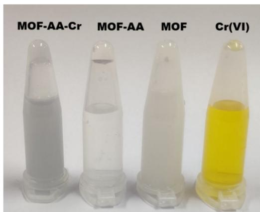
**Fig. S8.** Visual development of color as Cr(VI) is added in to Bio-MOF-1/AA solution.
