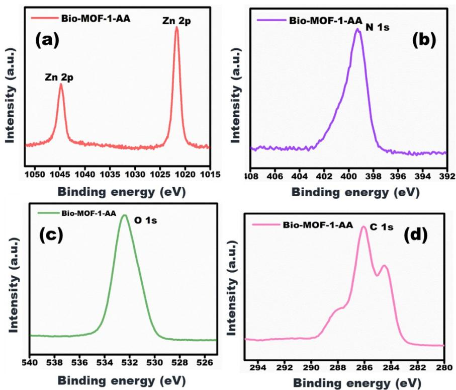
Fig. S6. XPS spectra of Bio-MOF-1/AA (a): Zn2p; (b): N1s; (c): O1s; (d): C1s
