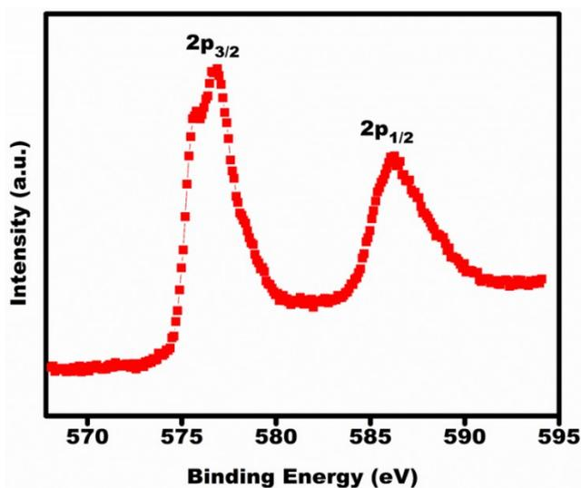
**Fig. S10.** High-resolution XPS spectra ( $2p_{3/2}$  and  $2p_{1/2}$  regions) of reaction product formed between Bio-MOF-1/AA and Cr(VI)
