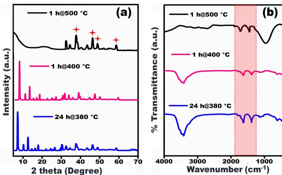
Fig. S4. Structural characterizations of thermally annealed Bio-MOF-1/AA samples at 380, 400 and 500 °C. (a): XRD patterns; the asterisks represent the peaks for ZnO; (b): FTIR spectra show retention of all the framework IR modes.
